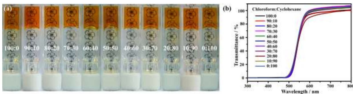
Fig. S1 (a) Photographs of 4 mg/mL BNB-t8 gel in various ratios of TCM/CYH at room temperature. (b) Transmittance spectra of BNB-t8 gel (4 mg/mL) in various ratios of TCM/CYH.
