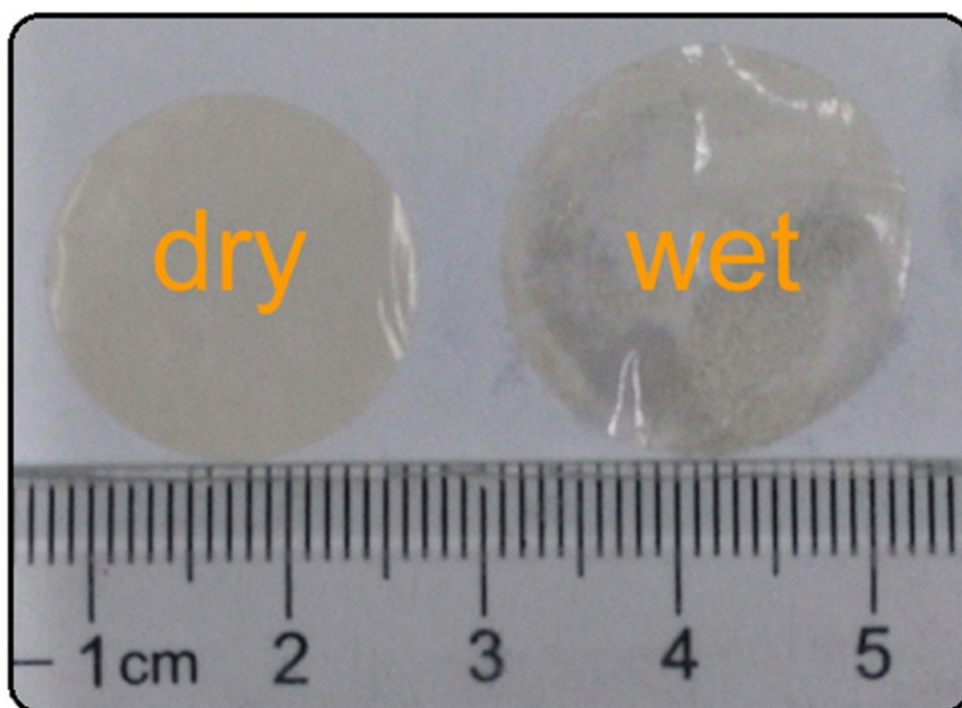
Fig. S2 The photo image of the dry and wet single ion conducting electrolyte membrane.
