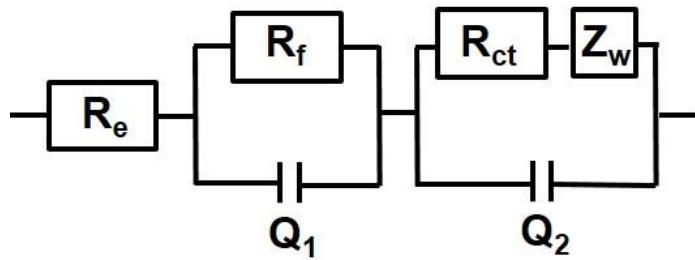
**Fig. S9** Randle-type equivalent circuit model used for EIS fitting.
