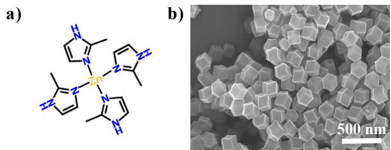
**Figure S1.** a) Molecular structure and b) SEM image ZIF-8 particles.
