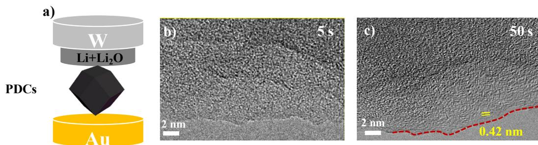
**Figure S7.** a) Schematic illustration of the *in situ* TEM experimental electrochemical setup. b, c) TEM images of the lithiated PDCs at different lithiation process: 5 and 50 seconds, respectively.
