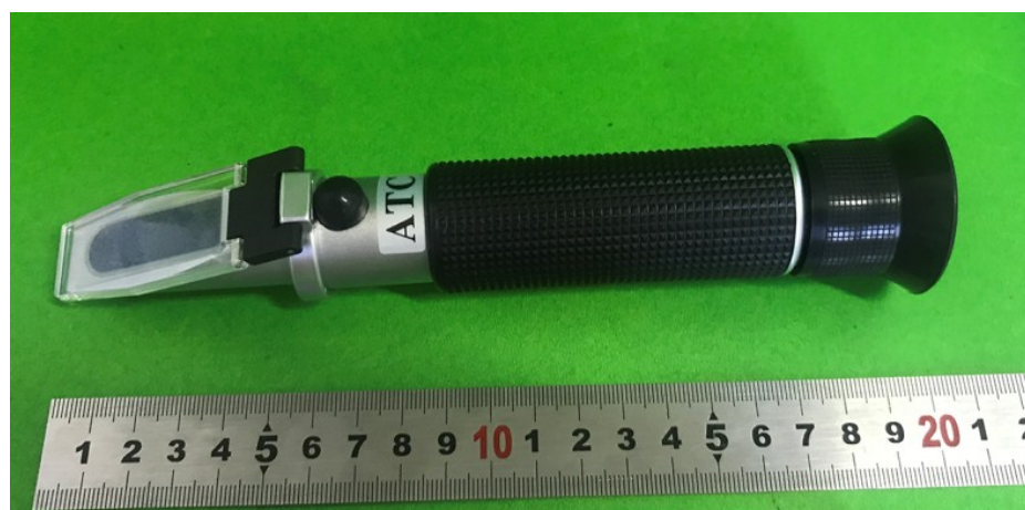
Fig. S14. A refractometer used to test the concentration of the dissolved salt in water.
