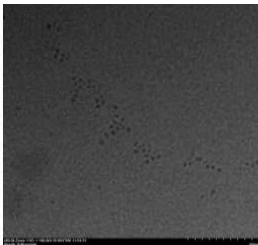
Figure S15. TEM image of ultra-small Pd nanoparticles as Prasad reported.
