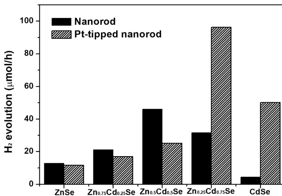
**Fig. S4** Photocatalytic hydrogen evolution rates of the  $Zn_{1-x}Cd_xSe$  and Pt-tipped nanorods ( $x = 0, 0.25, 0.5, 0.75, \text{ and } 1$ ) in a  $0.25 \text{ M Na}_2\text{S}/0.35 \text{ M Na}_2\text{SO}_3$  aqueous solution by the light irradiation without using a UV filter.
