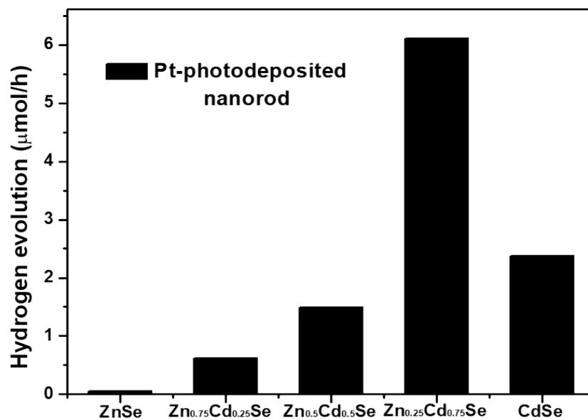
**Fig. S9** Photocatalytic hydrogen evolution rates of the Pt-photodeposited Zn<sub>1-x</sub>Cd<sub>x</sub>Se nanorods (x = 0, 0.25, 0.5, 0.75, and 1) in a 0.25 M Na<sub>2</sub>S/0.35 M Na<sub>2</sub>SO<sub>3</sub> aqueous solution under visible light ( $\lambda > 400$  nm) irradiation.
