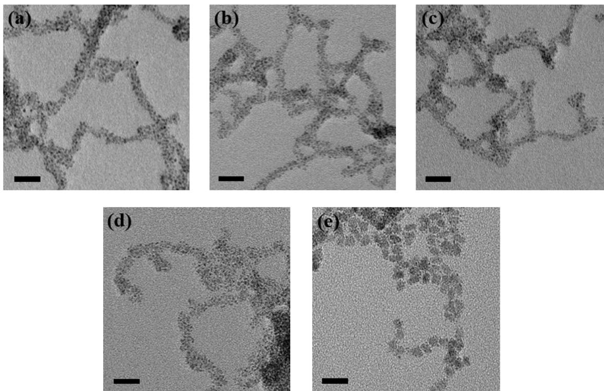
**Fig. S8** TEM images of Pt-photodeposited (a) ZnSe, (b)  $\text{Zn}_{0.75}\text{Cd}_{0.25}\text{Se}$ , (c)  $\text{Zn}_{0.5}\text{Cd}_{0.5}\text{Se}$ , (d)  $\text{Zn}_{0.25}\text{Cd}_{0.75}\text{Se}$ , and (e) CdSe nanorods. The bars represent 20 nm.
