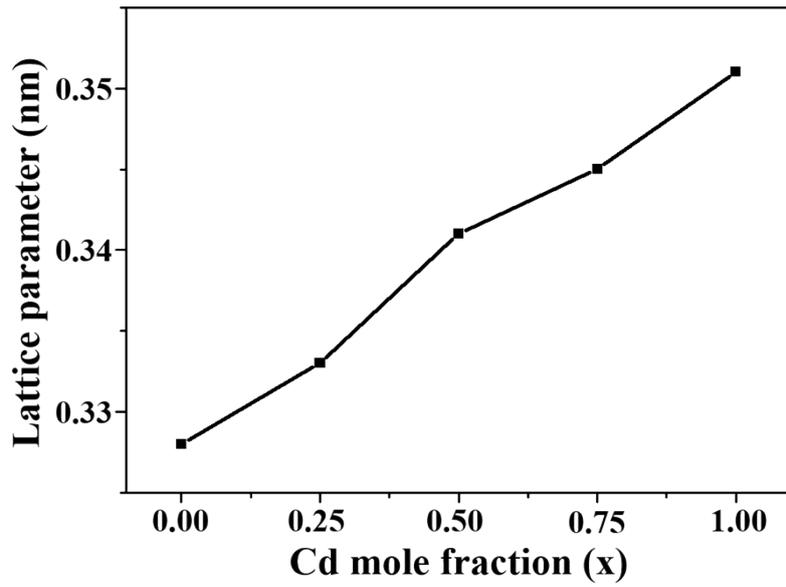
**Fig. S2** The lattice parameter values of the  $\text{Zn}_{1-x}\text{Cd}_x\text{Se}$  nanorods as a function of the Cd mole fraction (x).
