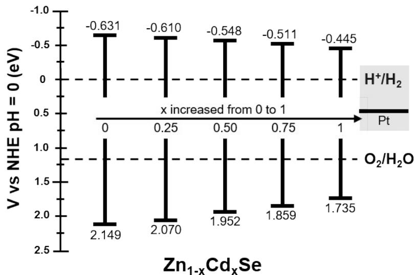
**Fig. S6** Valence and conduction band edge potentials of the  $\text{Zn}_{1-x}\text{Cd}_x\text{Se}$  nanorods ( $x = 0, 0.25, 0.5, 0.75,$  and  $1$ ).
