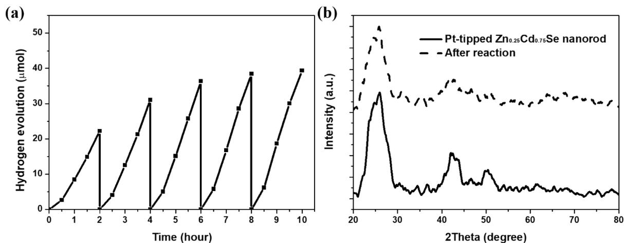
**Fig. S7** (a) The amount of hydrogen evolution using Pt-tipped  $\text{Zn}_{0.25}\text{Cd}_{0.75}\text{Se}$  nanorods under the identical reaction conditions.  $\text{N}_2$  purging was performed at the beginning of every 2-h reaction. (b) XRD spectra of the Pt-tipped  $\text{Zn}_{0.25}\text{Cd}_{0.75}\text{Se}$  nanorods before and after the repetitive hydrogen evolution reactions.
