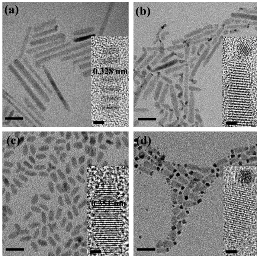
**Fig. S1** TEM images of (a) ZnSe, (b) Pt-tipped ZnSe nanorods, (c) CdSe, and (d) Pt-tipped CdSe nanorods. The bars represent 20 nm and (inset) 2 nm.
