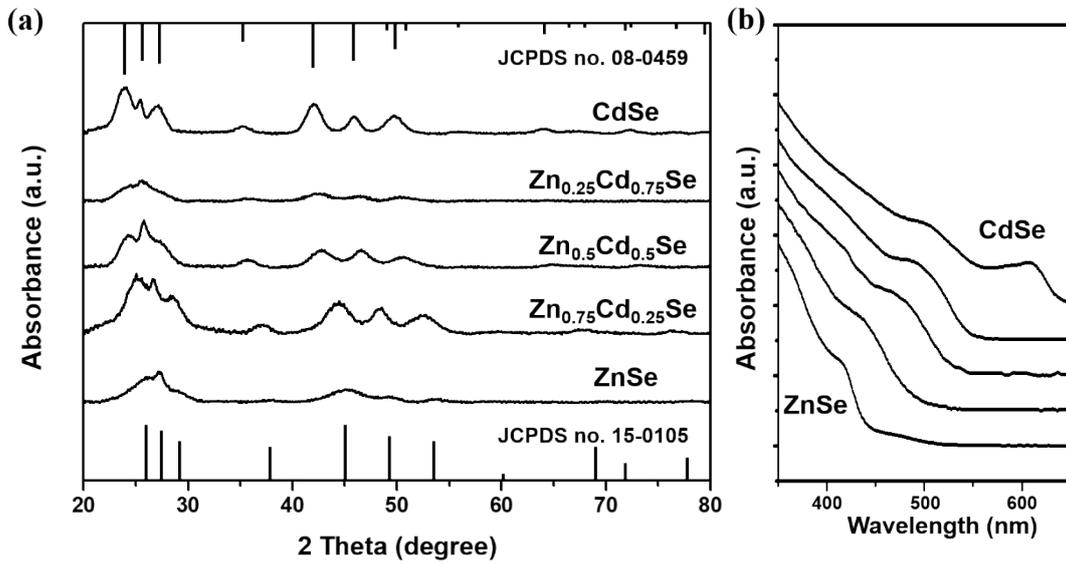
**Fig. S3** (a) XRD patterns and (b) UV-visible absorption spectra of the  $\text{Zn}_{1-x}\text{Cd}_x\text{Se}$  nanorods (x = 0, 0.25, 0.5, 0.75, and 1).
