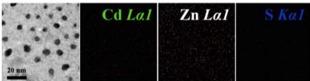
Fig. S2 TEM-EDS elemental mapping taken on Au-Cd 1-x Zn x S c .
