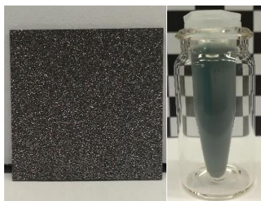
Fig. S1: B-doped starting material (left; 1.5 x 1.5 cm) and milled B-doped ND particles in aqueous dispersion (right; 1.5 ml with 1.0 wt%).
