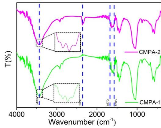
Figure S1 FTIR spectrum of CMPs aerogels.
