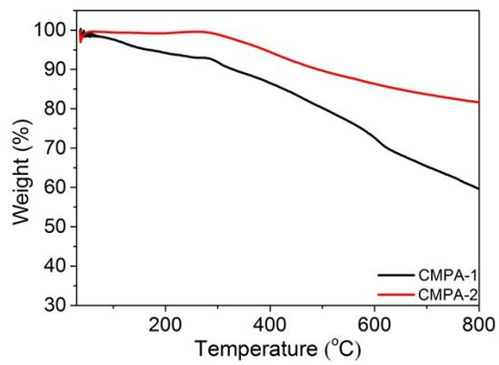
Figure S2 TGA curves of CMPs aerogels.
