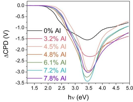
**Figure S6** SPS spectra of nano-Al:SrTiO<sub>3</sub> with variable Al<sup>3+</sup> concentration.
