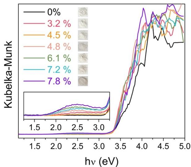
**Figure S5** UV-Vis diffuse reflectance spectra of nano-Al:SrTiO<sub>3</sub> with variable Al<sup>3+</sup> concentration with inset of their photos. The region from 1.25 eV to 3.25 eV is magnified to illustrate the weak absorption feature starting from 1.7 eV.
