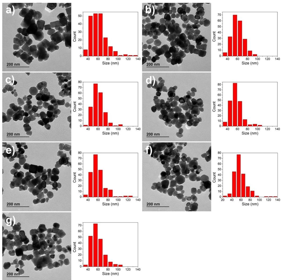
**Figure S2** TEM images and size histograms of (a) nano-SrTiO<sub>3</sub> and nano-Al:SrTiO<sub>3</sub> with (b) 10%, (c) 20%, (d) 30%, (e) 50%, (f) 70% Al, (g) 90 atom% Al precursor added during the hydrothermal synthesis.
