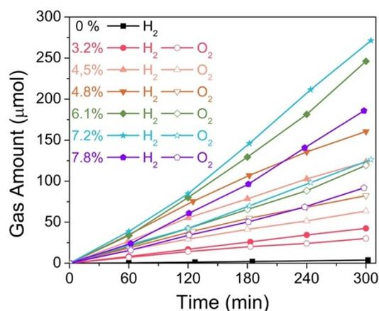
**Figure S4** Irradiation results of 1wt% Rh, 1.5 wt% Cr, Rh<sub>2-y</sub>Cr<sub>y</sub>O<sub>3</sub> loaded nano-Al:SrTiO<sub>3</sub> with different amount of Al in pure water under full spectrum of Xe lamp irradiation (240 mW/cm<sup>2</sup> by UV detector). Dots show H<sub>2</sub> amount while circles show O<sub>2</sub> amounts.
