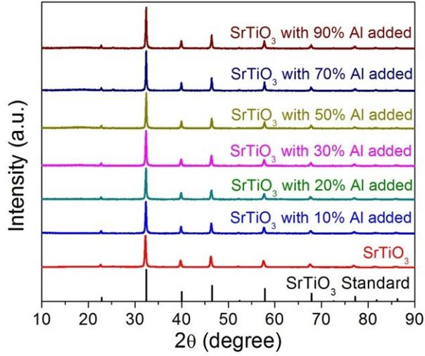
**Figure S1** XRD patterns of SrTiO<sub>3</sub> and Al:SrTiO<sub>3</sub> with different Al dopant amount obtained from hydrothermal synthesis with reference pattern for SrTiO<sub>3</sub> (JPDF #35-0734).
