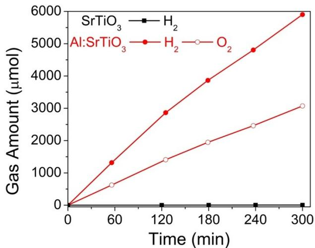
**Figure S7** H<sub>2</sub>/O<sub>2</sub> evolution from 0.1 wt% Rh, 0.1 wt% Cr, Rh<sub>2-y</sub>Cr<sub>y</sub>O<sub>3</sub> loaded ss-SrTiO<sub>3</sub> and micro-Al:SrTiO<sub>3</sub> in pure water under full spectrum Xe irradiation (320 mW/cm<sup>2</sup> by UV detector).
