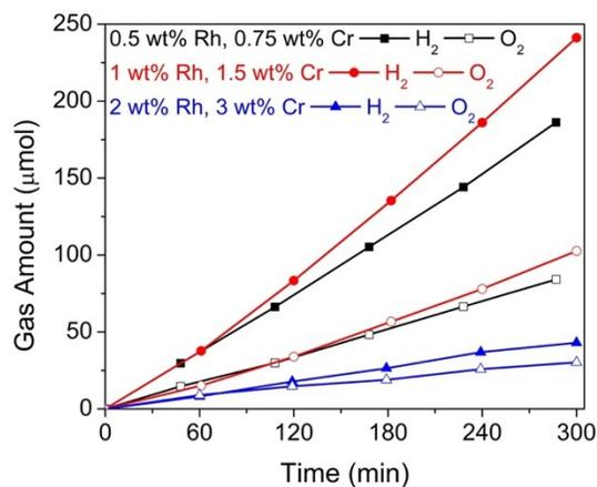
**Figure S3** Irradiation results of 7.2% nano-Al:SrTiO<sub>3</sub> with variable amounts of Rh<sub>2-y</sub>Cr<sub>y</sub>O<sub>3</sub> co-catalyst in pure water under full spectrum of Xe lamp irradiation (240 mW/cm<sup>2</sup> by UV detector).
