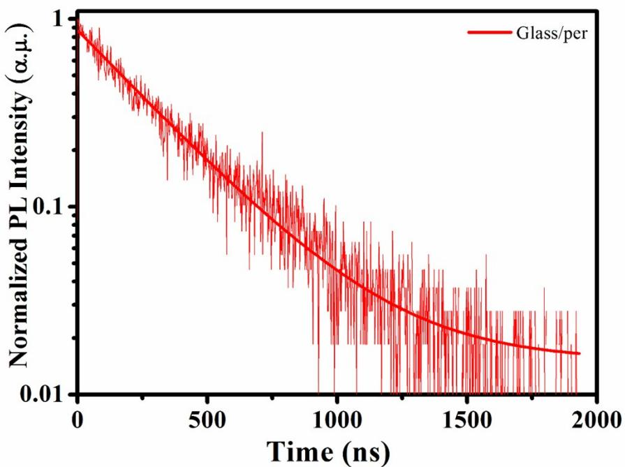
Figure S9. PL decay time spectrum of glass/perovskite.
