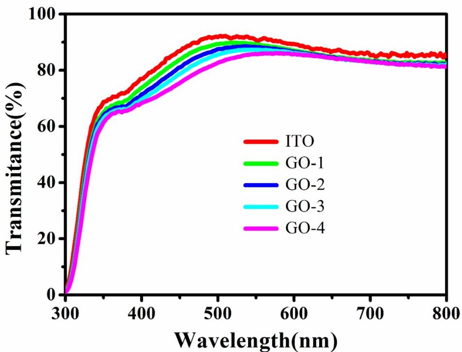
Figure S1. Transmittance spectra of ITO and substrates with GO-n films.
