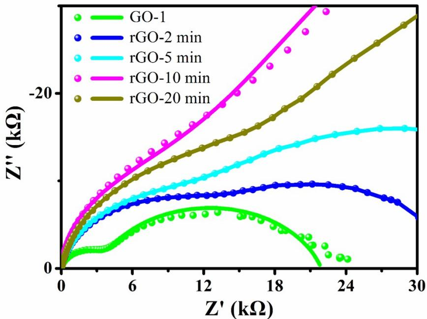
Figure S10. Enlarge figure of EIS Nyquist plots obtained under dark condition at  $-0.7$  V bias voltages of devices with different HTLs.
