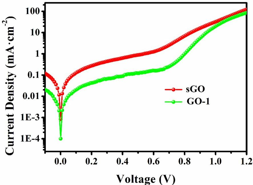
Figure S3. Dark  $J$ – $V$  curves of devices based on GO–1 and sGO HTLs.
