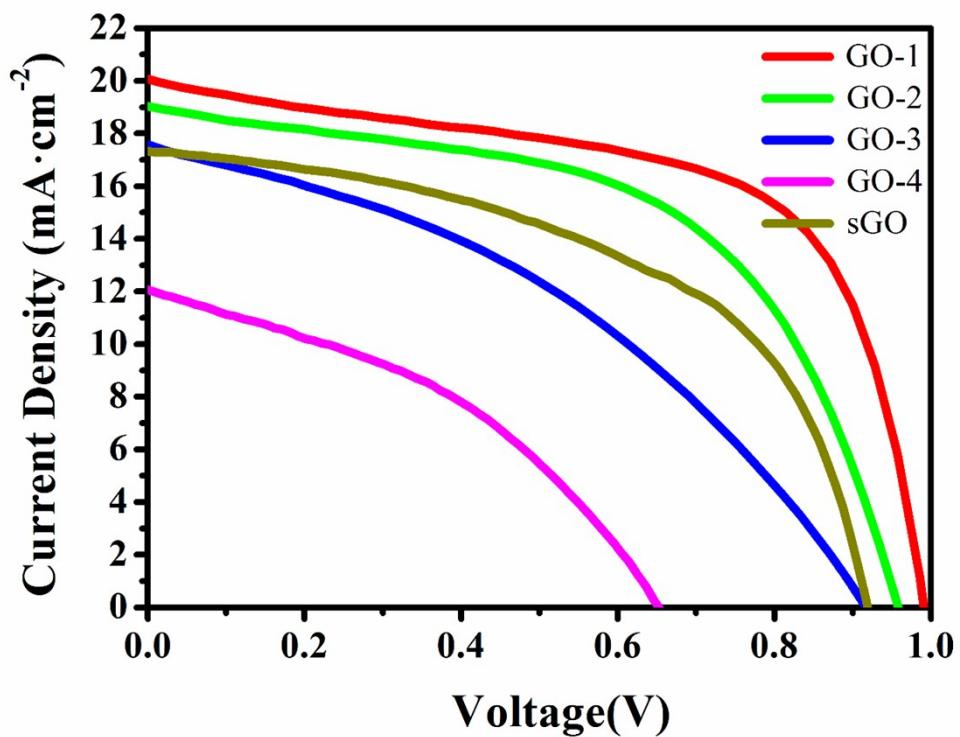
Figure S2.  $J-V$  curves of devices based on GO-n and sGO HTLs.
