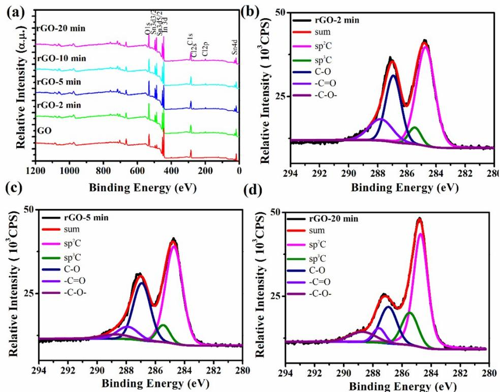
Figure S4. (a) Wide survey XPS spectra, (b–d) Deconvolution of C1s XPS spectra of rGO films on ITO with different reduction time.
