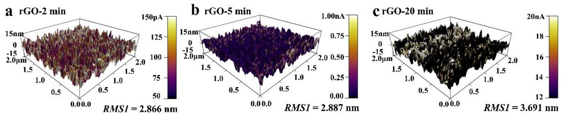
Figure S5. The 3D–AFM height images with current mapping images (color represent) of GO or rGO on ITO under the bias of 4 V. The scale bar represents the current detected by the contacted probe. (a. rGO–2 min; b. rGO–5 min; c. rGO–20 min)
