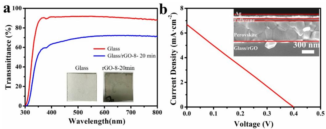
Figure S13. (a) Transmittance spectra of glass and glass/rGO–8–20 min. (Inset: images of glass and glass/rGO–8–20 min (glass/rGO–8–20 min means rGO films obtained by processing GO–8 films prepared by LbL method with 8 cycles together with reduction time of 20 min as shown in experimental section.)) (b) The  $J$ – $V$  curve of the device based on rGO electrode. (Inset: the cross–sectional SEM image of the device.)
