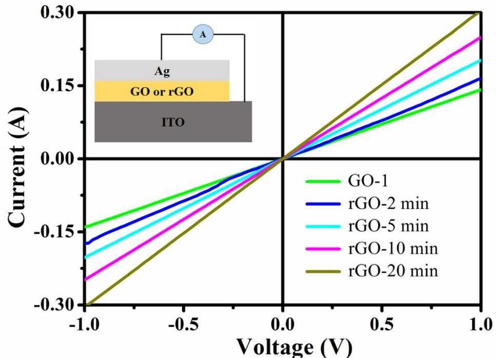
Figure S6. Current–voltage curves, obtained by linear–sweep voltammetry, of GO– and r–GO films.
