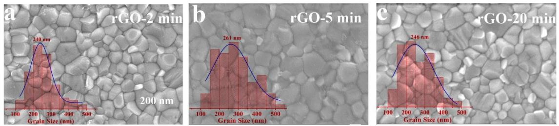
Figure S7. SEM images of perovskites on rGO films. (Inset: Statistical distributions and their Gaussian fitting (solid lines) of the perovskite grain sizes determined from the SEM images. a. rGO-2 min; b. rGO-5 min; c. rGO-20 min)
