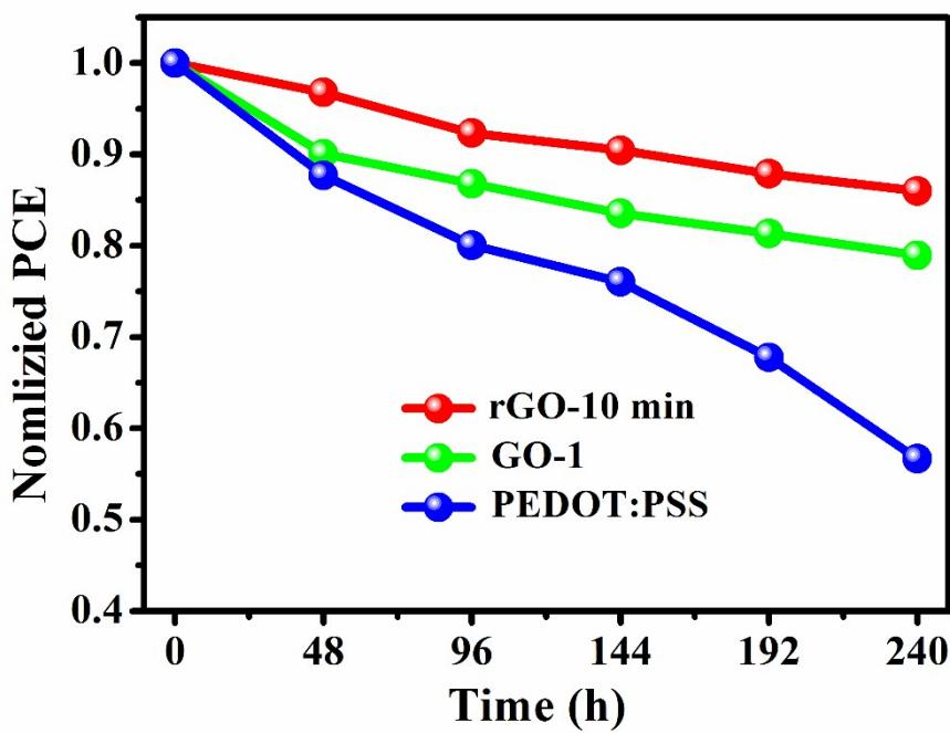
Figure S12. Evolution in normalized PCE values of devices based on PEDOT:PSS, GO-1 and rGO-10 min without encapsulation and stored in ambient condition with 40%  $\pm$ 5% humidity.
