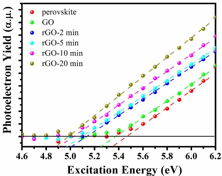
Figure S11. Ultraviolet photoelectron emission spectra of perovskite, GO and rGO films. The black line represents a regression analysis of the measured data.
