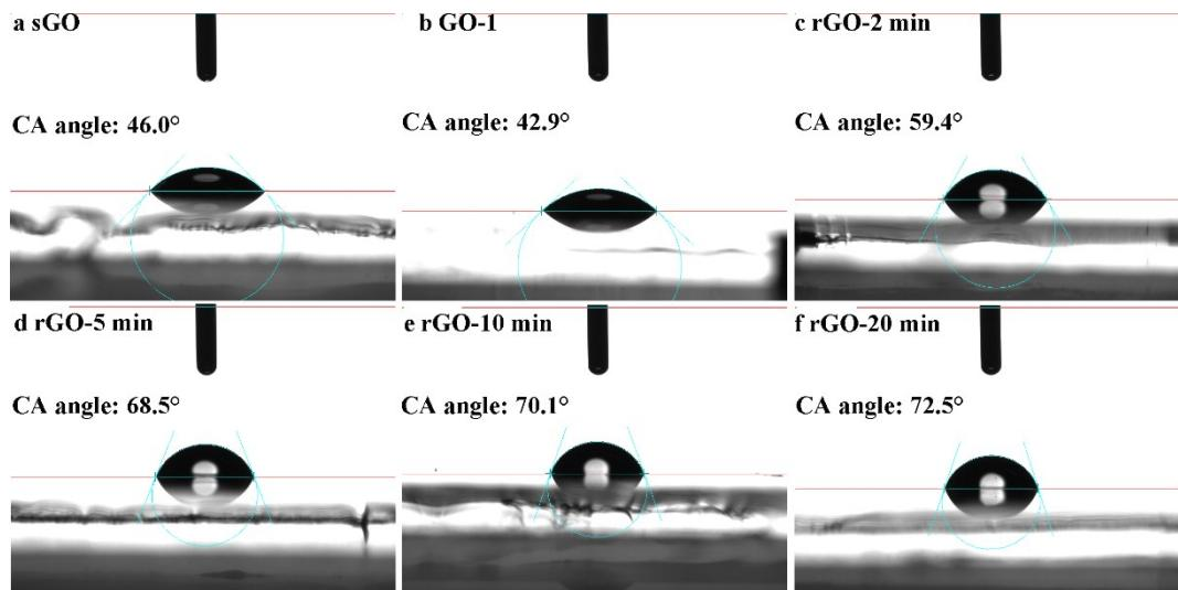
Figure S8. The contact angle images of water on different HTLs. (a. sGO; b. GO-1; c. rGO-2 min; d. rGO-5 min; e. rGO-10 min; f. rGO-20 min.)
