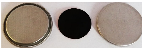
Figure S1 Photograph of the assembled CR2016 coin-type cells
