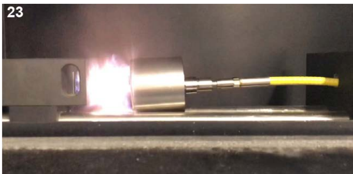
Figure S57 Moment of detonation of the copper(II) perchlorate complex 23 .
