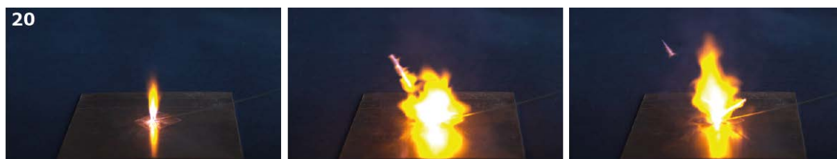
Figure S45 Moment of detonation of complex 19 during the hot plate test.
