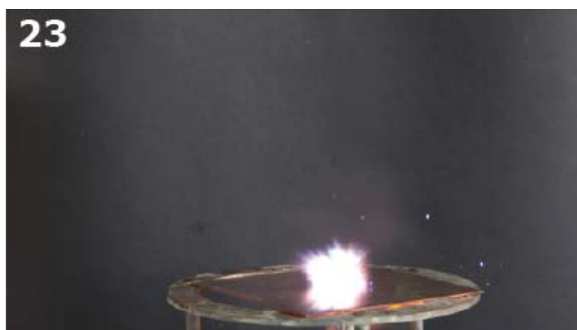
Figure S48 Behavior of complex 23 during the hot needle and hot plate tests, partly shown as a sequence.
