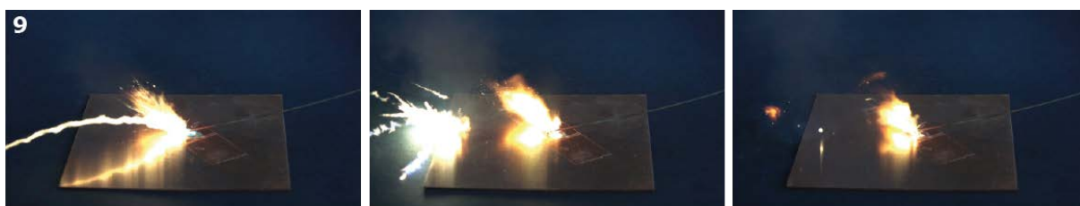
Figure S39 Hot plate test of complex 7 shown as a sequence.
