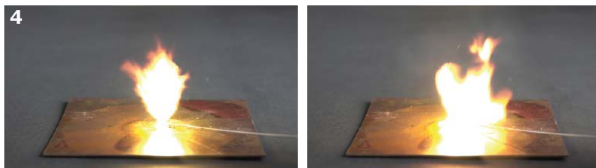
Figure S34 Hot needle test of coordination compound 4 shown as a sequence.
