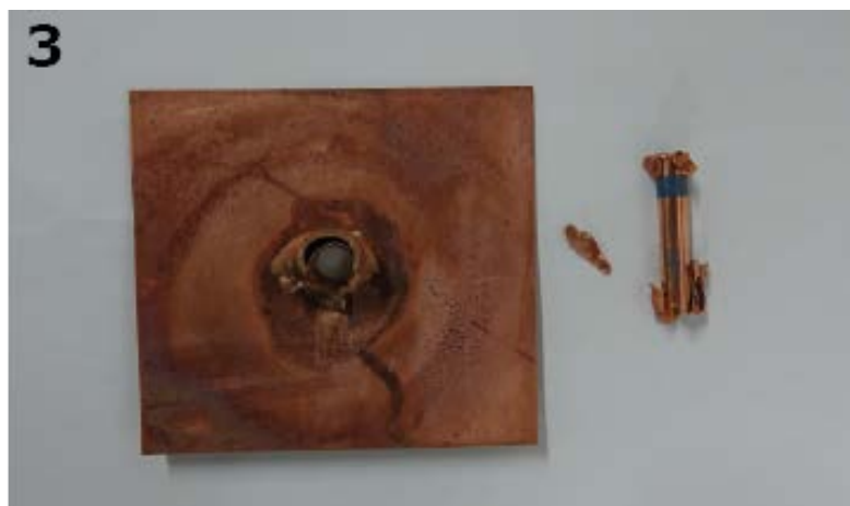
Figure S49 Positive PETN initiation test of 2-amino-5 H -tetrazolium perchlorate salt 3 .
