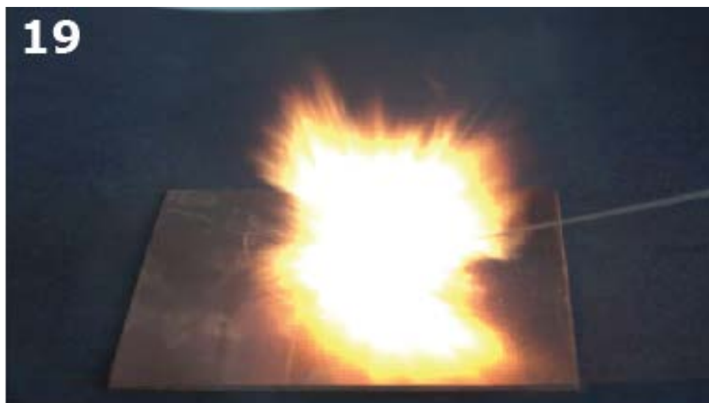
Figure S44 Moment of detonation of complex 19 during the hot needle test.
