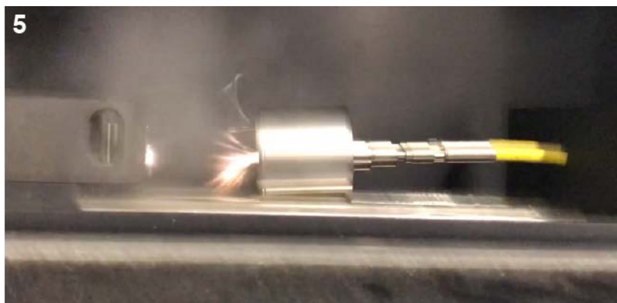
Figure S53 Detonation of 5 during the laser initiation test.
