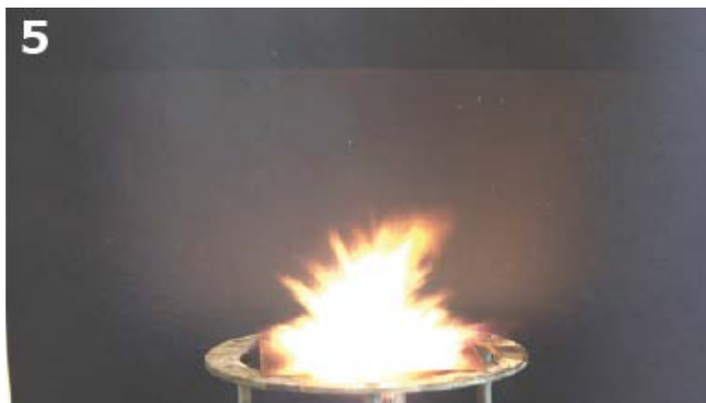
Figure S36 Detonation of coordination compound 5 during the hot needle and hot plate tests, partly shown as a sequence.
