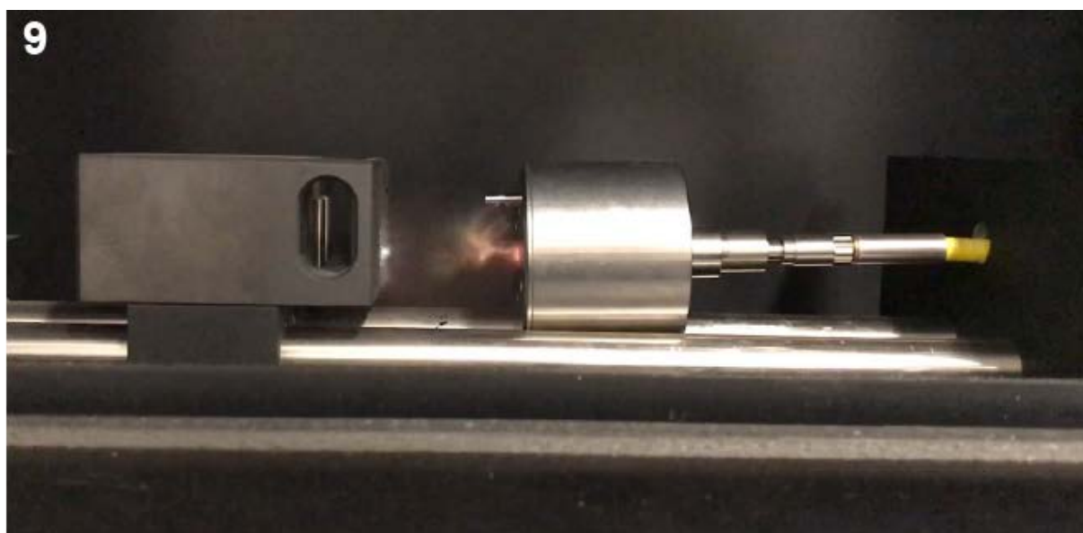
Figure S55 Moment of detonation of the copper(II) nitrate complex 9 .
