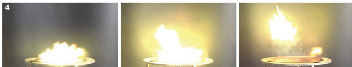
Figure S35 Hot plate test of coordination compound 4 shown as a sequence.
