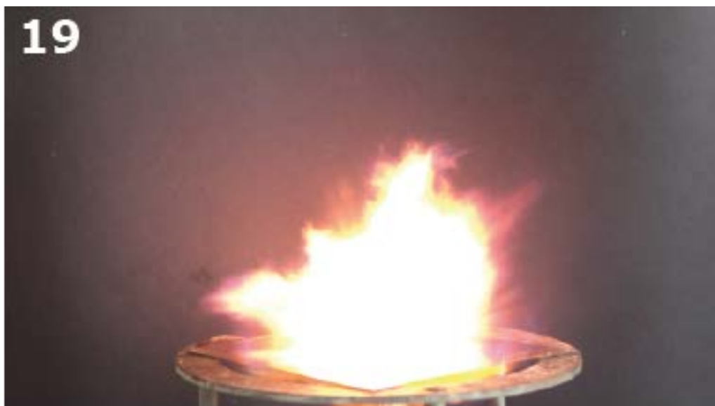
Figure S45 Moment of detonation of complex 19 during the hot plate test.
