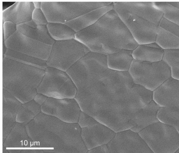
**Figure S1.** SEM image of nickel foam substrate.
