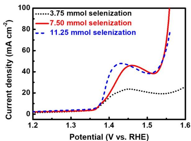
**Figure S7.** LSV curves of different production obtained with different selenium ratios.
