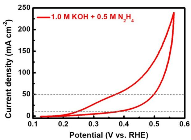
**Figure S10.** CV curve of HzOR in 1.0 M KOH with 0.5 M N<sub>2</sub>H<sub>4</sub>.
