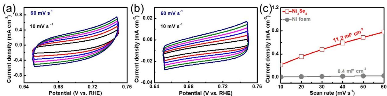
**Figure S8.** CV curves of (a)  $\text{Ni}_3\text{Se}_4$  and (b) Ni foam from  $10 \text{ mV s}^{-1}$  to  $60 \text{ mV s}^{-1}$ , (c) Cdl comparison of  $\text{Ni}_3\text{Se}_4$  and Ni foam.
