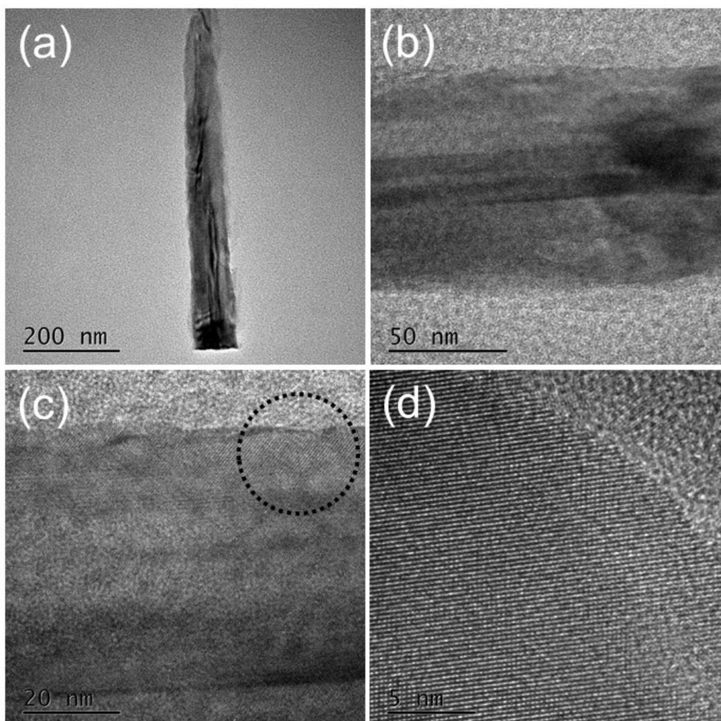
**Figure S2.** TEM images of Ni<sub>3</sub>Se<sub>4</sub> nanorod. Figure 1e and Figure S2d is derived from the selected area (black circle) of Figure S2c.
