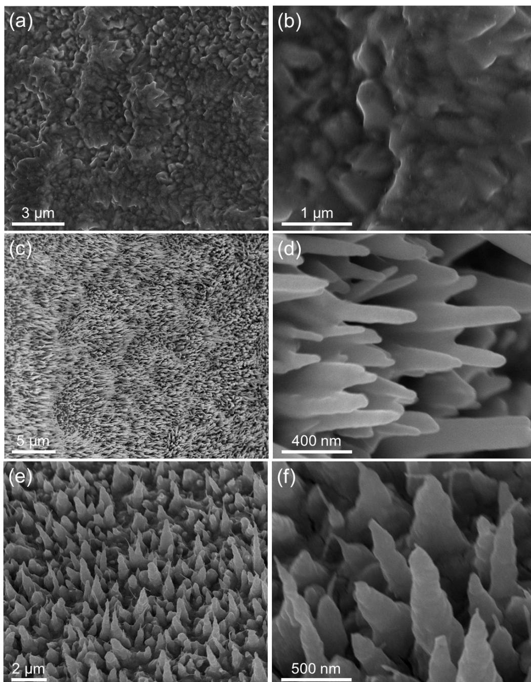
**Figure S3.** SEM images of different Se powder feeding ratio: a) and b) 3.75 mmol; c) and d) 7.5 mmol; e) and f) 11.25 mmol.
