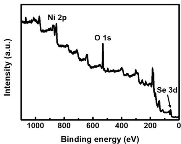
**Figure S5.** XPS survey spectrum of Ni<sub>3</sub>Se<sub>4</sub> sample.
