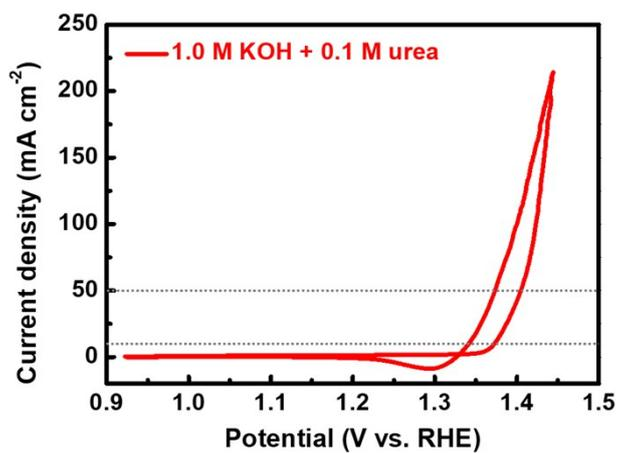
**Figure S9.** CV curve of UOR in 1.0 M KOH with 0.1 M urea.
