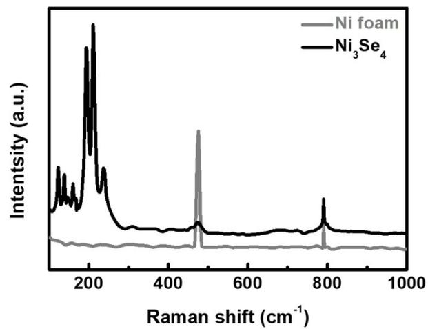
**Figure S4.** Raman spectrum of Ni<sub>3</sub>Se<sub>4</sub> and Ni foam.
