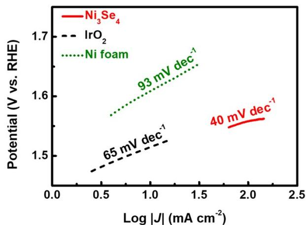
**Figure S6.** The corresponding OER Tafel slopes of  $\text{Ni}_3\text{Se}_4$ , Ni foam and  $\text{IrO}_2$ .
