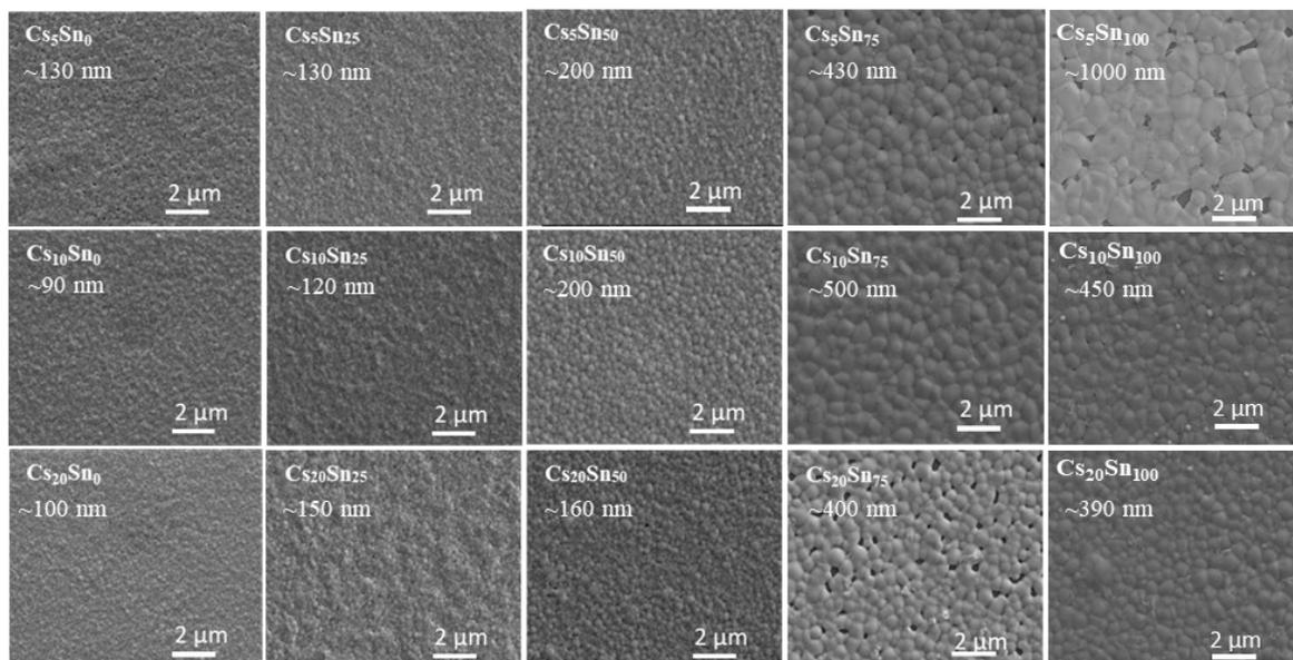
**Figure S1.** SEM images of  $Cs_x(MA_{0.17}FA_{0.83})_{1-x}Pb_{1-y}Sn_y(I_{0.83}Br_{0.17})_3$  perovskite thin films at 40,000 magnification with the average grain size of each film.
