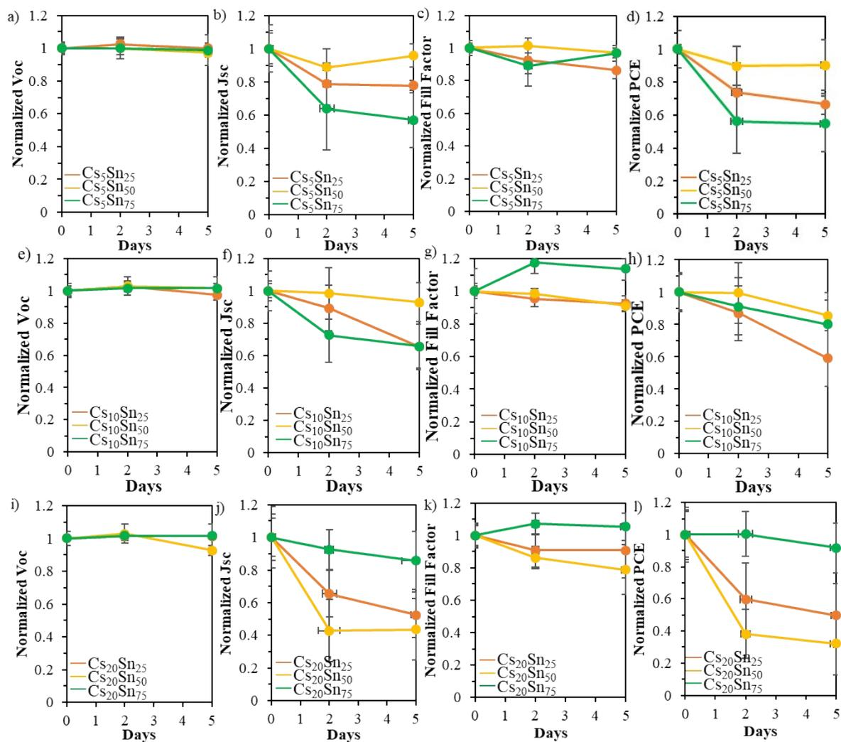
**Figure S6.** Normalized (a, e and i)  $V_{oc}$ , (b, f and j)  $J_{sc}$ , (c, g and k) FF, and (d, h and l) PCE of  $Cs_x(MA_{0.17}FA_{0.83})_{1-x}Pb_{1-y}Sn_y(I_{0.83}Br_{0.17})_3$  PVSCs for 5, 10 and 20% Cs, respectively, with Sn from 0 to 75% for each Cs composition, over time in ambient conditions after stored in glove box for 30 days.
