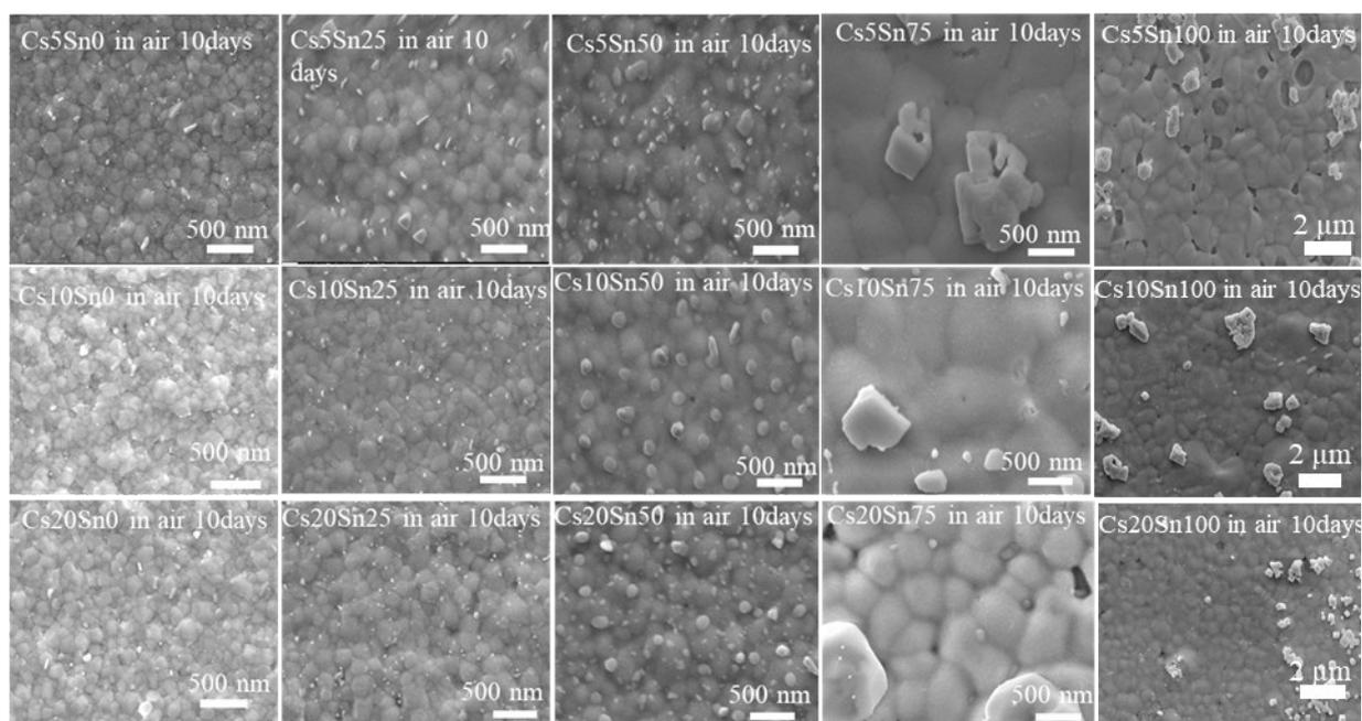
**Figure S8.** SEM images of  $\text{Cs}_x(\text{MA}_{0.17}\text{FA}_{0.83})_{1-x}\text{Pb}_{1-y}\text{Sn}_y(\text{I}_{0.83}\text{Br}_{0.17})_3$  perovskite films after 10 days of air exposure.
