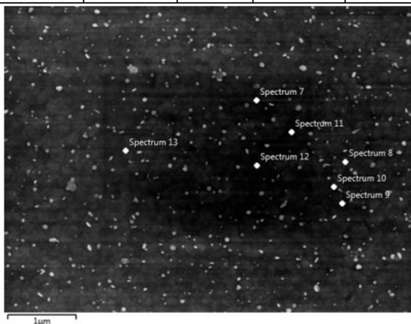
**Figure S9.** SEM image with the spots where EDS measurements were taken for  $\text{Cs}_{20}\text{Sn}_{25}$  thin film after 10 days of air exposure
