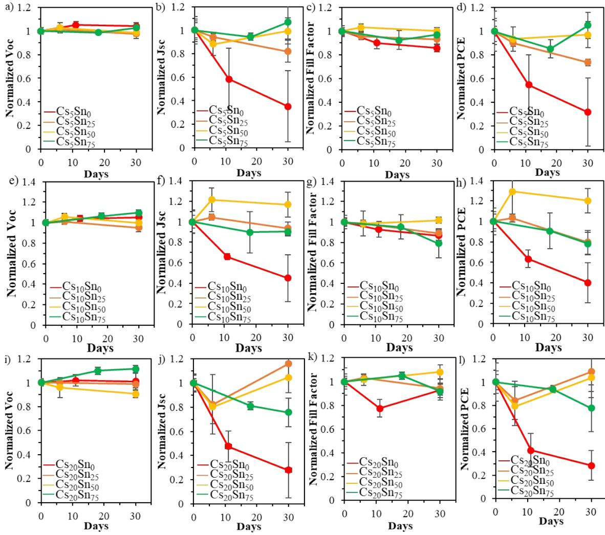
**Figure S5.** Normalized (a, e and i)  $V_{oc}$  (b, f and j)  $J_{sc}$ , (c, g and k) FF, and (d, h and l) PCE of  $Cs_x(MA_{0.17}FA_{0.83})_{1-x}Pb_{1-y}Sn_y(I_{0.83}Br_{0.17})_3$  PVSCs for 5, 10 and 20% Cs, respectively, with Sn from 0 to 75% for each Cs composition, over time in the glovebox.
