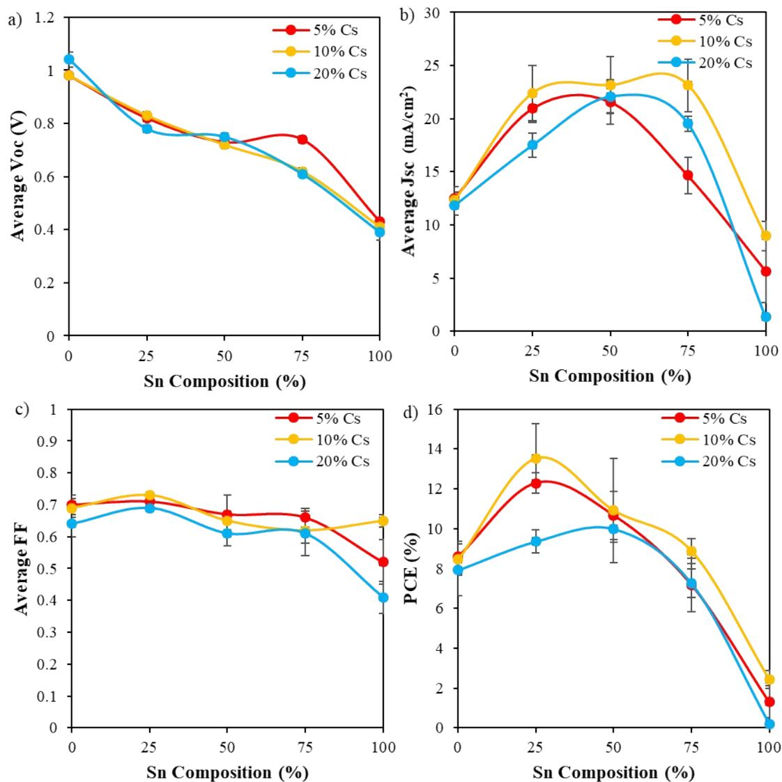
**Figure S4.** The averages of a)  $V_{oc}$ , b)  $J_{sc}$ , c) FF, and d) PCE of PVSCs as a function of Sn composition for different Cs contents with  $Cs_x(MA_{0.17}FA_{0.83})_{1-x}Pb_{1-y}Sn_y(I_{0.83}Br_{0.17})_3$  perovskite thin films as the active layers.
