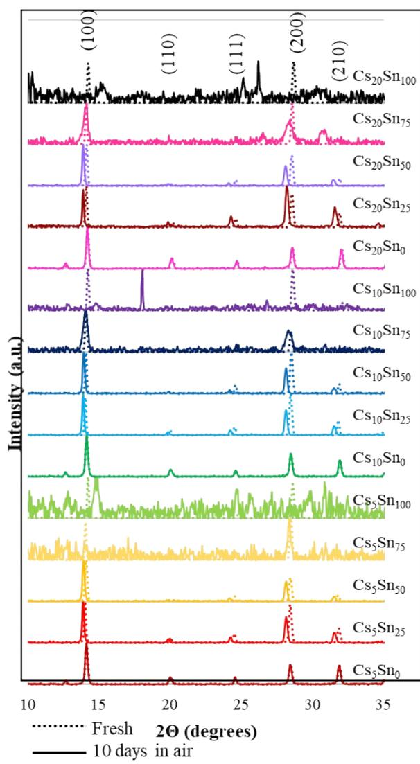
**Figure S7.** XRD patterns of pristine (dashed lines) and after 10 days of air exposure (solid lines) of the  $\text{Cs}_x(\text{MA}_{0.17}\text{FA}_{0.83})_{1-x}\text{Pb}_{1-y}\text{Sn}_y(\text{I}_{0.83}\text{Br}_{0.17})_3$  perovskite thin films.
