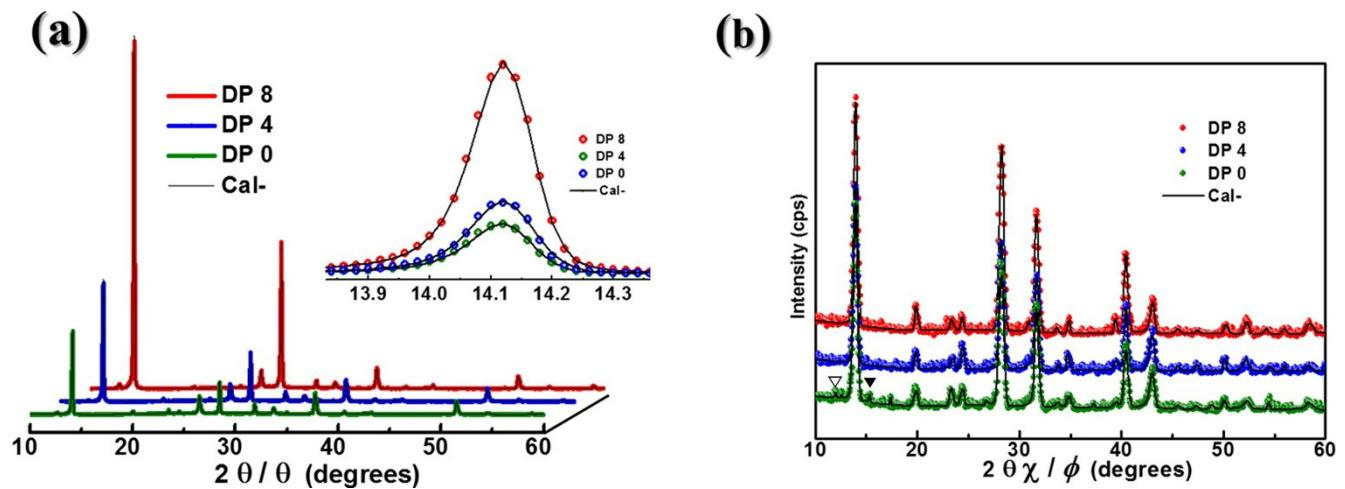
**Figure S1.** (a) Out-of-plane and (b) In-plane diffraction patterns of the perovskite films fabricated at various DPs. The X-ray beam was collimated with a beam slit analyzer.
