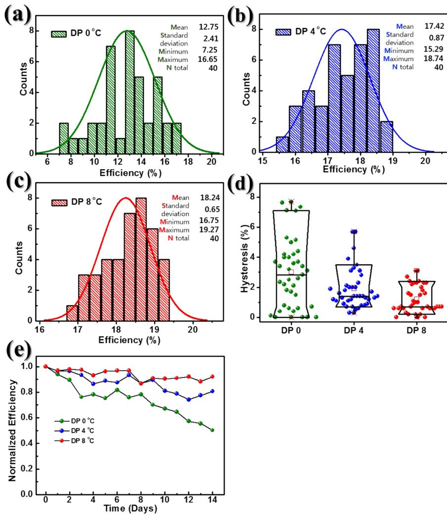
**Figure S2.** (a)-(c) Statistical results of the perovskite photovoltaics fabricated at various DPs. (d) Hysteresis of the perovskite photovoltaics in the statistical results defined as differences in efficiencies between reverse and forward scans. (e) Long term stability of non-encapsulated devices; the devices were stored in the dark under dry air and J-V curves were periodically measured under ambient condition ( 25–40% humidity, 18–27 °C).
