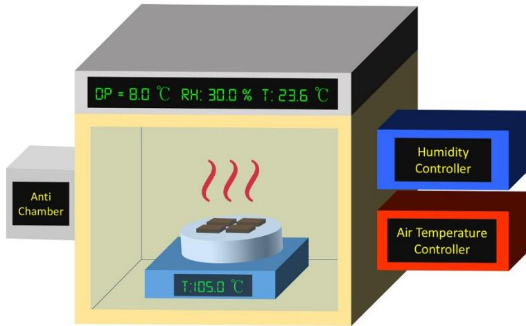
**Figure S4.** Schematic illustration of annealing system to adjust thermal equilibrium with relative humidity (RH).
