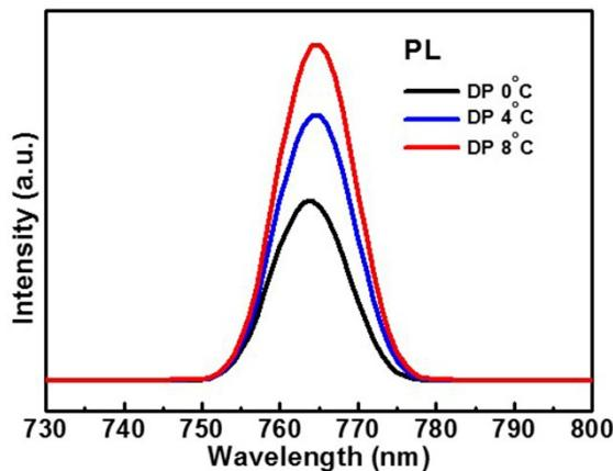
**Figure S3.** Steady-state photoluminescence spectra for the perovskite films fabricated at various DPs.
