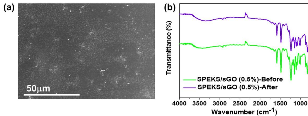
**Fig. S15** (a) FE-SEM image of SPEKS/sGO (0.5%) membrane surface after 300 charge-discharge cycle of the VRB. (b) FT-IR spectra of SPEKS/sGO (0.5%) membrane before and 300 charge-discharge cycles of the VRB.
