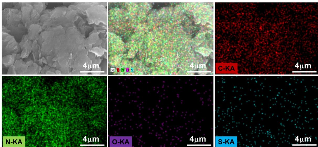
**Fig. S2.** FE-SEM elemental mapping of sample graphene oxide (GO).
