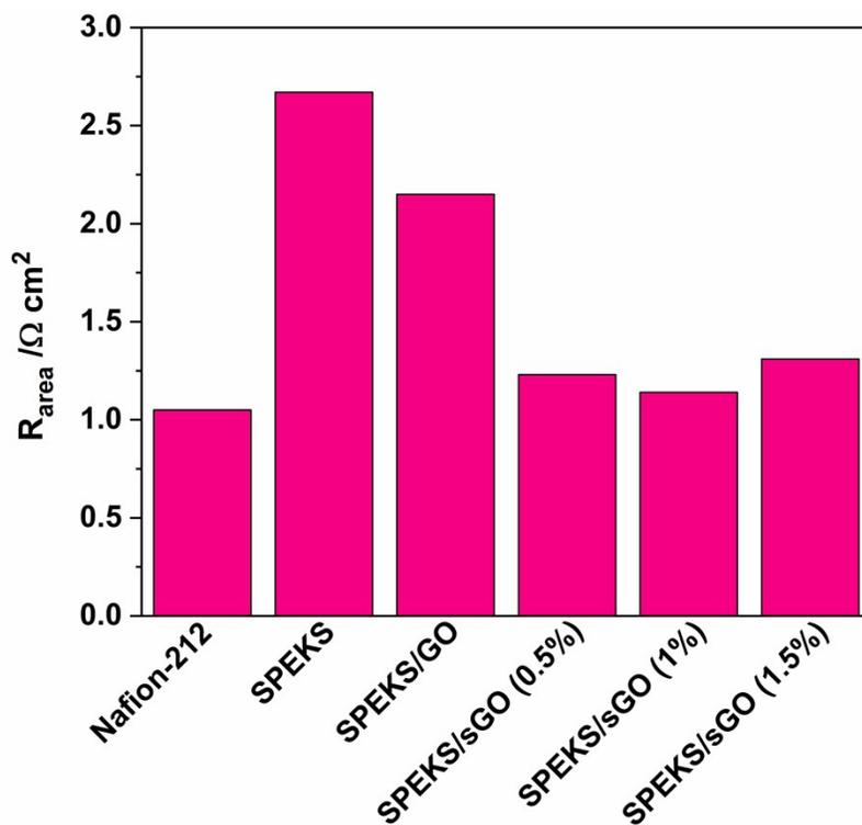
**Fig. S12** Areal resistance of the samples of Nafion-212, SPEKS, SPEKS/GO, SPEKS/sGO (0.5%), SPEKS/sGO (1%) and SPEKS/sGO (1.5%) membranes.
