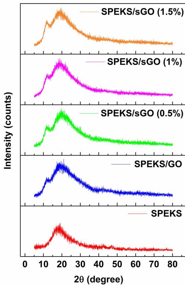
**Fig. S5** Powder X-ray diffraction pattern of samples SPEKS, SPEKS/GO, SPEKS/sGO (0.5%), SPEKS/sGO (1%) and SPEKS/sGO (1.5%) membranes.
