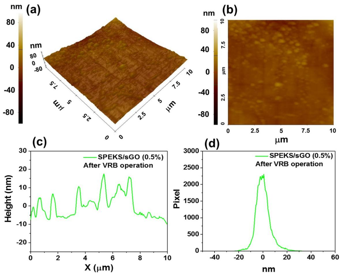
**Fig. S14** AFM analysis: (a) 3D image, (b) Topography, (c) Line profile and (d) Histogram of the SPEKS/sGO (0.5%) composite membrane after 300 charge-discharge cycles in the VRB.
