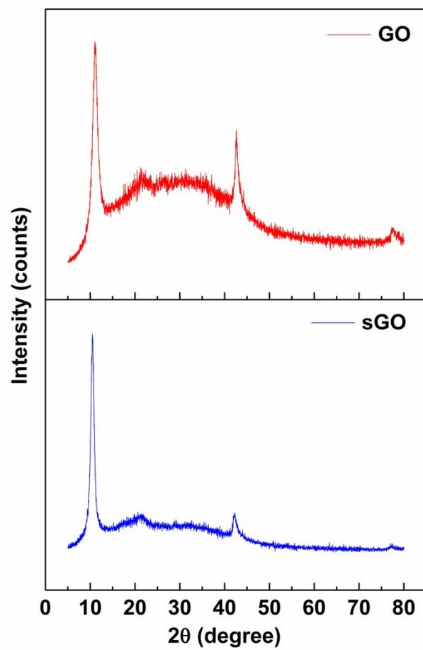
**Fig. S4** Powder X-ray diffraction pattern of GO and sGO.
