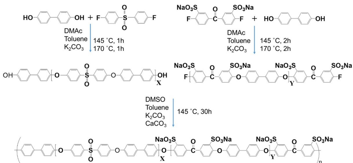
**Fig. S1** Schematic description of synthesis of hydrophobic, hydrophilic and block copolymers.
