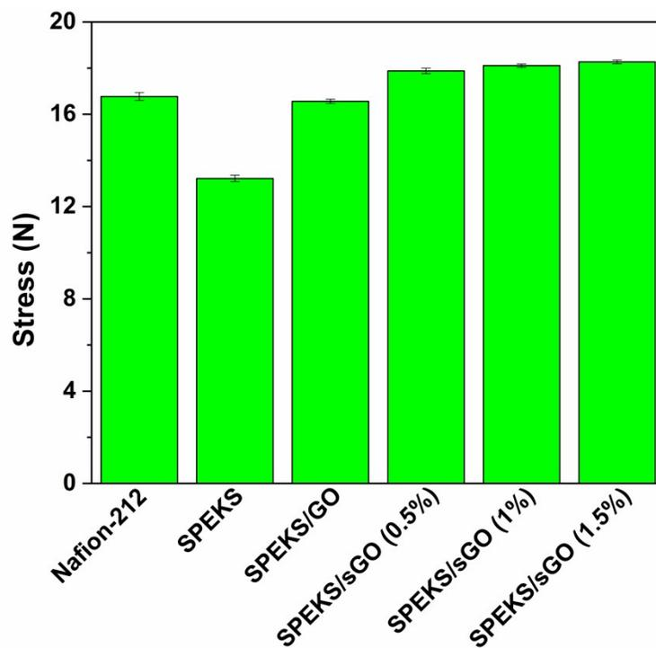
**Fig. S11** The tensile stress of Nafion-212, SPEKS, SPEKS/GO, SPEKS/sGO (0.5%), SPEKS/sGO (1%) and SPEKS/sGO (1.5%) membranes.
