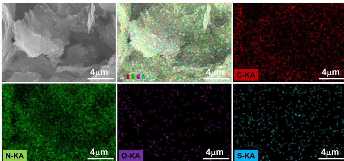
**Fig. S3** FE-SEM elemental mapping of sample sulfonated graphene oxide (sGO).
