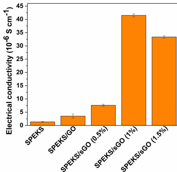
**Fig. S10** The electrical conductivity measurement of SPEKS, SPEKS/GO, SPEKS/sGO (0.5%), SPEKS/sGO (1%) and SPEKS/sGO (1.5%) membranes.
