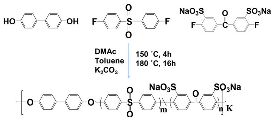
**Fig. S16** Schematic description of synthesis of random sulfonated poly(ether ketone sulfone) copolymer membrane.
