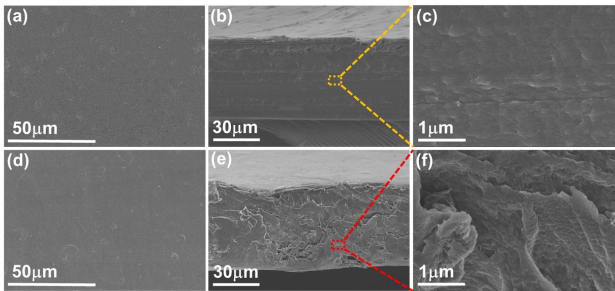
**Fig. S7** FE-SEM image of SPEKS membrane (a) Surface, (b) and (c) Cross-section; SPEKS/sGO (0.5%) membrane (d) Surface, (e) and (f) Cross-section.
