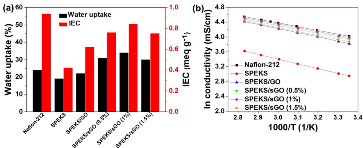
**Fig. S9** (a) Water uptake and IEC value of Nafion-212, SPEKS, SPEKS/GO, SPEKS/sGO (0.5%), SPEKS/sGO (1%) and SPEKS/sGO (1.5%) membranes. (b) Regression curve of proton conductivity with  $T^{-1}$  for Nafion-212, SPEKS, SPEKS/GO, SPEKS/sGO (0.5%), SPEKS/sGO (1%) and SPEKS/sGO (1.5%) membranes measured at 25 to 80 °C under 100% RH.
