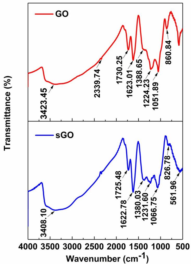
Fig. S6 FT-IR spectra of GO and sGO.
