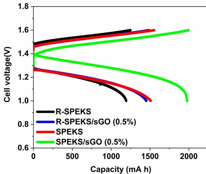
**Fig. S17** VRB charge-discharge capacity of random copolymer membrane R-SPEKS, pure SPEKS block copolymer and their composite membranes.
