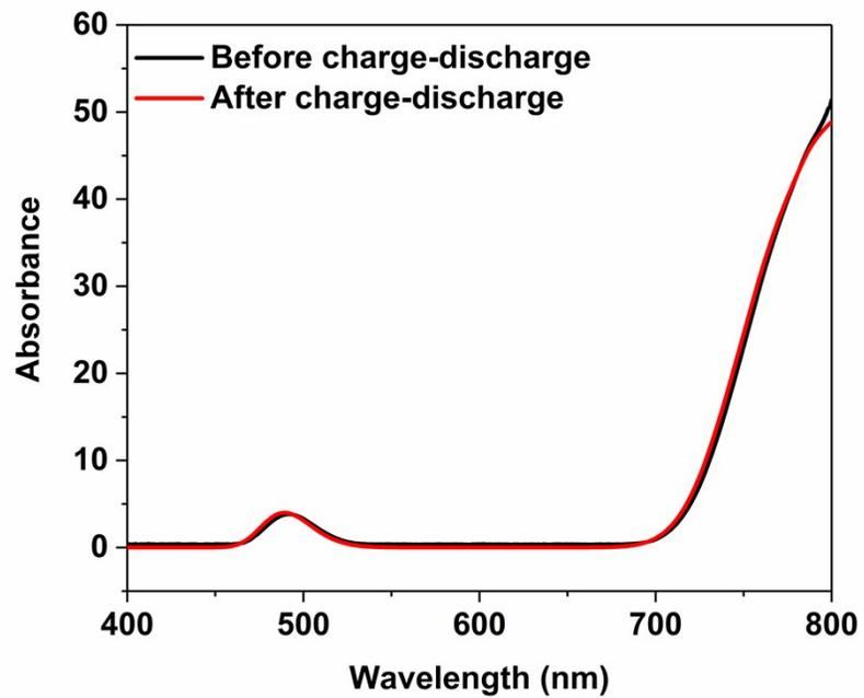
**Fig. S13** UV-vis. absorption spectra of the vanadium electrolyte solution at before and after 300 charge-discharge cycles in the VRB.
