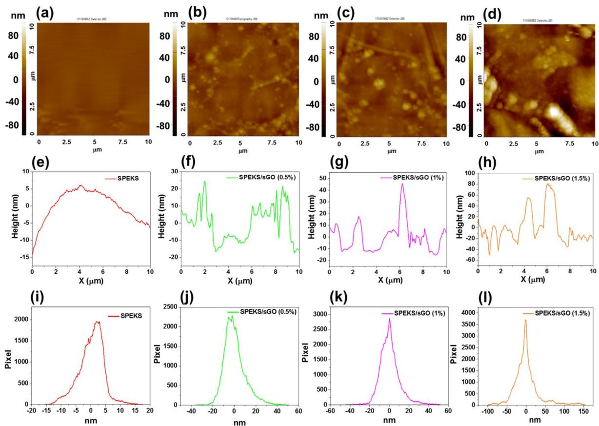
**Fig. S8** Topography: (a) SPEKS, (b) SPEKS/sGO (0.5%), (c) SPEKS/sGO (1%) and (d) SPEKS/sGO (1.5%) membranes. Line profile: (e) SPEKS, (f) SPEKS/sGO (0.5%), (g) SPEKS/sGO (1%) and (h) SPEKS/sGO (1.5%) membranes. Histogram: (i) SPEKS, (j) SPEKS/sGO (0.5%), (k) SPEKS/sGO (1%) and (l) SPEKS/sGO (1.5%) membranes.
