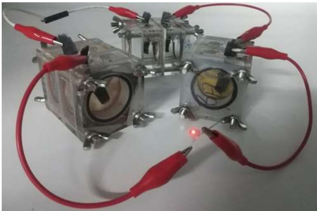
Figure S11. Photograph of a red LED (about 1.8-2.2 V) powered by three HzOR-HER asymmetric-electrolyte cell with \text{Ni}_{0.5}\text{Co}_{0.5}\text{Se}_2 as the electrodes
