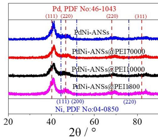
**Fig. S4** XRD patterns of PdNi-ANSs without PEI, PdNi-ANSs@PEI1800, PdNi-ANSs@PEI10000, and PdNi-ANSs@PEI70000.
