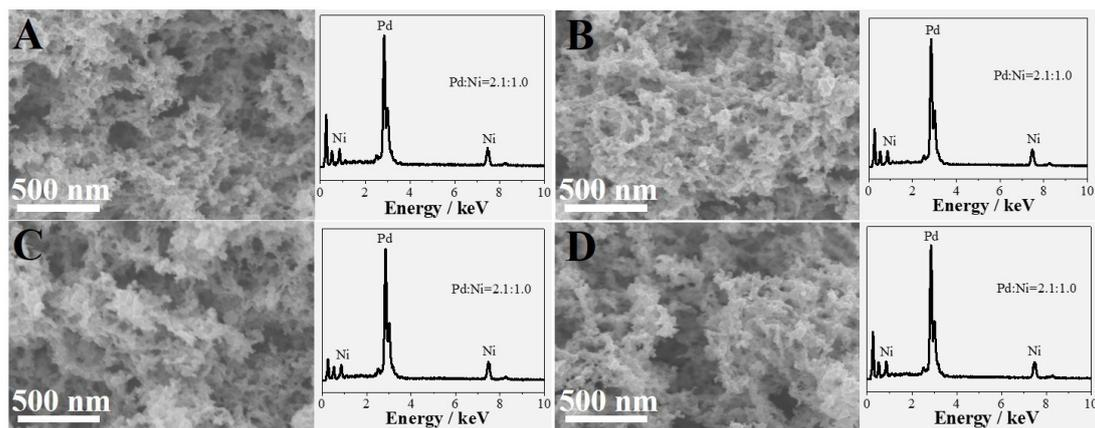
**Fig. S3** SEM images and EDX spectra of (A) PdNi-ANSs, (B) PdNi-ANSs@PEI1800, (C) PdNi-ANSs@PEI10000, and (D) PdNi-ANSs@PEI70000.
