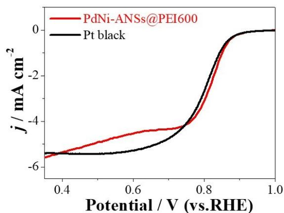
**Fig. S6** ORR polarization curves of PdNi-ANSs@PEI600 and commercial Pt black in  $O_2$ -saturated 0.5 M  $H_2SO_4$  solution at a sweep rate of  $10 \text{ mV s}^{-1}$  and a rotation rate of 1600 rpm.
