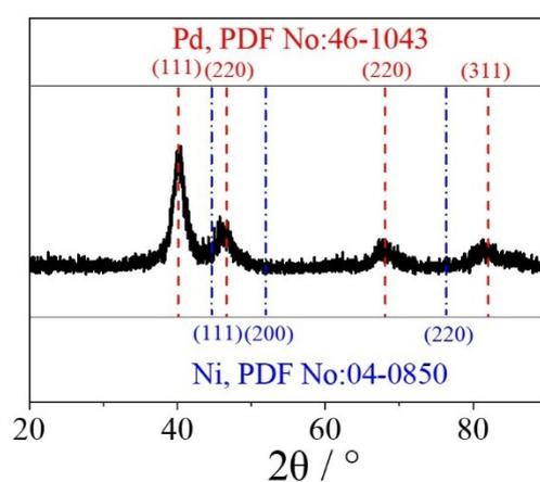
**Fig. S2** XRD pattern of PdNi bimetallic nanoparticles by using mixture of  $K_2PdCl_4$  and  $NiCl_2$  as precursors.
