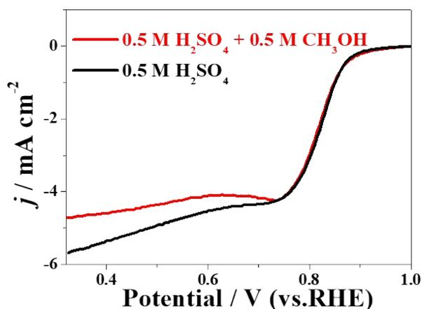
**Fig. S7** ORR polarization curves of PdNi-ANSs@PEI600 in O<sub>2</sub>-saturated 0.5 M H<sub>2</sub>SO<sub>4</sub> and 0.5 M H<sub>2</sub>SO<sub>4</sub> + 0.5 M CH<sub>3</sub>OH solution at a sweep rate of 10 mV s<sup>-1</sup> and a rotation rate of 1600 rpm.
