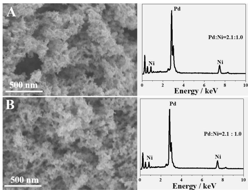
**Fig. S10** SEM images and EDX spectra of PdNi-ANSs@PEI600 after the stability test for (A) ORR and (B) HER.
