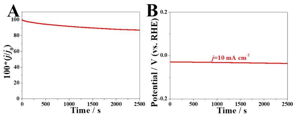
**Fig. S9** (A) Chronoamperometry and (B) chronopotentiometry curves of PdNi-ANSs@PEI600 in O<sub>2</sub>-saturated ( $E=0.7$  V) and N<sub>2</sub>-saturated 0.5 M H<sub>2</sub>SO<sub>4</sub> ( $j=10$  mA cm<sup>-2</sup>), respectively.
