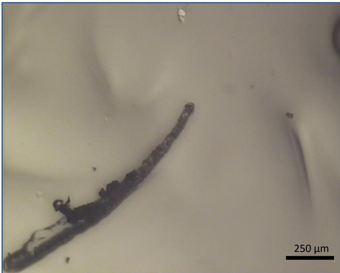
**Figure S3:** Crack made with a scalpel induced into the metallopolymer based on poly(butyl methacrylate) crosslinked via manganese(II)-chloride-terpyridine interactions. Cracks and ridges can be seen on the crack edge.
