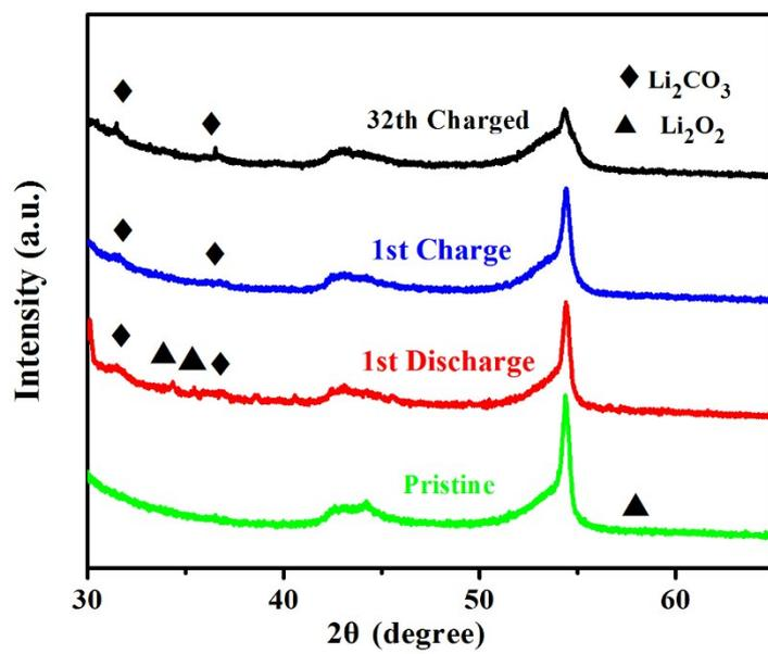
Fig. S9 XRD patterns of N-C cathode at different stages.
