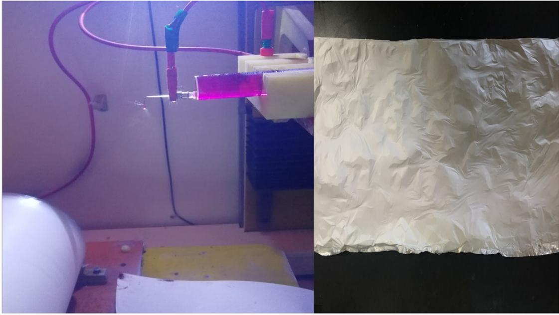
**Fig. S1** Photo of the electrospinning process to fabricate the nanofibers with collected  $\text{Co}(\text{NO}_3)_2/\text{PVP}$  mat on Al foil.
