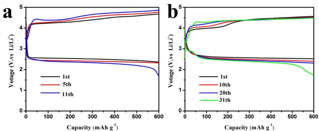
**Fig. S7** The cycle performance of a) Super P carbon and b) N-C cathode at a current density of  $100 \text{ mA g}^{-1}$  with a specific capacity limit of  $600 \text{ mAh g}^{-1}$ .
