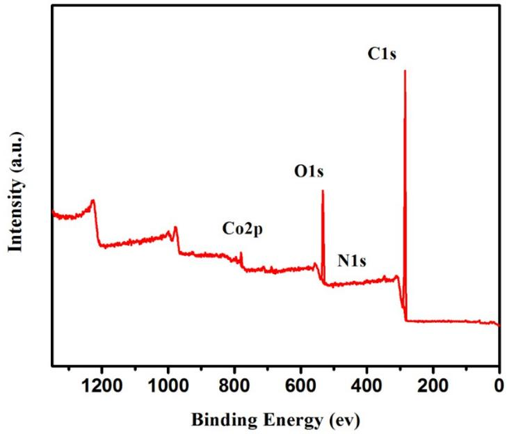
**Fig. S5** XPS survey spectra of CoO/Co-N-C, and the content of C, N, O and Co elements are C 85.38 at%, N 0.82 at%, O 13.51at%, and Co 0.29 at%, respectively.
