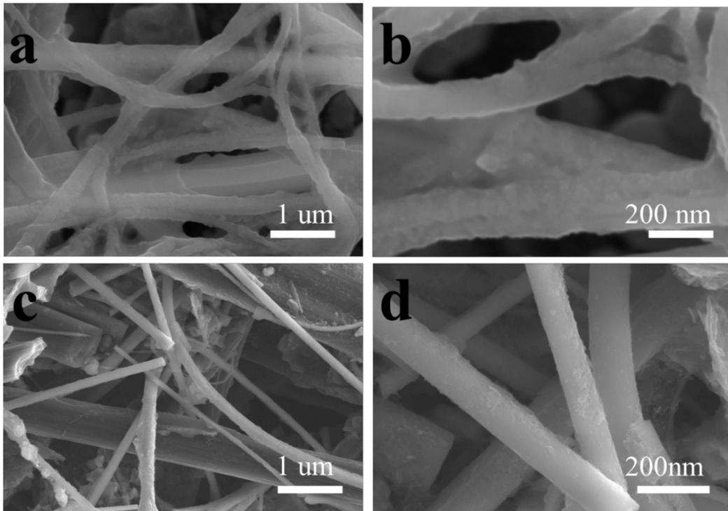
**Fig. S8** SEM images of CoO/Co-N-C-2 cathodes at different stages a) and b) after 140th discharged; c) and d) after 140th charged.
