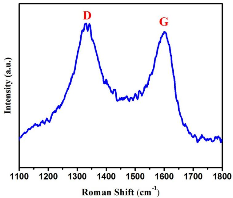
**Fig. S6** Raman spectra of CoO/Co-N-C-2 with the corresponding intensity ratio of D and G bands ( $I_D/I_G=1.094$ ).
