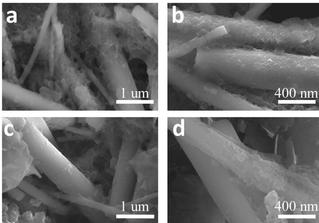
**Fig. S10** SEM images of N-C cathode at different stages under a current of  $100 \text{ mAh g}^{-1}$ : a) and b) after 1st discharged; c) and d) after 1st charged.
