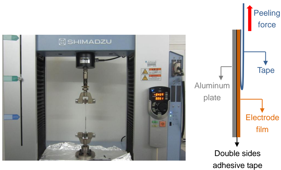
Fig. S11 Optical image of the setup, and schematic of the sample for the peeling test.
