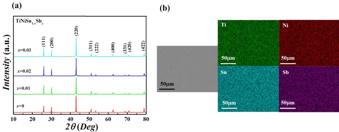
**Fig. S7** (a) XRD patterns of the products after SHS-SPS of TiNiSn<sub>1-x</sub>Sb<sub>x</sub> ( $x = 0, 0.01, 0.02, 0.03$ ) (b) element distribution of the polished surface of TiNiSn<sub>0.99</sub>Sb<sub>0.01</sub> after SHS-SPS
