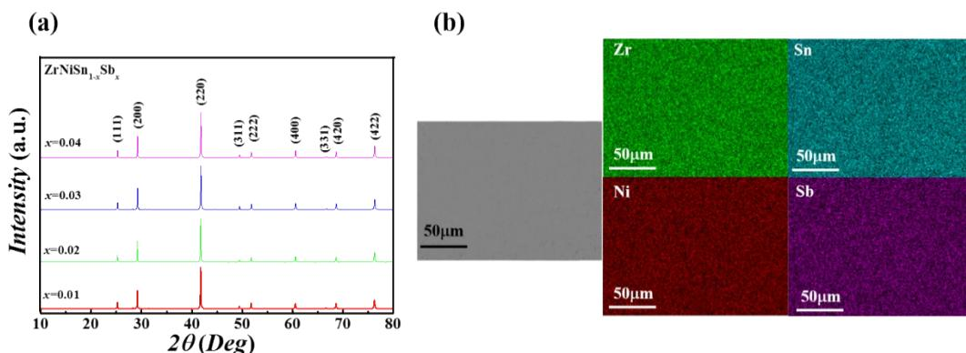
**Fig. S1** (a) XRD patterns of the products after SHS-SPS of ZrNiSn<sub>1-x</sub>Sb<sub>x</sub> ( $x = 0.01, 0.02, 0.03, 0.04$ ) (b) element distribution of the polished surface of ZrNiSn<sub>0.99</sub>Sb<sub>0.01</sub> after SHS-SPS
