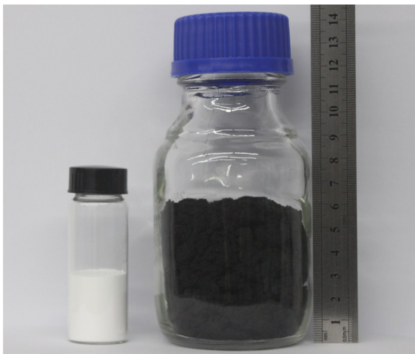
Figure S8. A photo picture showing bulk quantity of N-doped GNRs products, in which ~1 g N-doped GNRs can be fabricated from ~11 g DPA@AEL crystals.
