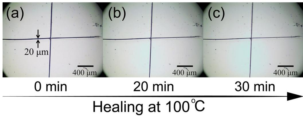
**Fig. S6** Digital images during the healing process of LP2-HE-HP film.
