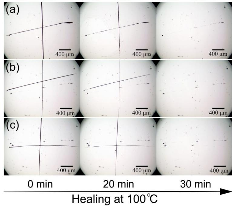
**Fig. S3** Digital images during the scratch healing process on the same location of LP2-SS-HP film left in air for 24 h before starting self-healing (a: the 1<sup>st</sup> healing process; b: the 2<sup>nd</sup> healing; c: the 3<sup>rd</sup> healing process).
