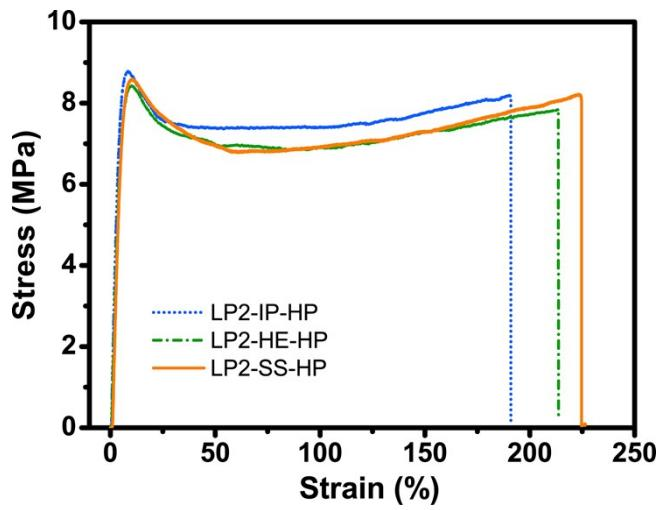
**Fig. S4** Tensile stress–strain curves of LP2-IP-HP, LP2-HE-HP and LP2-SS-HP films.
