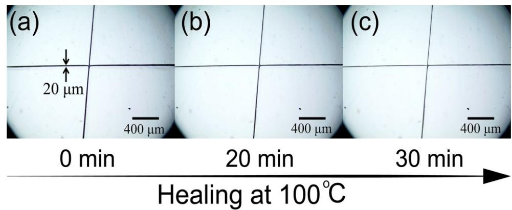
**Fig. S5** Digital images during the healing process of LP2-IP-HP film.
