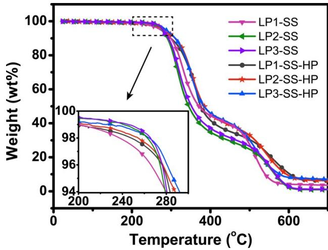
**Fig. S2** TGA curves of LP<sub>x</sub>-SS-HP and LP<sub>x</sub>-SS under N<sub>2</sub> atmosphere.
