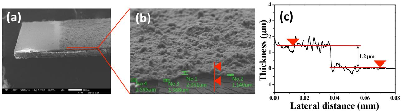
**Figure S3.** (a) Cross-sectional SEM images of the PPy3DrGO/npAu based electrode surface, deposited on a PET substrate; (b) magnified view showing average thickness of the deposited hybrid material on the current collector (c) Surface profiling of the selected area shows material thickness to be around 1.2 μm. (Red probes are shown in (b) and (c) for the representations only)
