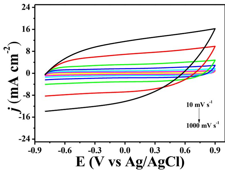
**Figure S9.** CV analysis showing retention of voltammogram shapes of the all-solid-state in-plane MSC based on Ppy-3DrGO composite material even at high scan rates.
