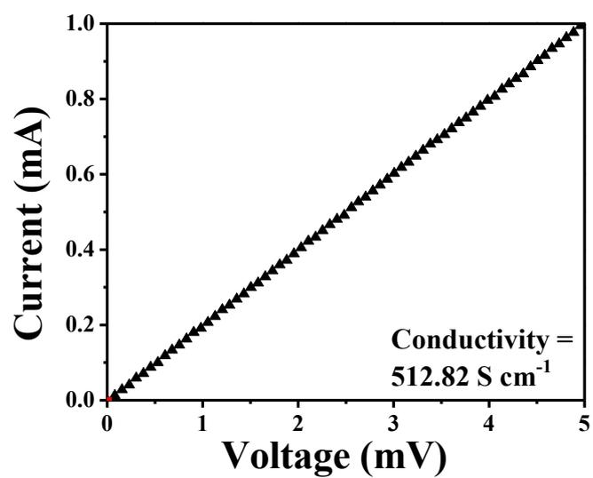
**Figure S6.** Electrical conductivity measurement (I-V characterization) of the hybrid material, PPy-3DrGO on npAu current collector via two-probe method.
