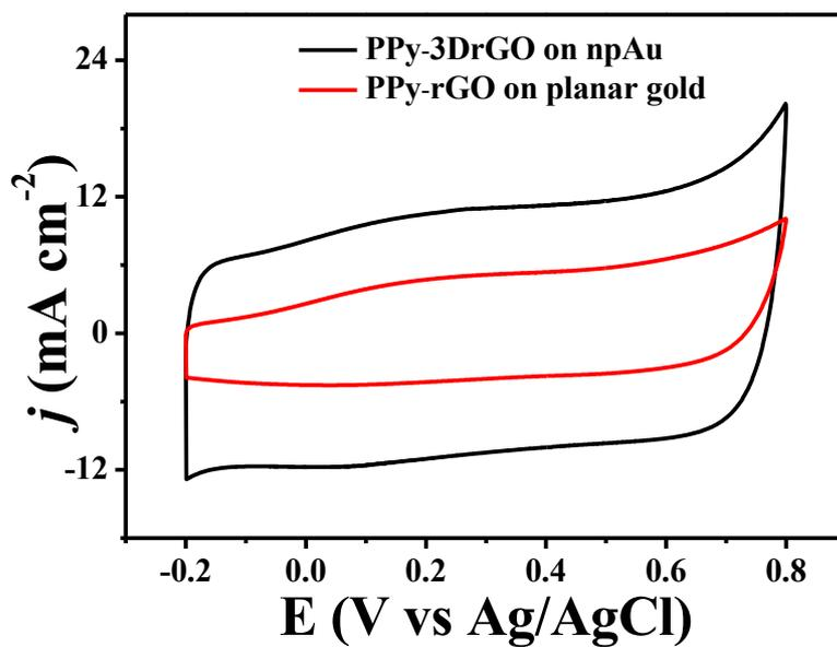
**Figure S8.** Comparative cyclic voltammetric analyses showing the influence of npAu as compared to a planar gold substrate in increasing the capacitive properties of the reduced graphene oxide-conducting polymer (PPy-3DrGO) composite material.
