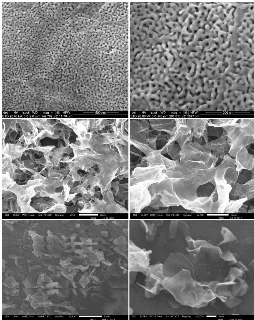
**Figure S1.** Microscopic images of the surfaces of the current collector and the active electrode materials on the current collector; **(a)-(b)** npAu, **(c)-(d)** 3DrGO/npAu and **(e)-(f)** PPy/npAu electrodes (top view) at various resolutions. Scale bar: 300 nm, 500 nm, 1 μm, 10 μm, 20 μm.
