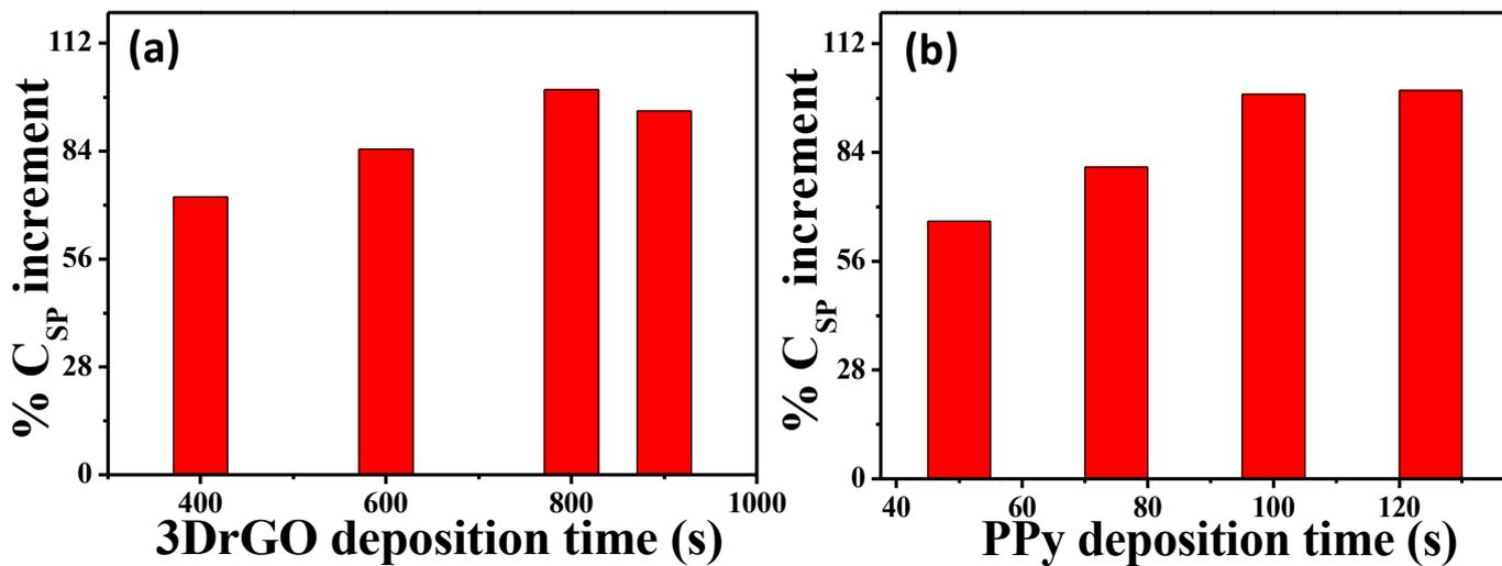
**Figure S7.** Effect of concentration of the analyte on the percentage specific capacitance of the developed PPy-3DrGO hybrid electrode material (a) 3DrGO; (b) PPy.
