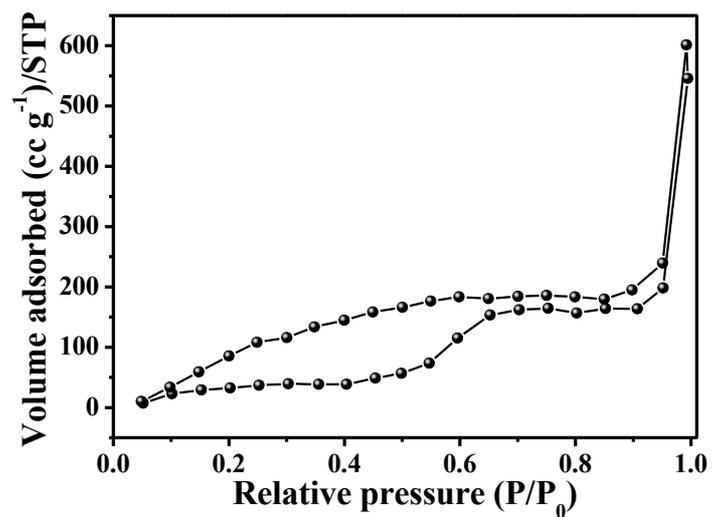
**Figure S5.** BET surface area analysis of the hybrid material, PPy-3DrGO by N<sub>2</sub> sorption analysis isotherm.
