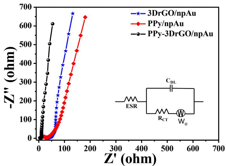
**Figure S10.** Comparative Nyquist plot showing enhanced capacitive property of the PPy-3DrGO composite material. Inset shows the equivalent circuit used to fit the EIS spectra).
