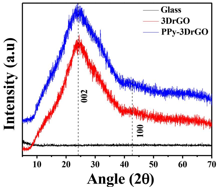
**Figure S4.** XRD spectra of the active materials, 3DrGO and PPy-3DrGO on a glass substrate.
