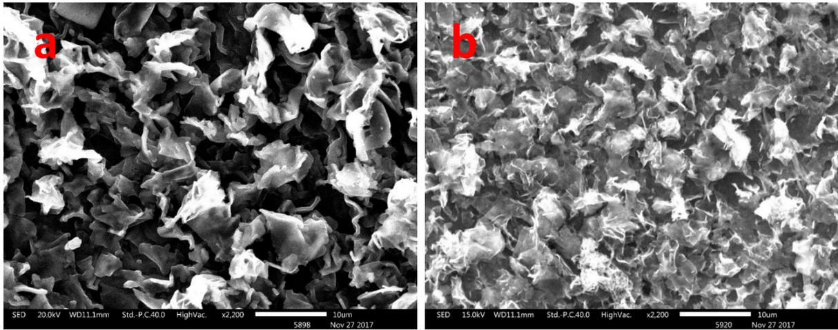
**Figure S11.** SEM images of the solid-state symmetric supercapacitor electrode surface obtained (a) before and (b) after 10000 cycles of charge-discharge at a high current density of  $5 \text{ mA cm}^{-2}$ .
