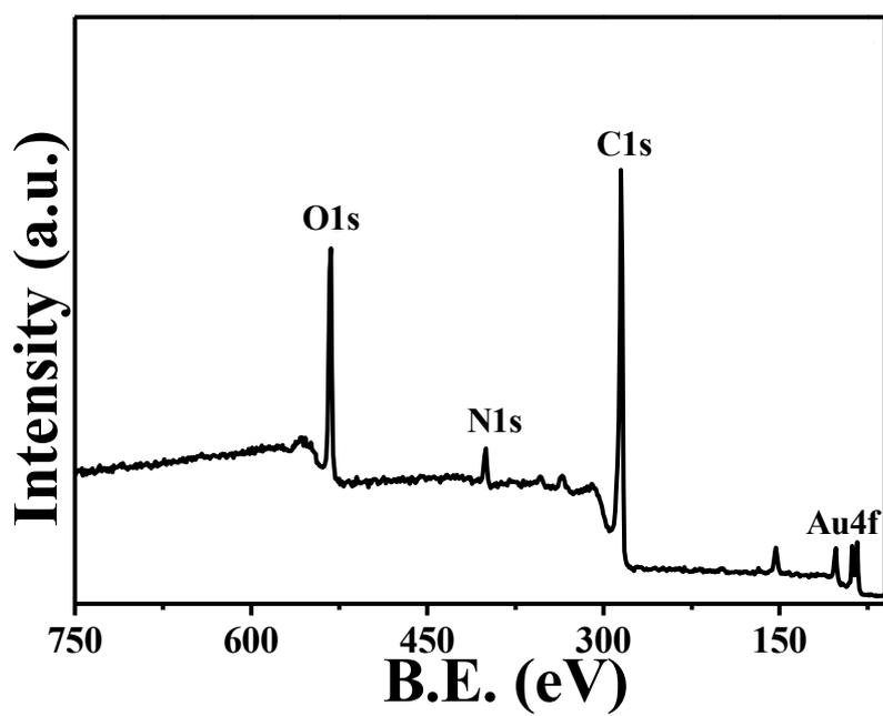
**Figure S2.** The overall XPS spectra of the PPy-3DrGO hybrid material on npAu substrate.
