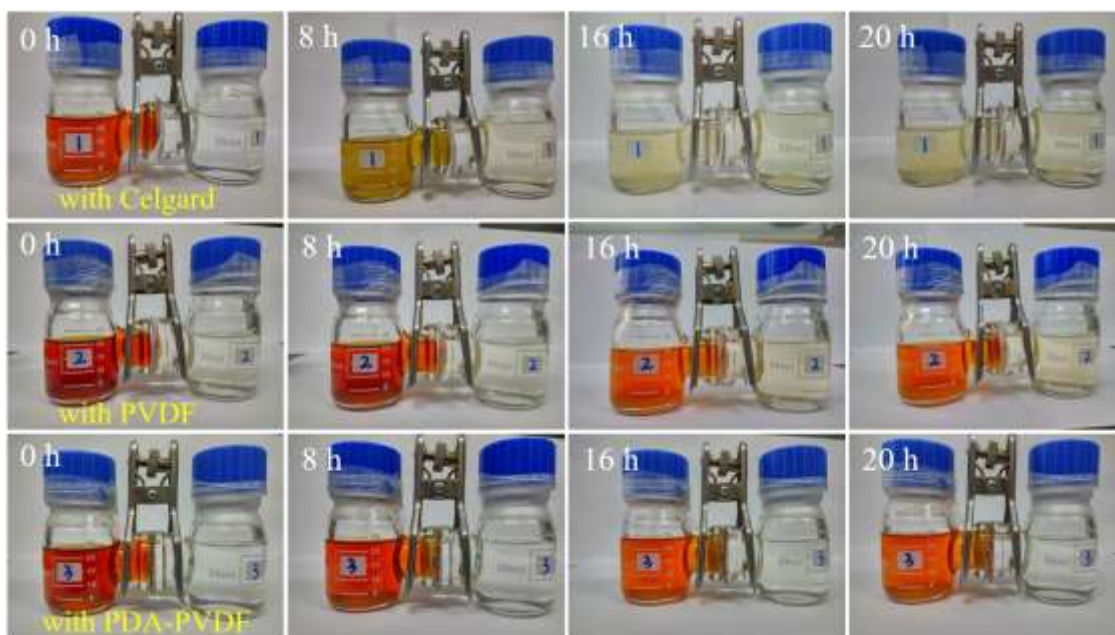
Fig. S6. The photos for the diffusion of polysulfides in the H-type cells with Celgard, PVDF and PDA-PVDF films.
