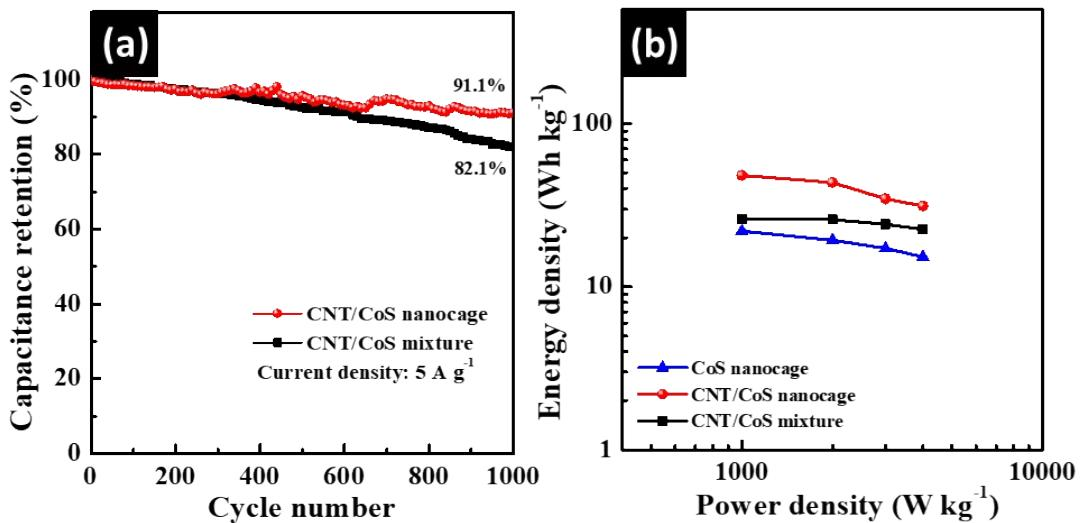
**Figure S12** (a) Cycling performance of hybrid CNT/CoS nanocage and CNT/CoS mixture, and (b) Ragone plot of CoS nanocage, hybrid CNT/CoS nanocage and CNT/CoS mixture under various current densities in three-electrode system.
