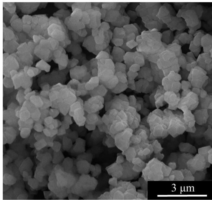
**Figure S2** FE-SEM images of ZIF-67 nanoparticles synthesized with PVP.
