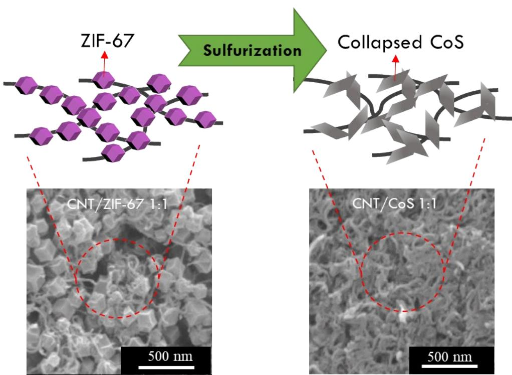
**Figure S7** FE-SEM images of CNT/ZIF-67 1:1, CNT/CoS 1:1 and the schematic illustration of the collapsed CoS *via* sulfurization.
