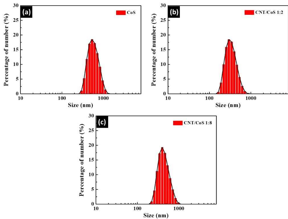
**Figure S6** Particle size distributions of (a) CoS, (b) CNT/CoS 1:2 and (c) CNT/CoS 1:8.
