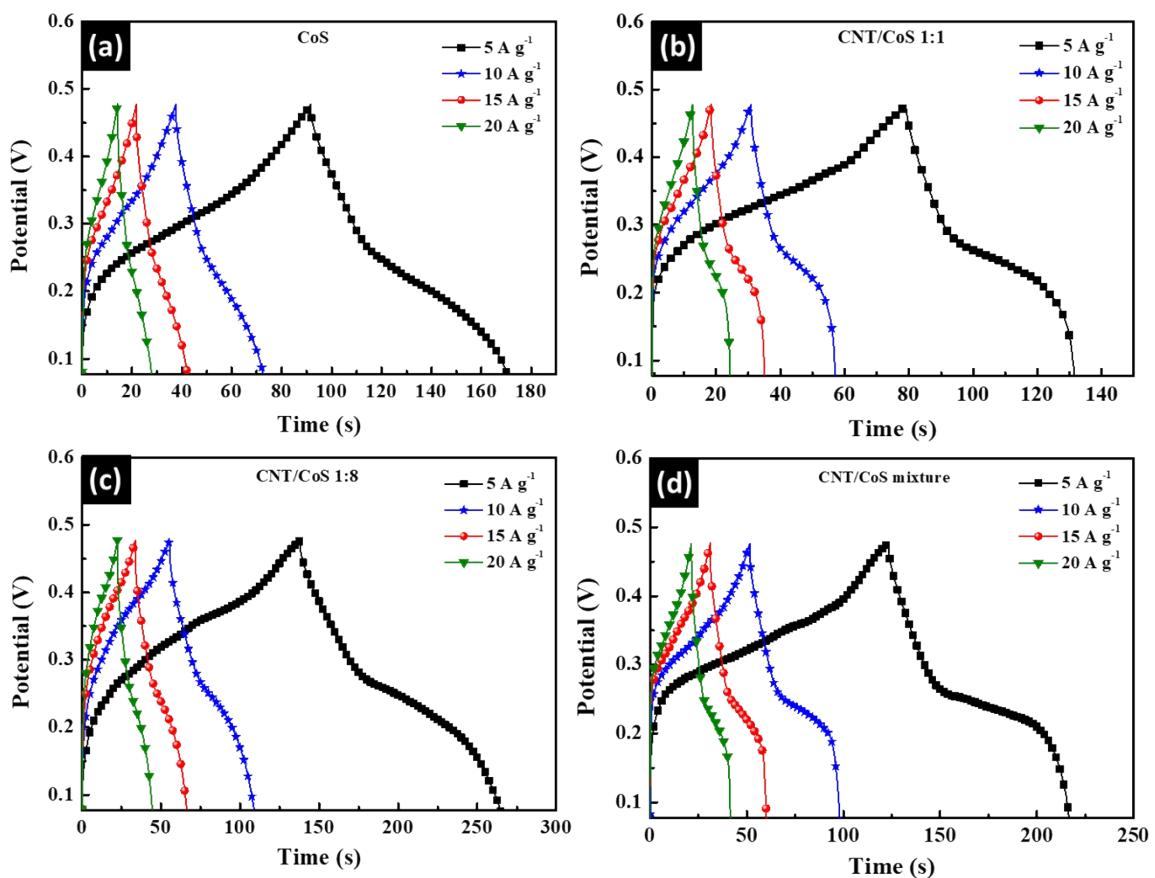
**Figure S10** GCD curves of (a) CoS nanocage, (b) CNT/CoS 1:1 nanocage, (c) CNT/CoS 1:8 nanocage, and (d) CNT/CoS mixture electrodes at different current densities.
