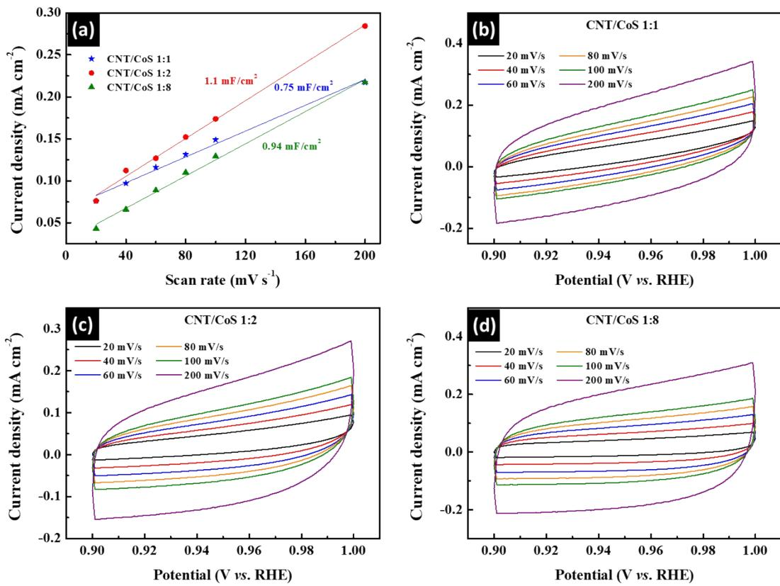
**Figure S11** Electrochemical active surface area using CVs recorded in non-faradic region at different scan rates. (a) Linear fits of anodic current density measured at 0.95 V (vs. RHE) versus scan rate plots. (b) CNT/CoS 1:1 nanocage, (c) CNT/CoS 1:2 nanocage and (d) CNT/CoS 1:8 nanocage.
