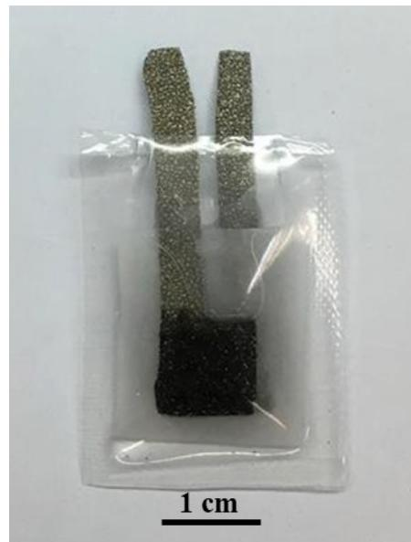
**Figure S13** A photograph of the symmetric supercapacitor of hybrid CNT/CoS nanocage as electrodes.
