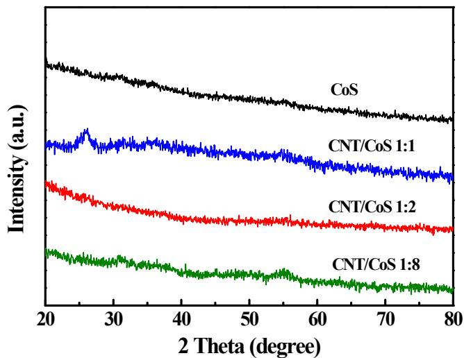
**Figure S8** XRD patterns of CoS cage and hybrid CNT/CoS nanocages with various sizes of ZIF-67 as templates.
