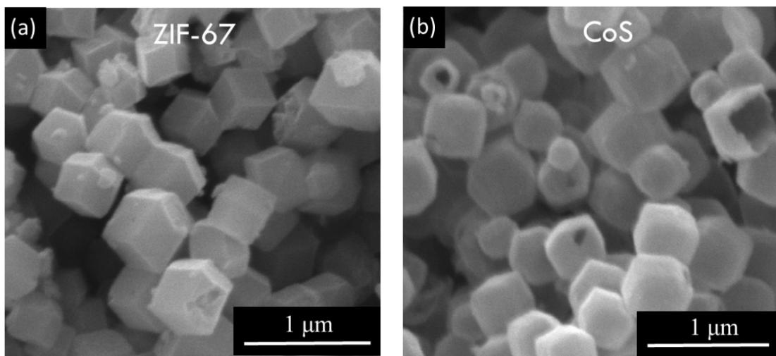
**Figure S5** FE-SEM images of (a) ZIF-67 nanoparticles, and (b) CoS nanocages.
