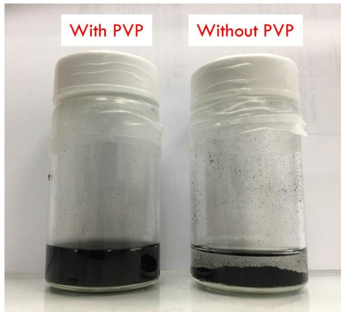
**Figure S1** CNT dispersed in methanol with (left) and without (right) PVP.
