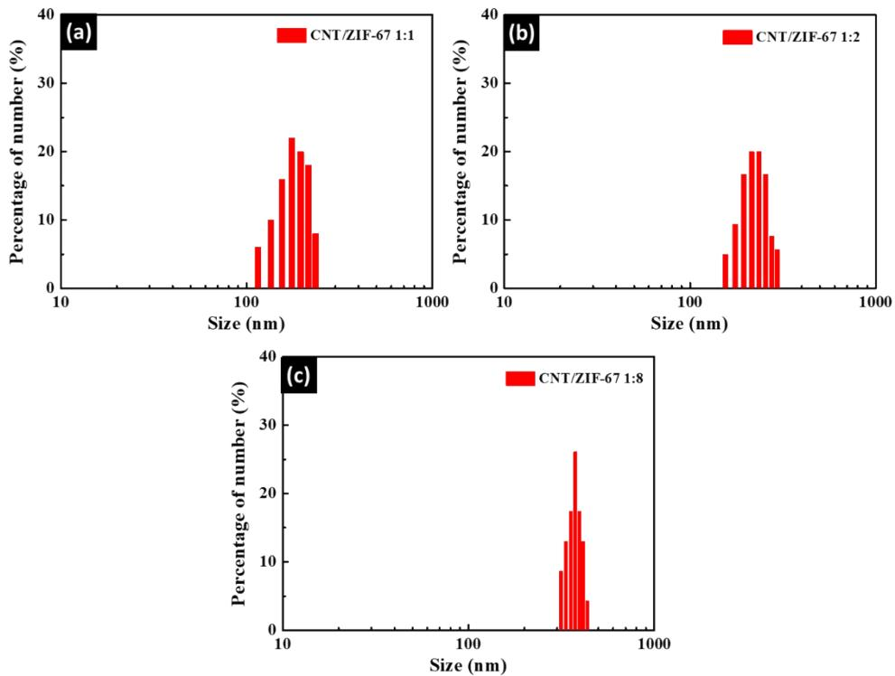
**Figure S3** Particle size distributions of (a) CNT/ZIF-67 1:1, (b) CNT/ZIF-67 1:2, and (c) CNT/ZIF-67 1:8.
