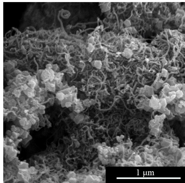
**Figure S4** FE-SEM images of CNT/ZIF-67 composites with unfunctionalized CNTs.
