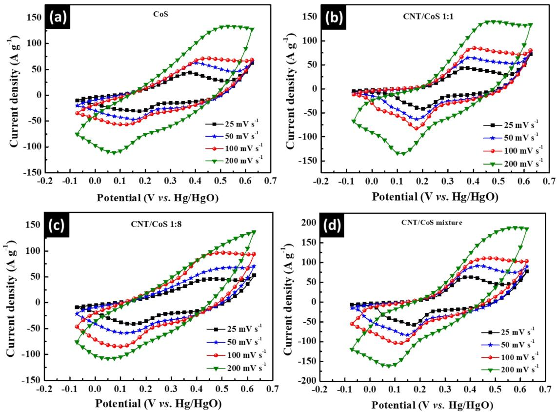
**Figure S9** CVs of (a) CoS nanocage, (b) CNT/CoS 1:1 nanocage, (c) CNT/CoS 1:8 nanocage, and (d) CNT/CoS mixture electrodes at different scan rates.
