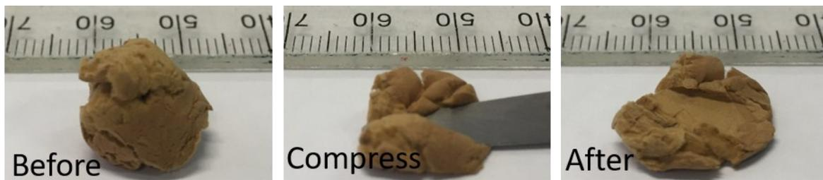
Fig. S2. Photographs of an as lyophilized lignin based sample with no shape recovery functions
