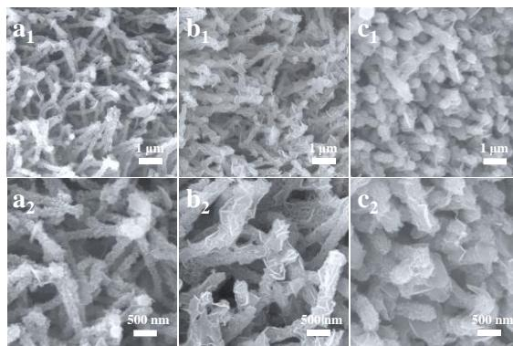
**Figure 11** SEM images of (a) E-CoSe<sub>2</sub>/Ni<sub>0.85</sub>Se-4, (b) E-CoSe<sub>2</sub>/Ni<sub>0.85</sub>Se-8 and (c) E-CoSe<sub>2</sub>/Ni<sub>0.85</sub>Se-12.
