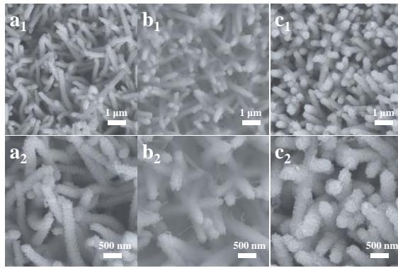
**Figure S10** SEM images of (a) CoSe<sub>2</sub>/Ni<sub>0.85</sub>Se-4, (b) CoSe<sub>2</sub>/Ni<sub>0.85</sub>Se-8 and (c) CoSe<sub>2</sub>/Ni<sub>0.85</sub>Se-12.
