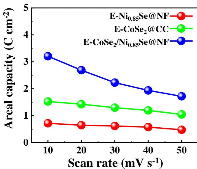
**Figure S6** The calculated areal capacity of obtained electrodes via CV measurements.
