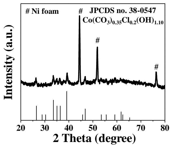
**Figure S2** XRD patterns of Co-precursors on Ni foam.
