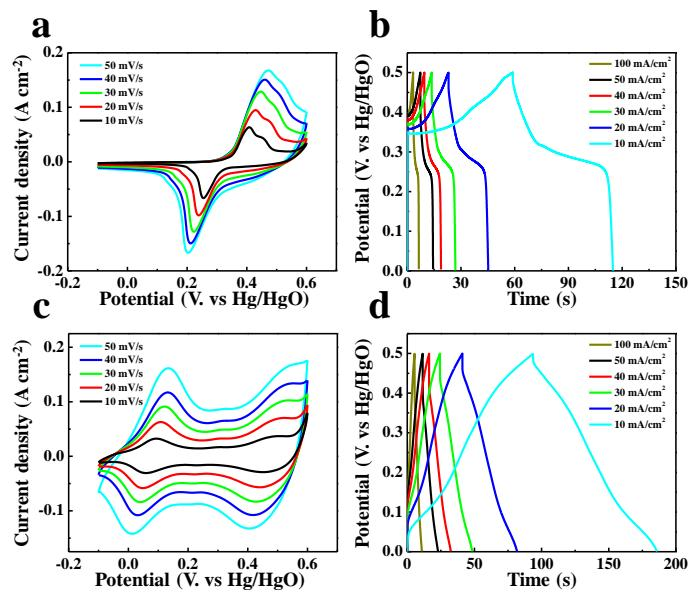
**Figure S5** CV and GCD curves of (a, b) E- $\text{Ni}_{0.85}\text{Se}$ @NF and (c, d) E- $\text{CoSe}_2$ @CC.
