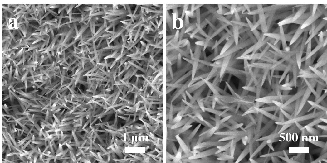
**Figure S1** SEM images of Co-precursors on Ni foam.
