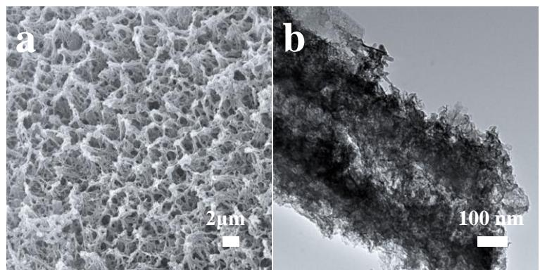
**Figure S8** SEM and TEM images of E-CoSe<sub>2</sub>/Ni<sub>0.85</sub>Se@NF after cycling test.
