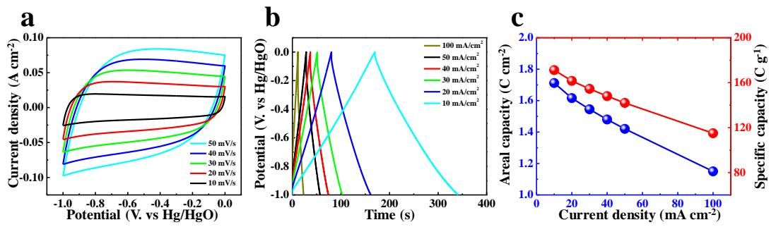
**Figure S9** (a) CV, (b) GCD curves and (c) corresponding calculated capacity of AC.
