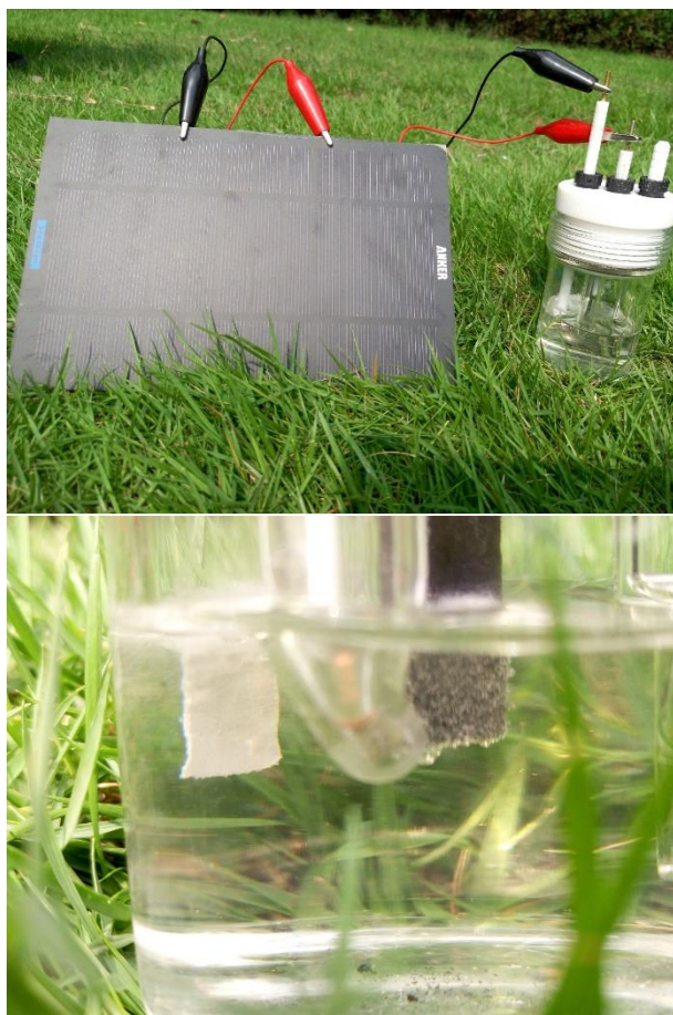
Figure S12. Solar-driven water splitting process using the EG/Co(OH) 2 /ZIF-67 hybrid.
