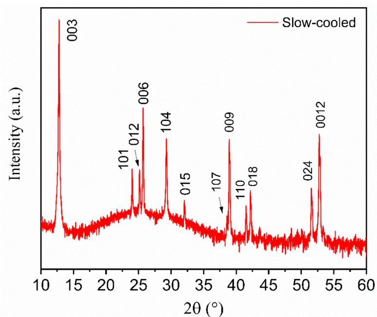
**Fig. S2.** Collected XRD pattern of annealed/slow-cooled thin film of Ag-Bi-I without excess of  $\text{BiI}_3$  ( $180\text{ }^\circ\text{C}$  for 15 min), which was deposited with  $r = 0.6$ .
