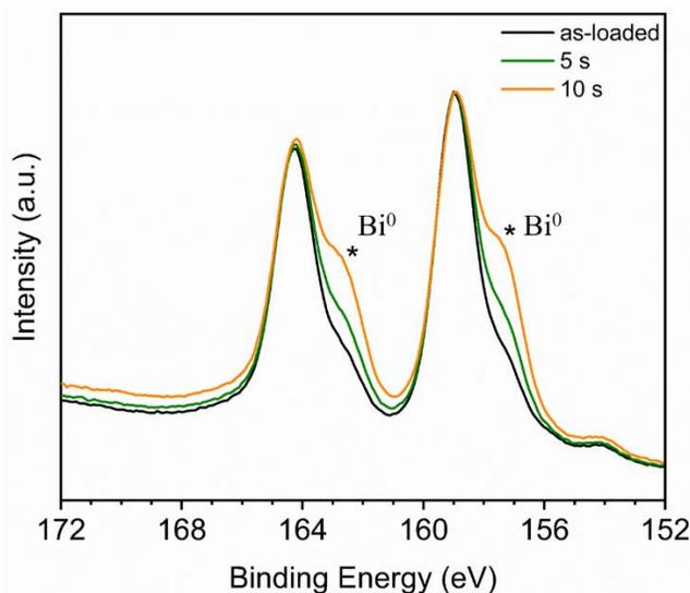
**Fig. S9.** Close-up Mg K $\alpha$  scans of Bi4f peaks for as-loaded, 5 s, and 10 s sputtered thin film of AgBi<sub>4</sub>. Two small shoulders at ~162 eV and 157 eV originate from metallic Bi (Bi<sup>0</sup>).
