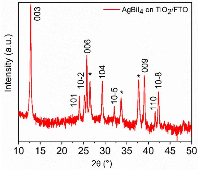
**Fig. S10.** Experimental XRD pattern of annealed/slow-cooled thin film of Ag-Bi-I without excess of BiI<sub>3</sub>, which was deposited with  $r = 0.6$  on TiO<sub>2</sub>/FTO. The labeled peaks with "\*" originate from FTO.
