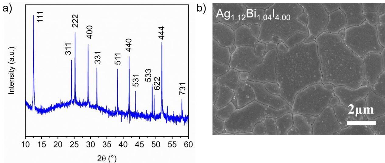
**Fig. S1.** a) Experimental XRD pattern of annealed/quenched thin film of Ag-Bi-I without excess of  $\text{BiI}_3$  ( $180\text{ }^\circ\text{C}$  for 15 min), which was deposited with  $r = 0.6$  and b) SEM image of the thin film with the same noted composition.
