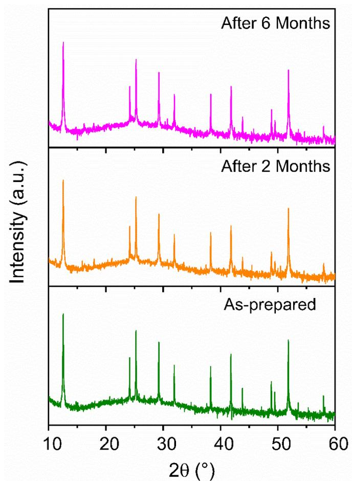
**Fig. S3.** Monitoring N<sub>2</sub> stability of the annealed (without an excess of BiI<sub>3</sub>)  $r = 0.6$  Ag-Bi-I film using XRD, demonstrating the stability of the cubic phase over at least 6 months.
