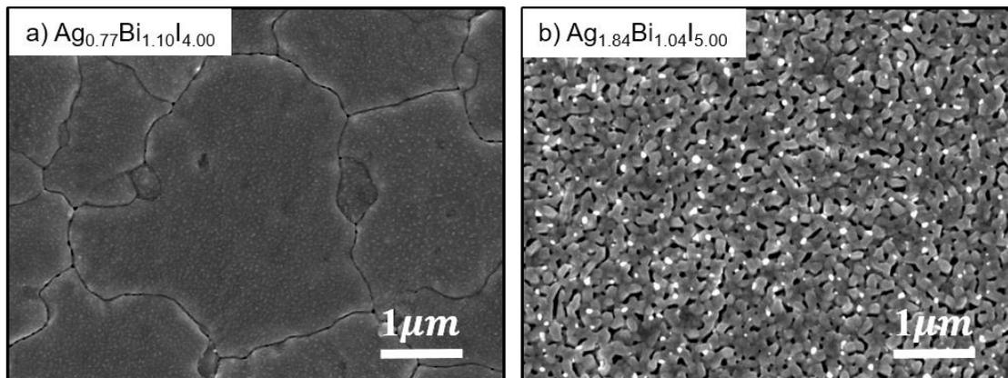
**Fig. S5.** SEM images of the annealed films from the TD XRD process with the associated compositions obtained from SEM/EDX; a) annealed film of  $r = 0.6$  in  $N_2$  (25°-180 °C, 180 °C for 1 h and cooled to 25 °C), b) annealed film of  $r = 0.8$  in  $N_2$  (25°-180 °C, 180 °C for 1 h and cooled to 25 °C).
