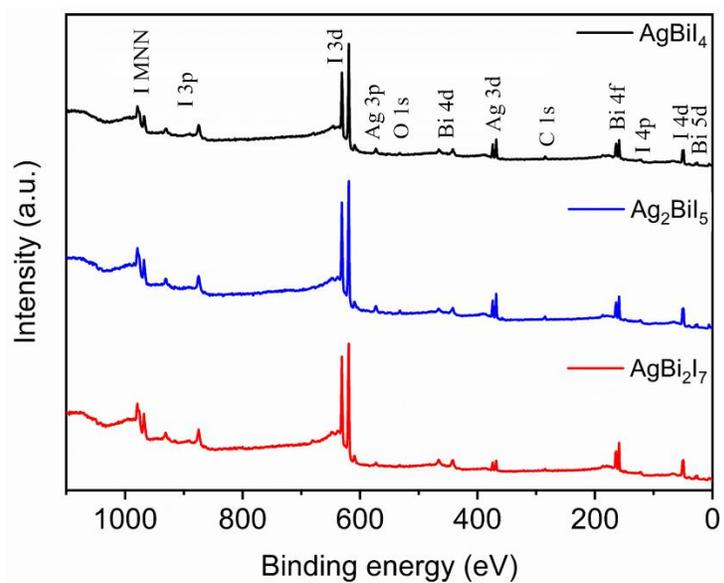
**Fig. S7.** XPS Al K $\alpha$  survey scans of the as-loaded films of annealed  $r = 0.6$  ( $\text{AgBi}_2\text{I}_7$ ) and  $r = 0.8$  ( $\text{Ag}_2\text{BiI}_5$ ) at 180 °C under  $\text{BiI}_3$  vapor and  $r = 0.6$  ( $\text{AgBiI}_4$ ) at 180 °C under  $\text{N}_2$ .
