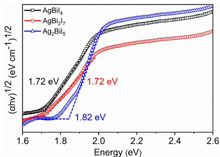
Fig. S6. Tauc plots showing indirect band gaps for  $\text{AgBi}_2\text{I}_7$  (red),  $\text{AgBiI}_4$  (black), and  $\text{Ag}_2\text{BiI}_5$  (blue) films.
