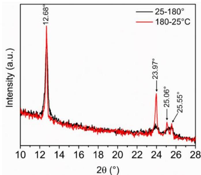
**Fig. S4.** Experimental XRD patterns of as-deposited thin film of Ag-Bi-I (black) with  $r = 0.8$  at 25 °C and the annealed film from the TD XRD process (red) after cooling to 25 °C. Diffraction peaks at 12.68°, 23.97°, 25.06°, and 25.55° are assigned to 003, 101, 012, and 006 of rhombohedral Ag-Bi-I.
