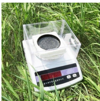
Fig. S10 Optical image of the portable balance that was used to measure the mass loss of water in the BCP 7 -coated petri dish under natural sunlight irradiation.
