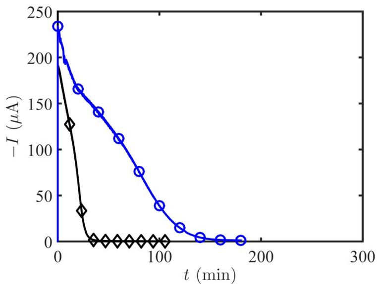
**Figure S2.** Evolution of current ( $I$ ) versus time ( $t$ ), obtained from the chronoamperometry experiments with the same operating conditions as **Figure 1** for an inhibitor-free system (black) and in the presence of 10  $\mu\text{L}$  of pure azidoethyl phosphonate (blue). Despite using a large amount of pure linear phosphonated species, the scaling takes place in less than 2 h, which necessitates the development of more efficient macromolecules.
