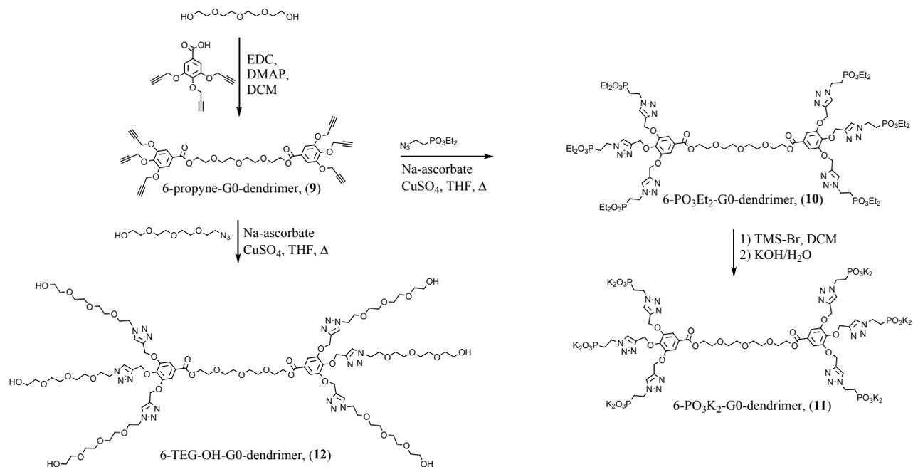
**Scheme 2.** Synthesis of TEG-based dendrimers of generation 0, and the synthesis of 6-TEG-OH-G<sub>0</sub>-dendrimer (12).<sup>1</sup>
