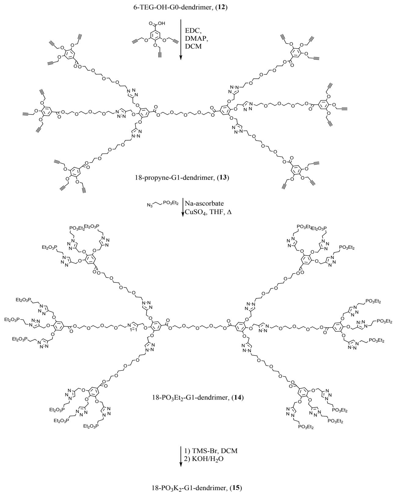
**Scheme 3.** Synthesis of TEG dendrimers: 6-TEG-OH-G1 and 18-PO<sub>3</sub>K<sub>2</sub>-G1.<sup>1</sup>
