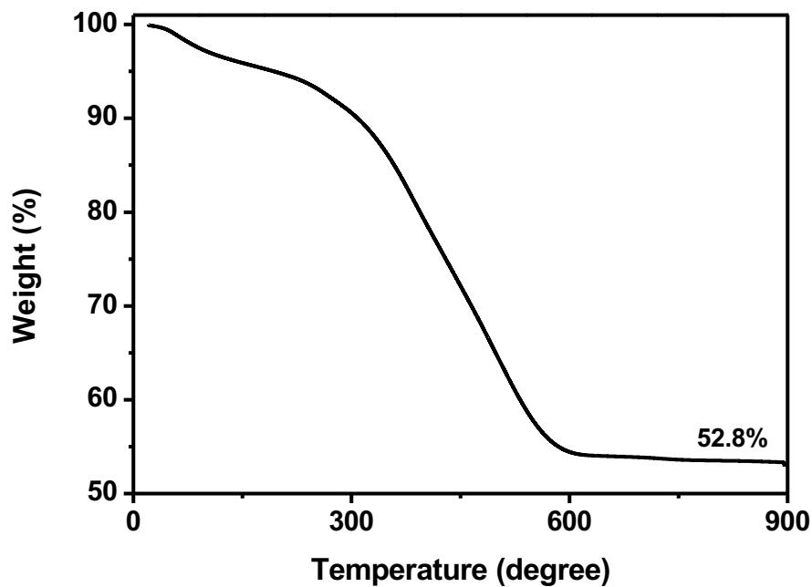
**Fig. S9** TGA profile of  $\text{Ni}_x\text{B}/\text{f-MWCNT}$ .
