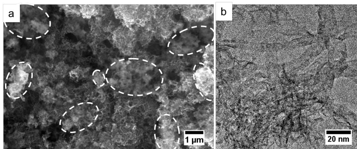
**Fig. S12** (a) SEM and (b) TEM images of the physical mixture  $\text{Ni}_x\text{B}$  and f-MWCNT ( $\text{Ni}_x\text{B}+\text{f-MWCNT}$ ). The areas circled by dashed lines show aggregated  $\text{Ni}_x\text{B}$  particles.
