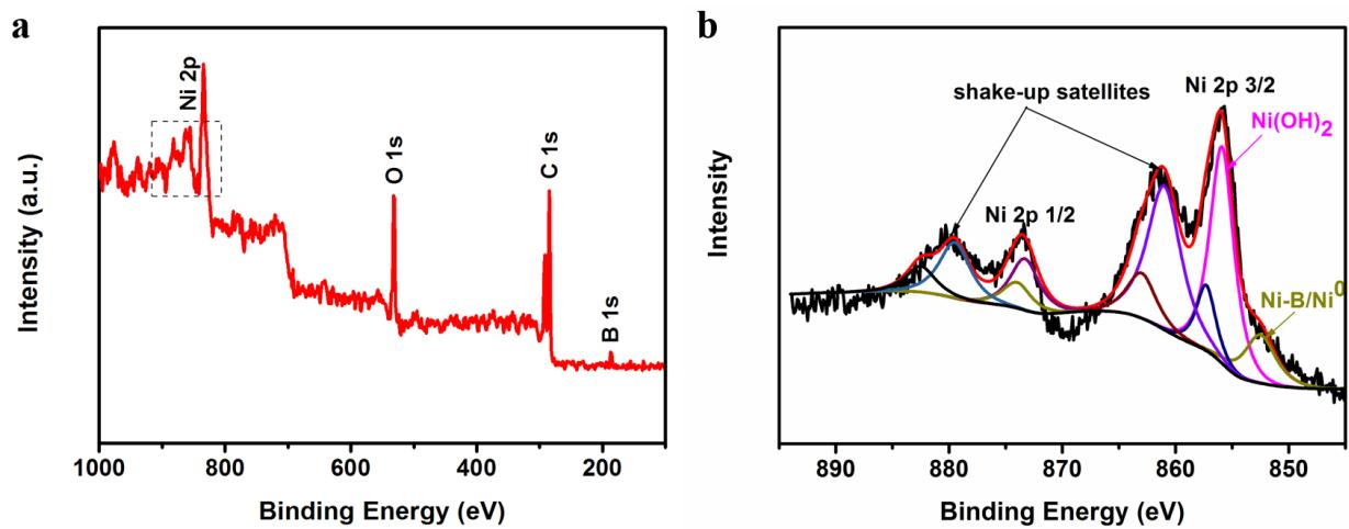
**Fig. S19** (a) XPS survey spectrum of  $\text{Ni}_x\text{B}/\text{f-MWCNT}$  after the 100-hour HER test in  $\text{H}_2$ -saturated 1 M KOH electrolyte under the current density of  $20 \text{ mA cm}^{-2}$ , and (b) the corresponding core-level XPS spectra near the region of Ni2p.
