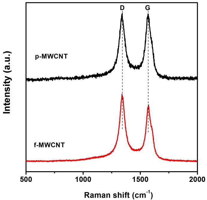
**Fig. S1** Raman spectra of commercial multi-walled carbon nanotubes (MWCNTs) at pristine and chemically functionalized forms: p-MWCNTs and f-MWCNTs. (Note that pristine MWCNTs were not subjected to chemical cleaning and tested in their as-received form.)
