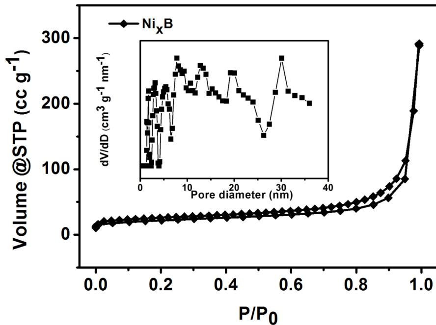
**Fig. S8** Nitrogen adsorption-desorption isotherms of  $\text{Ni}_x\text{B}$ . The inset shows the pore size distribution of  $\text{Ni}_x\text{B}$ .
