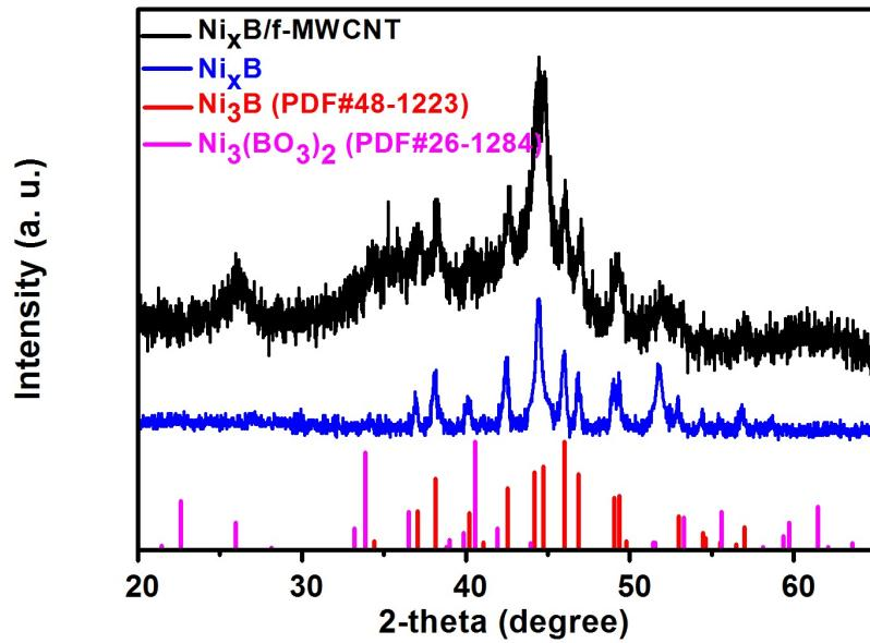
**Fig. S6** XRD patterns of  $\text{Ni}_x\text{B}/\text{f-MWCNT}$  and  $\text{Ni}_x\text{B}$ . The reference XRD peaks of  $\text{Ni}_3\text{B}$  (red vertical lines, JCPDS No. 48-1223) and  $\text{Ni}_3(\text{BO}_3)_2$  (pink vertical lines, JCPDS No. 26-1284).
