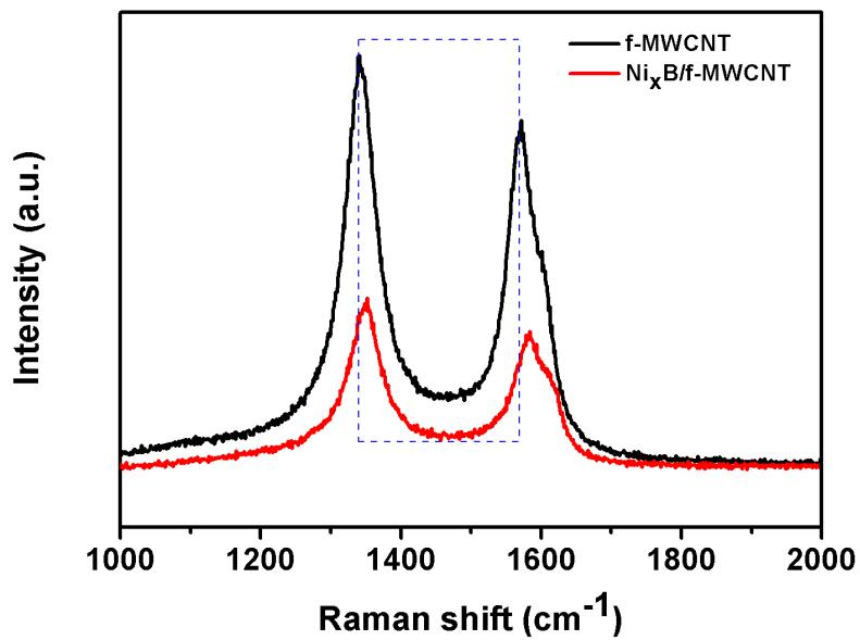
**Fig. S11** Raman spectra of  $\text{Ni}_x\text{B}/\text{f-MWCNT}$  and f-MWCNT.
