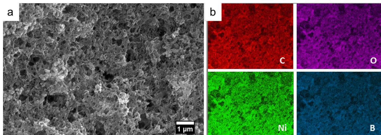
**Fig. S18** Characterization of  $\text{Ni}_x\text{B}/\text{f-MWCNT}$  after the 100-hour HER test in 1 M KOH electrolyte under the current density of 20  $\text{mA cm}^{-2}$ . (a) SEM image and (b) the corresponding EDX elemental mappings of C, O, Ni, and B.
