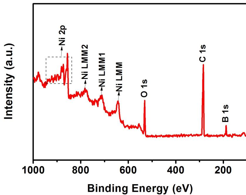
**Fig. S10** XPS survey scan of  $\text{Ni}_x\text{B}/\text{f-MWCNT}$ .
