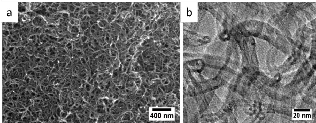
**Fig. S3** (a) SEM and (b) TEM images of f-MWCNTs.
