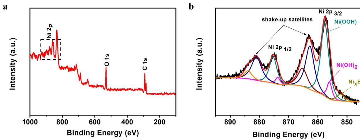
**Fig. S15** (a) XPS survey spectrum of  $\text{Ni}_x\text{B}/\text{f-MWCNT}$  after the 100-hour OER test in 1 M KOH electrolyte under the current density of  $20 \text{ mA cm}^{-2}$ , and (b) the corresponding core-level XPS spectra near the region of Ni2p.
