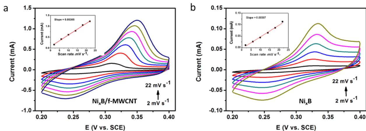
**Fig. S17** CV curves of (a)  $\text{Ni}_x\text{B}/\text{f-MWCNT}$  and (b)  $\text{Ni}_x\text{B}$  at the different scan rates from 2 to 22  $\text{mV s}^{-1}$  in 1 M KOH electrolyte. The inset figures show the corresponding plots of the oxidation peak current *vs.* the scan rate extracted from (a) and (b), respectively.
