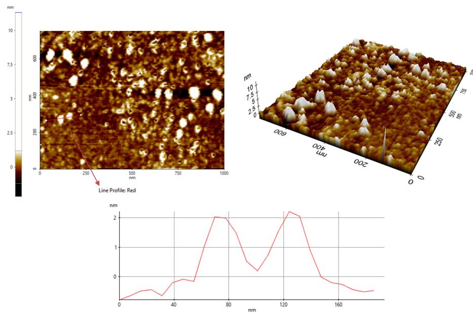
**Figure S7** AFM images of  $\text{Ni}_x\text{B}/\text{f-MWCNT}$  in 2D and 3D projection, recorded in the tapping mode, and the corresponding height profile.
