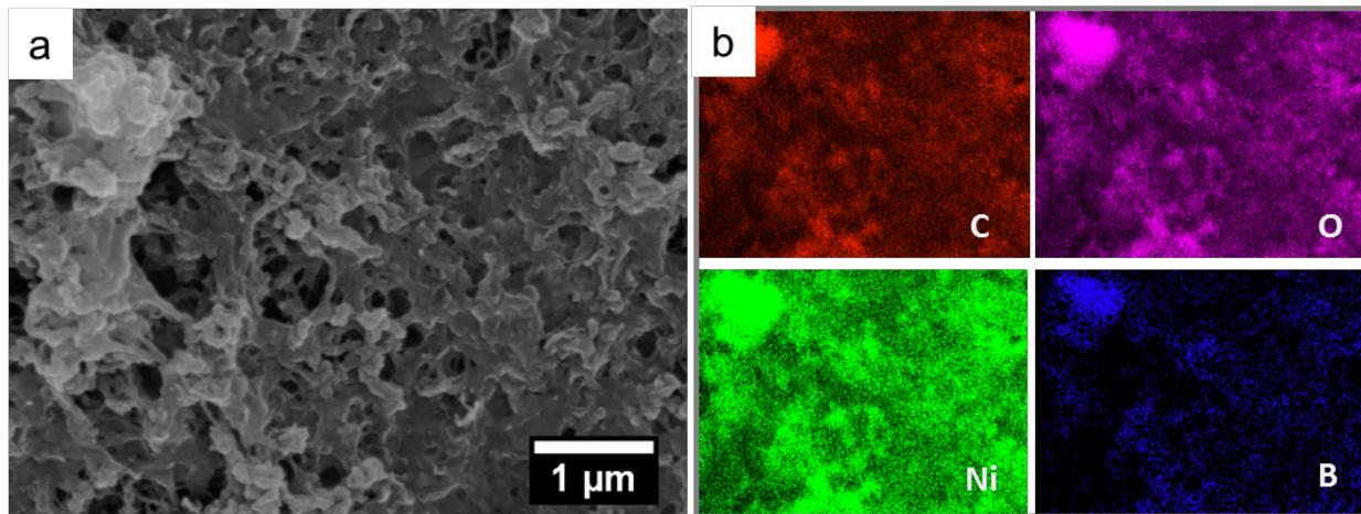
**Fig. S14** Characterization of  $\text{Ni}_x\text{B}/\text{f-MWCNT}$  after the 100-hour OER test in 1 M KOH electrolyte under the current density of  $20 \text{ mA cm}^{-2}$ . (a) SEM image and (b) the corresponding EDX elemental mappings of C, O, Ni, and B.
