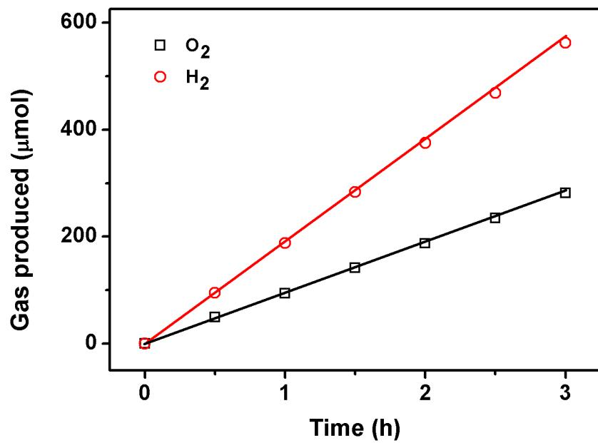
**Fig. S20.** The amount of gas theoretically calculated and experimentally measured vs. time for OER and HER vs. time for Ni<sub>x</sub>B/f-MWCNT.
