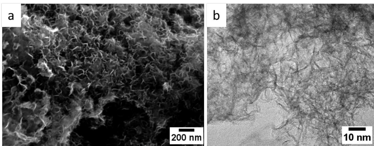
**Fig. S4** (a) SEM and (b) TEM images of Ni<sub>x</sub>B nanosheets.
