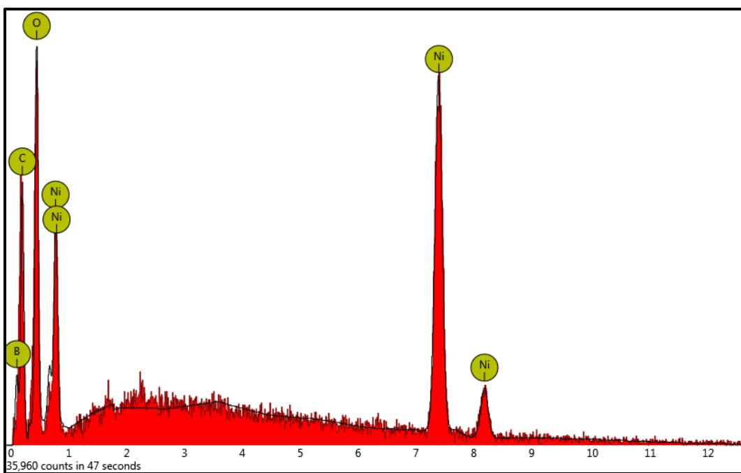
**Fig. S5** EDS spectrum of  $\text{Ni}_x\text{B}/\text{f-MWCNT}$ .
