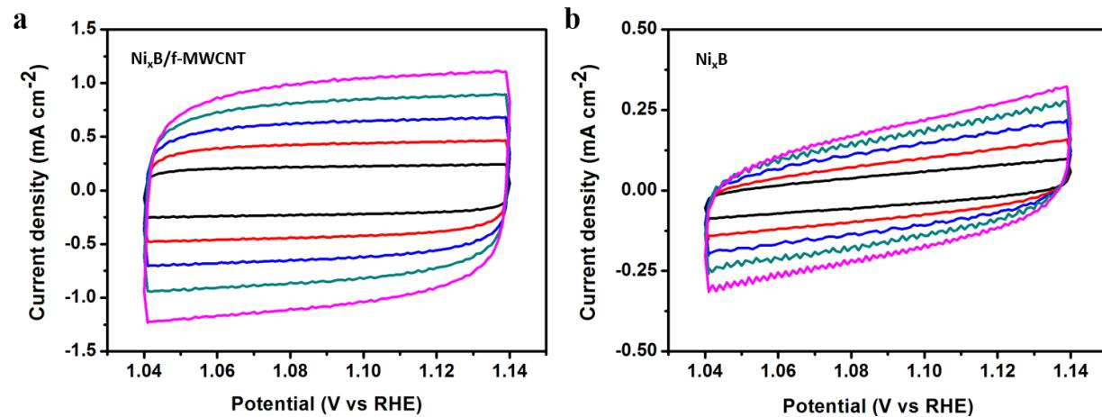
**Fig. S16** Cyclic voltammogram (CV) curves of (a)  $\text{Ni}_x\text{B}/\text{f-MWCNT}$  and (b)  $\text{Ni}_x\text{B}$  recorded in a non-Faradic region in 1 M KOH at different scan rates of 20, 40, 60, 80, and 100 mV s<sup>-1</sup>.
