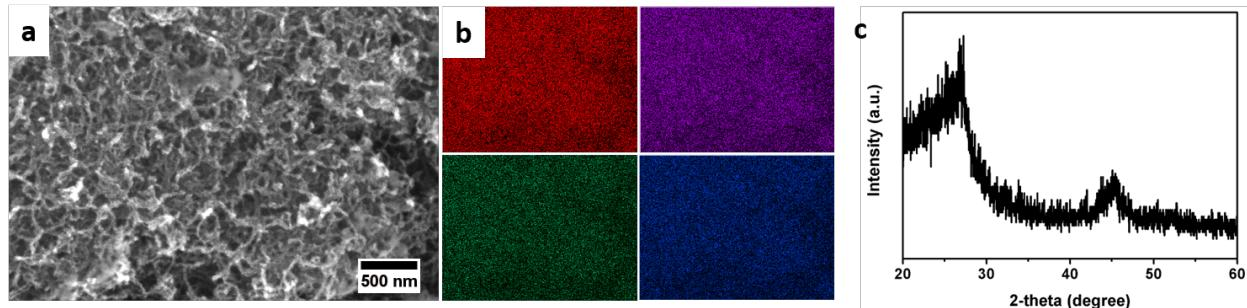
**Fig. S2** Characterization of the morphology and structure properties of NixB/f-MWCNT hybrids before 300 °C calcination. (a) SEM; (b) the corresponding EDX elemental mappings of the whole region of (a); (c) XRD.
