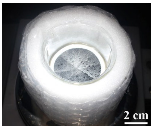
Fig. S11. Optical image of a folded CNT@PEI/MCE membrane with reserved water replenishment via the capillary pumping (some droplet on the surface).
