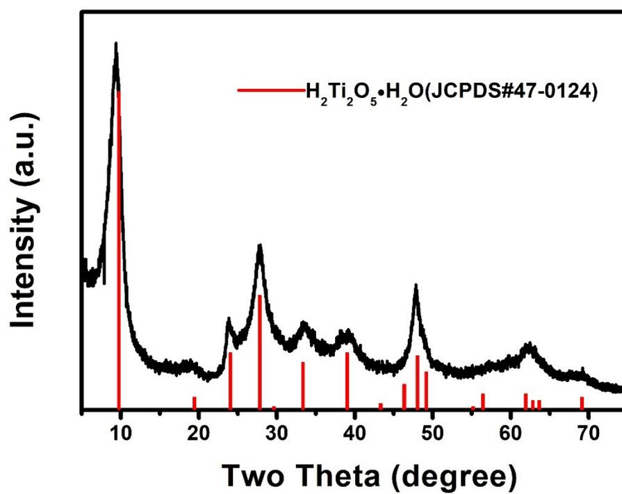
**Fig. S3.** XRD patterns of nanosheets-assembled  $\text{H}_2\text{Ti}_2\text{O}_5 \cdot \text{H}_2\text{O}$  tubes.
