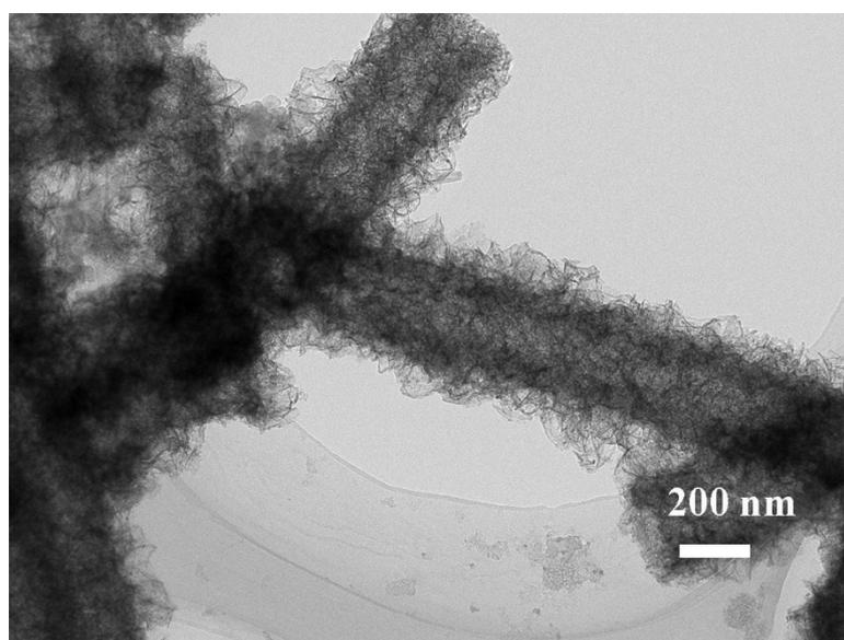
**Fig. S4.** TEM images of the nanosheet-assembled  $\text{TiO}_2$  tubes (400 °C) after 1000 cycles.
