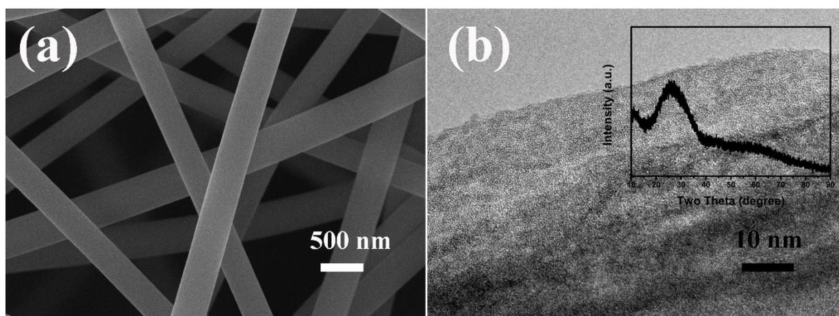
**Fig. S1.** (a) SEM and (b) HR-TEM images of the amorphous  $\text{TiO}_2/\text{SiO}_2$  composite fibers. Inset in (b) is the XRD pattern of amorphous  $\text{TiO}_2/\text{SiO}_2$  composite fibers.
