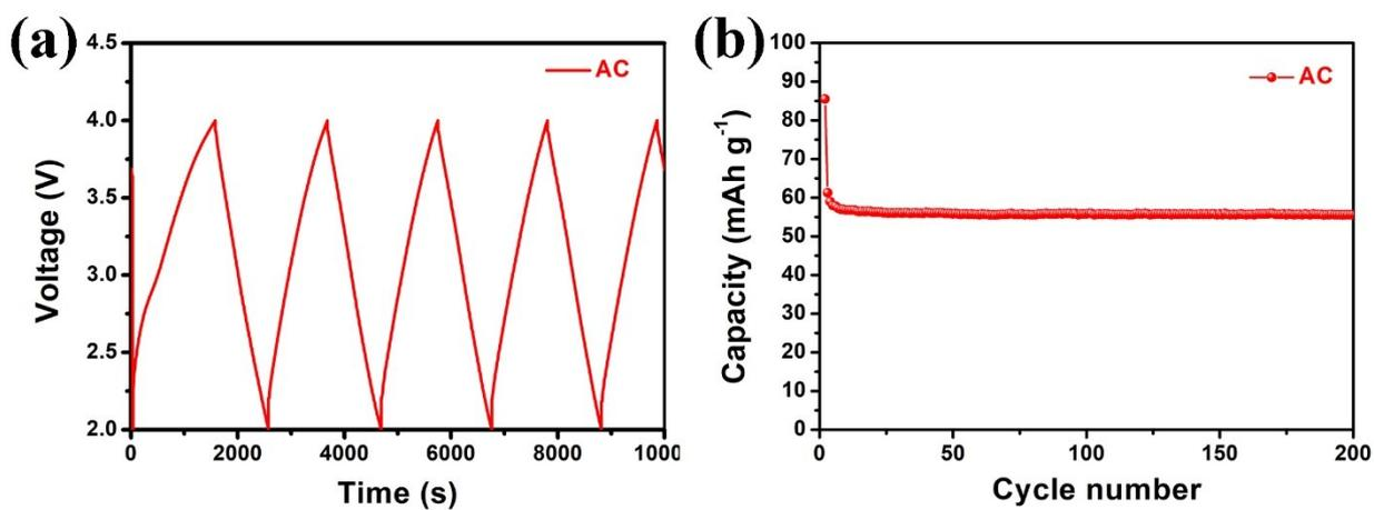
**Fig. S6.** (a) Galvanostatic charge-discharge curve and (b) cycling performance of the AC electrode at  $1.0 \text{ A g}^{-1}$  between 2.0 and 4.0 V.
