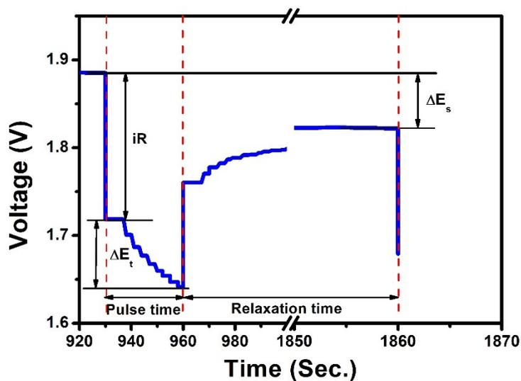
**Fig. S5.** E vs. t curves of TONS-HT-400 electrode for a single GITT during discharge process.
