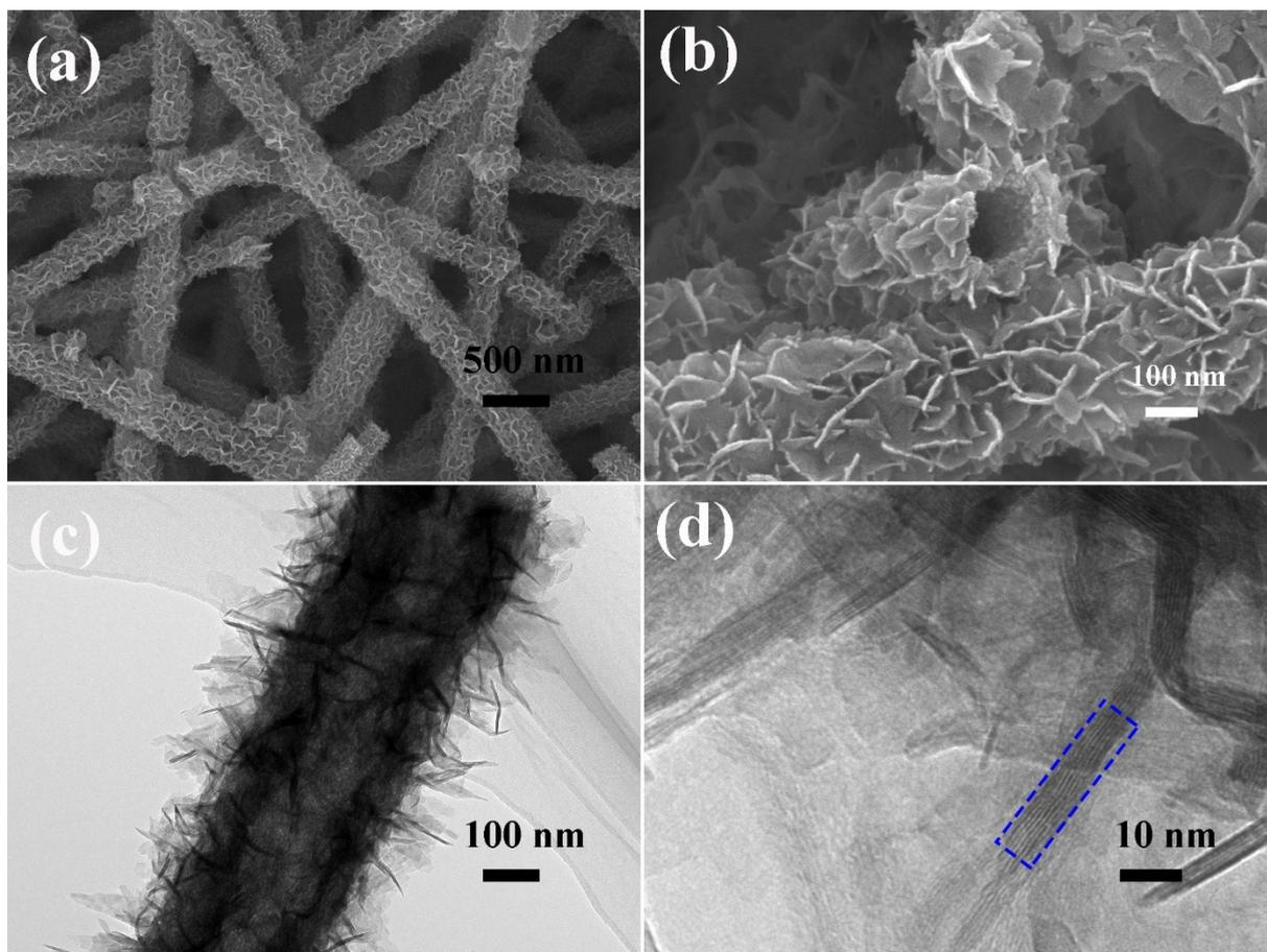
**Fig. S2.** (a, b) SEM, (c) TEM and (d) HR-TEM images of the layered hydrate titanate.
