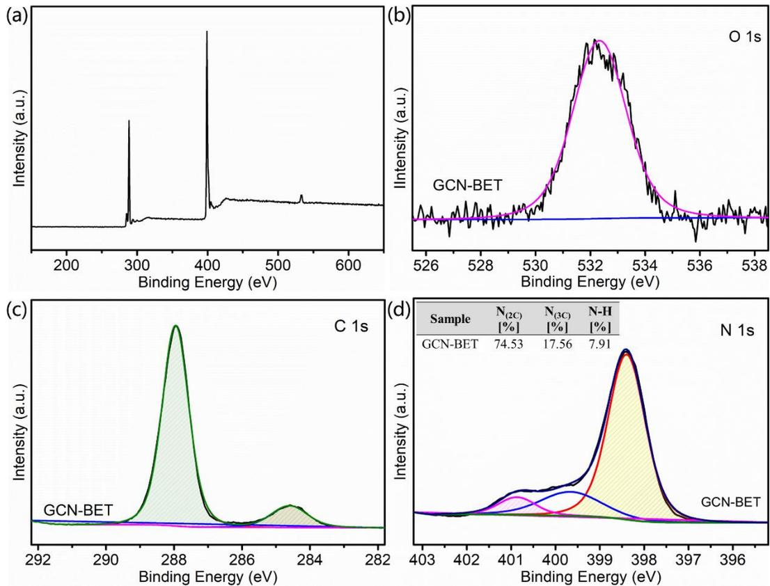
**Figure S7.** (a) XPS survey spectra; high resolution XPS (b) O 1s, (c) C 1s, (d) N 1s spectra of GCN-BET sample.
