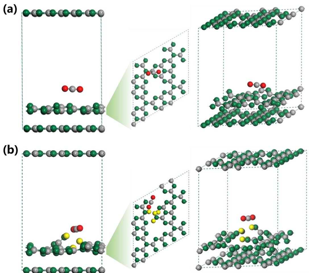
**Figure S5.** Optimized geometry structure for CO<sub>2</sub> adsorption on (a) GCN surface and (b) carbon-vacancy modified GCN surface, where the green, gray, yellow and red color spheres represent C, N, H and O atoms, respectively.
