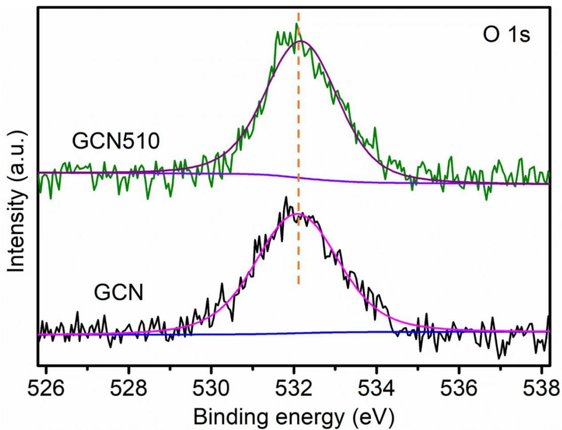
**Figure S1.** High resolution XPS O 1s spectra of GCN and GCN510 samples.
