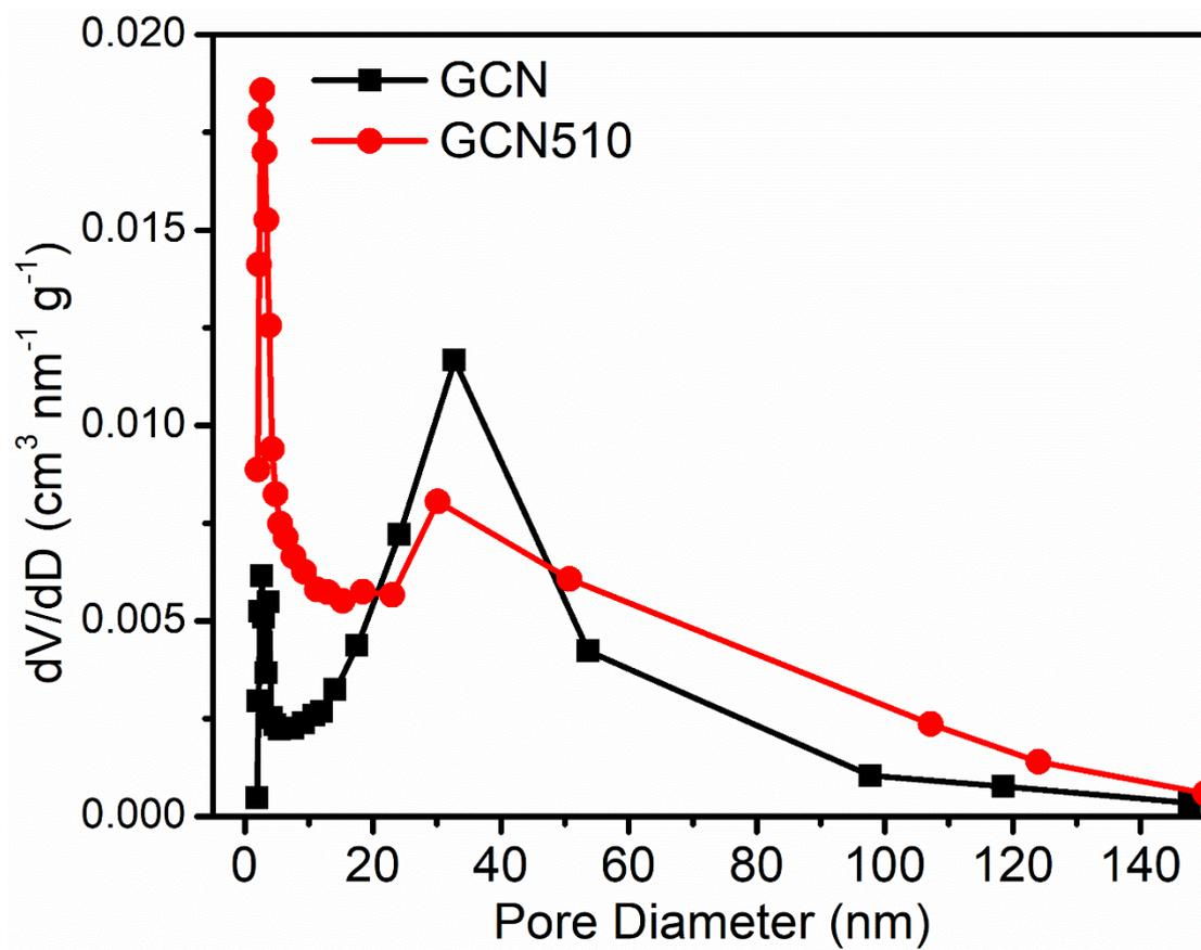
**Figure S2-2.** The pore-size distributions calculated from the desorption branch of GCN and GCN510 samples.
