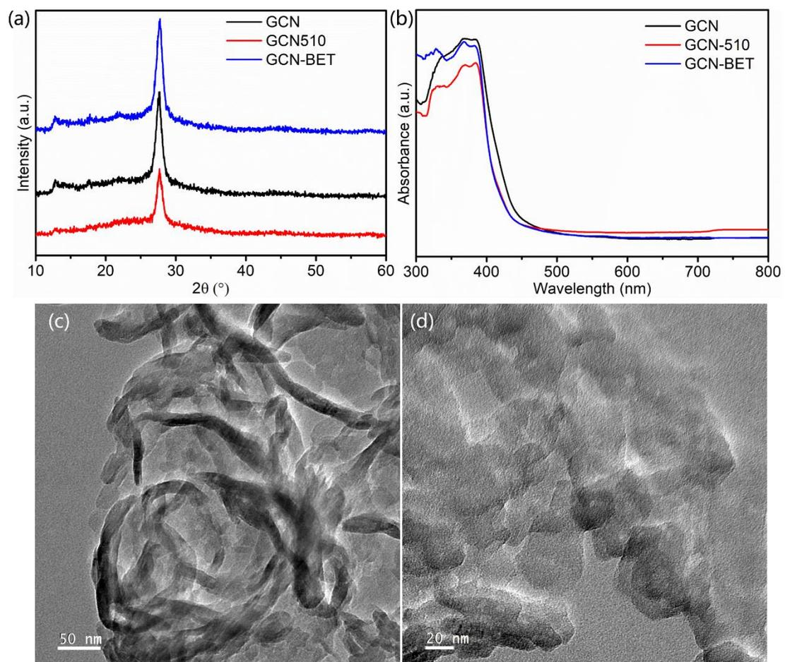
**Figure S6.** (a) The XRD pattern, (b) UV-Vis diffuse reflectance spectra of GCN-BET compared with GCN and GCN510 samples, (c) and (d) TEM images of GCN-BET
