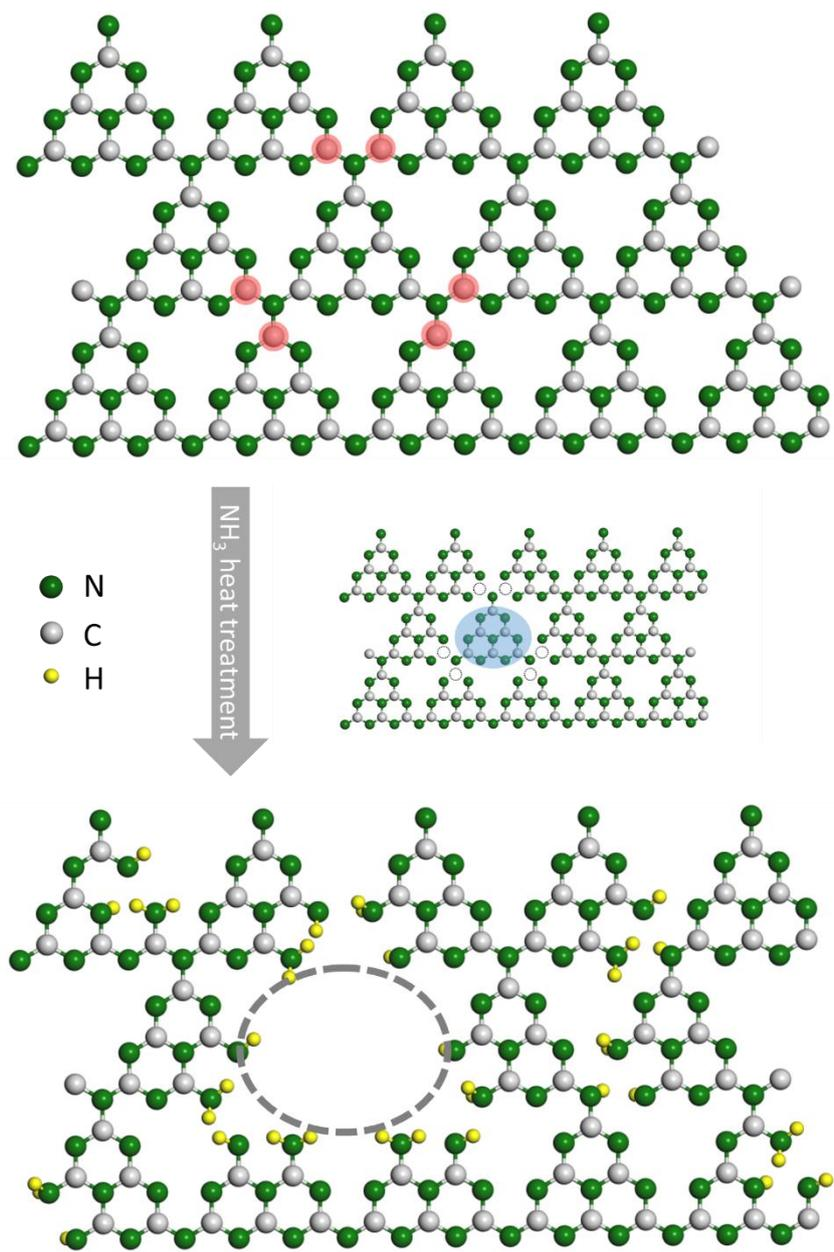
**Figure S4.** Schematic illustration of an example of nanometer-scale holes formation in GCN510.
