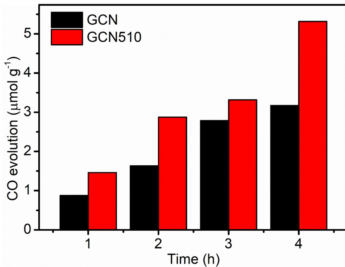
**Figure S3.** CO evolution on GCN and GCN510 photocatalysts in 4 h light ( $\lambda \geq 420$  nm) illumination.
