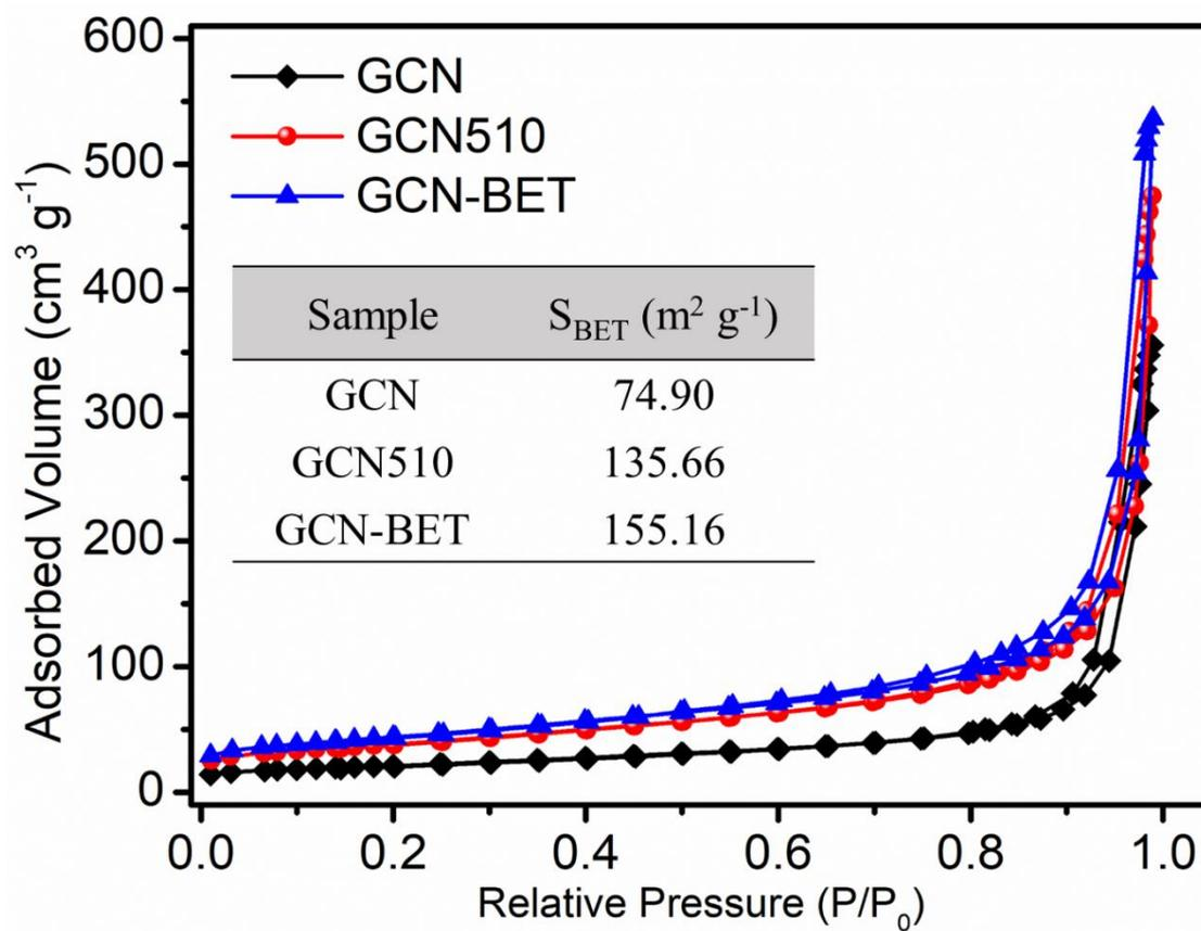
**Figure S2-1.**  $\text{N}_2$  adsorption/desorption isotherms of GCN, GCN510 and GCN-BET samples.
