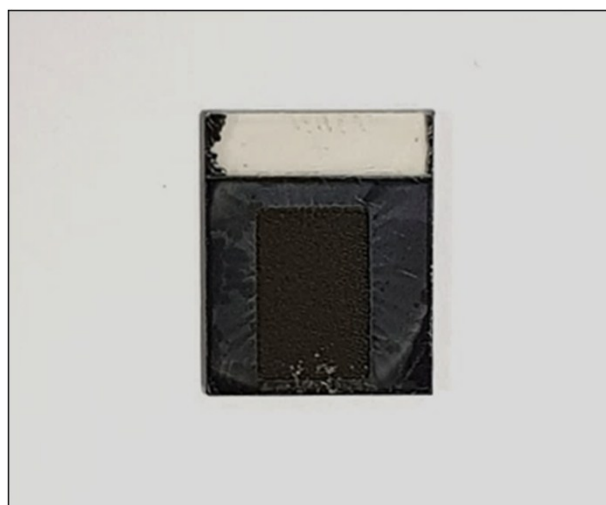
Figure S10. A digital photograph of our carbon-based PSC with PEAI treatment.
