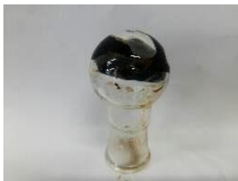
Fig. S3 Photograph of the crosslinking of QAPVP and BHMC in a DMSO solution
