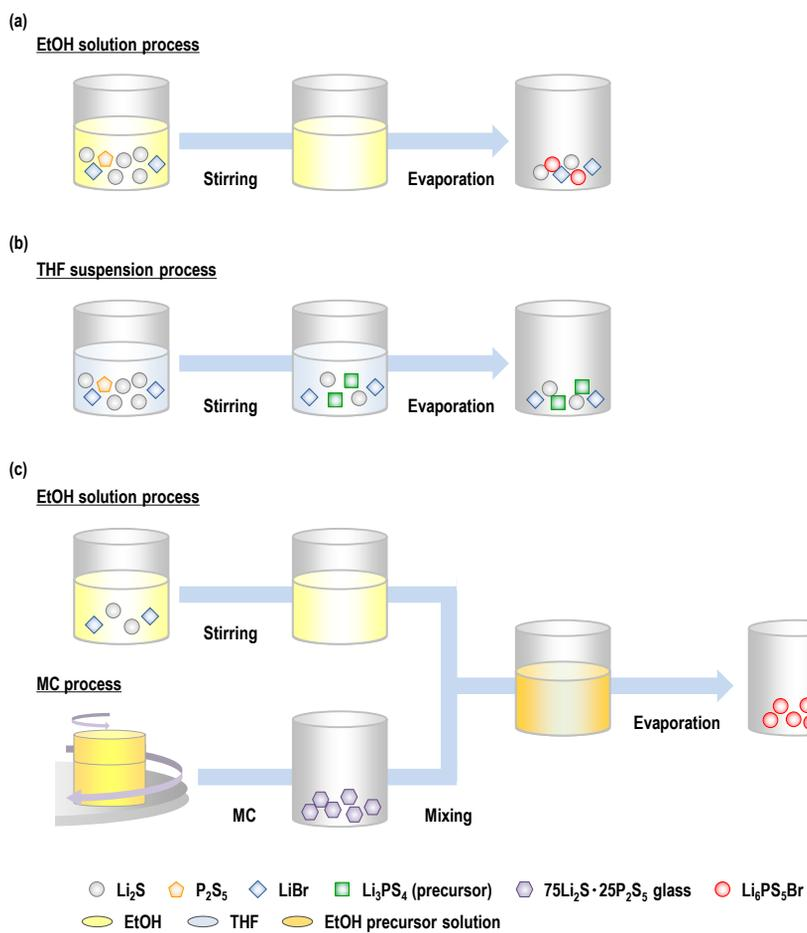
Figure S1. Schematic illustrations of the LP techniques for synthesis of  $\text{Li}_6\text{PS}_5\text{Br}$  with (a) EtOH only, (b) THF only, and (c) *via* EtOH solution and MC processes.
