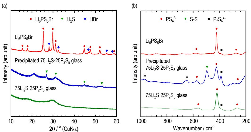
Figure S5. (a) XRD patterns and (b) Raman spectra of Li<sub>6</sub>PS<sub>5</sub>Br synthesized from Li<sub>2</sub>S, LiBr, and 75Li<sub>2</sub>S·25P<sub>2</sub>S<sub>5</sub> glass with EtOH solvent, 75Li<sub>2</sub>S·25P<sub>2</sub>S<sub>5</sub> glass precipitated from EtOH solvent, and 75Li<sub>2</sub>S·25P<sub>2</sub>S<sub>5</sub> glass. Asterisks indicate unknown peaks.
