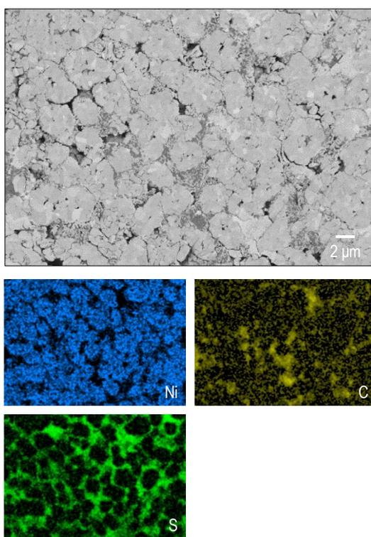
Figure S9. Cross-sectional FE-SEM image and EDX maps of nickel, carbon, and sulfur for the infiltrated NMC electrode.
