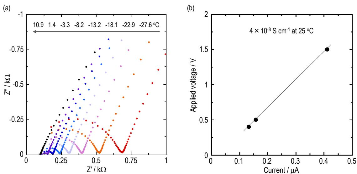
Figure S6. (a) Nyquist plots of LP-550 sintered body at temperatures between  $-27.6\text{ }^{\circ}\text{C}$  and  $10.9\text{ }^{\circ}\text{C}$ . A resistance of more than  $100\ \Omega$  was used for analyzing the temperature-dependence of the conductivity. (b) Relationship between the applied voltage and current, measured by DC polarization technique to determine the electronic conductivity, for the LP-550 green compact pressed at 360 MPa.
