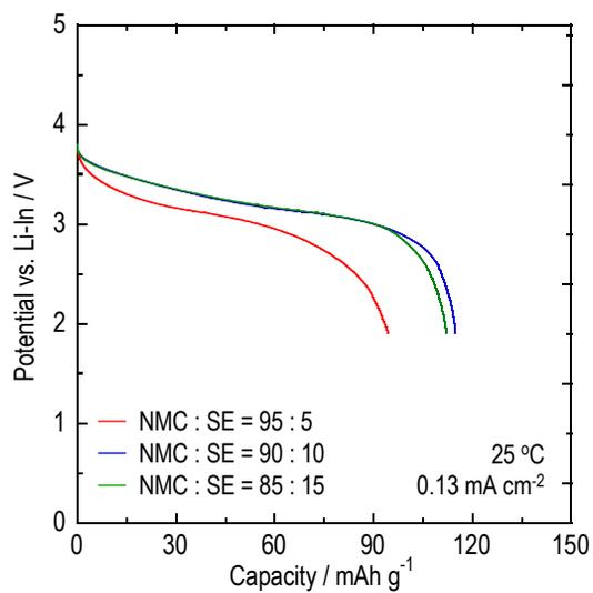
Figure S8. Discharge curves of cells with SE-coated NMC electrodes. The NMC/SE weight ratios were  $x:100-x$  ( $x = 85, 90, 95$ ).
