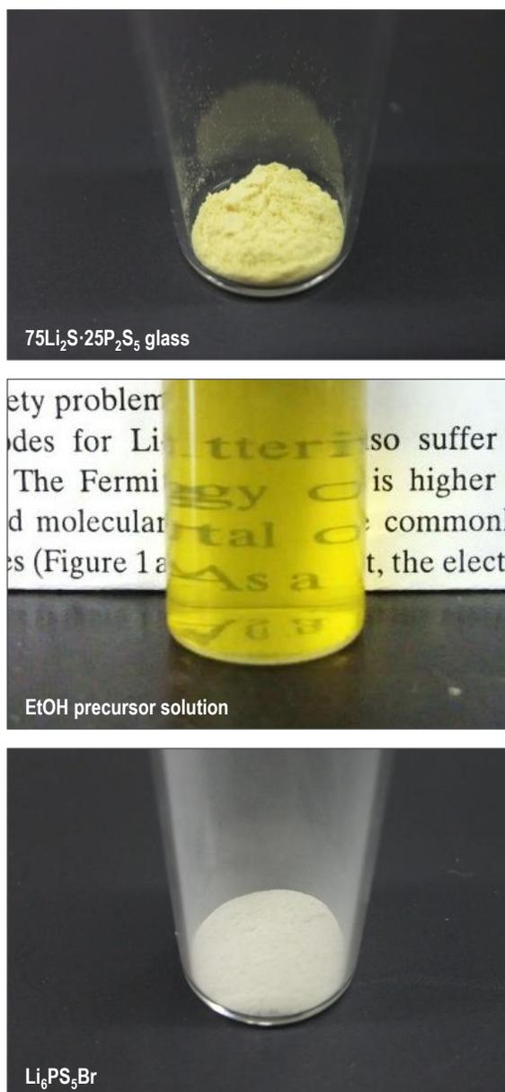
Figure S4. Photographic images of 75Li<sub>2</sub>S·25P<sub>2</sub>S<sub>5</sub> glass powder, EtOH precursor solution, and Li<sub>6</sub>PS<sub>5</sub>Br powder synthesized from Li<sub>2</sub>S, LiBr, and 75Li<sub>2</sub>S·25P<sub>2</sub>S<sub>5</sub> glass with EtOH solvent.
