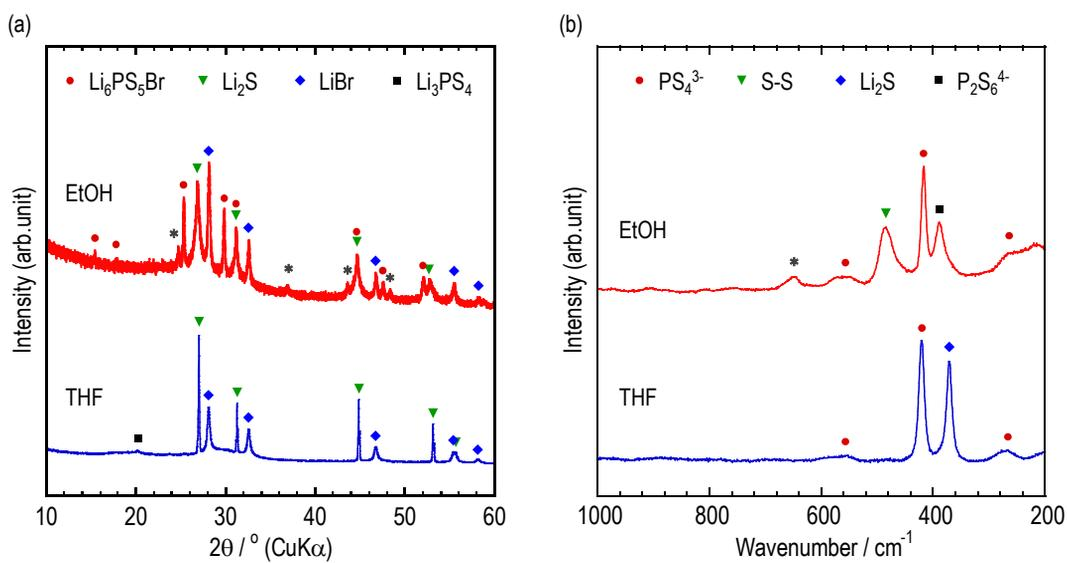
Figure S3. (a) XRD patterns and (b) Raman spectra of the samples prepared with EtOH only and THF only, respectively. Asterisks indicate unknown peaks.
