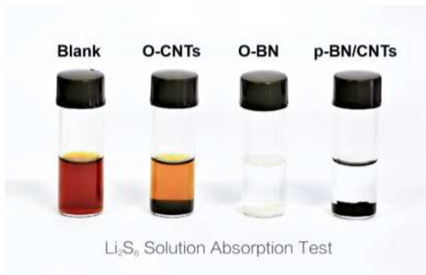
Figure S7. Static adsorption test of O-CNTs, O-BN and p-BN/CNTs with \text{Li}_2\text{S}_6 solution.
