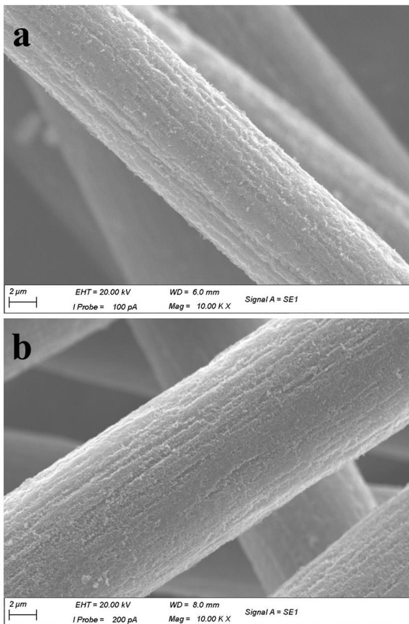
**Fig. S9:** SEM images of (a) NiCoO<sub>2</sub>/GF before charge-discharge cycling; (b) NiCoO<sub>2</sub>/GF after cycling.
