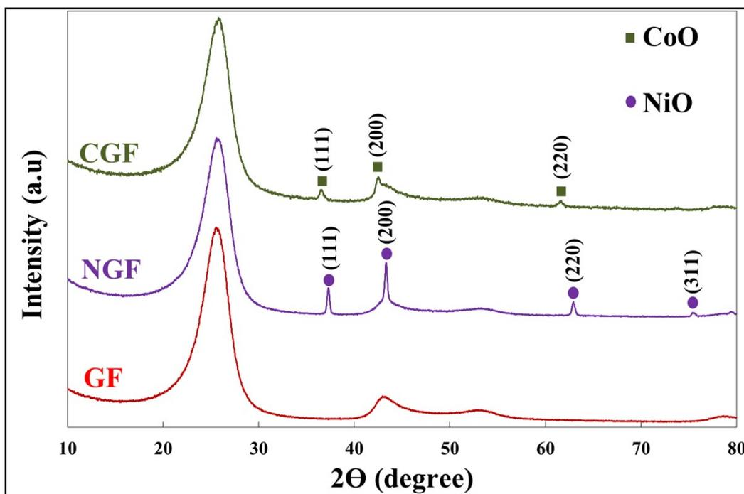
Fig. S1: XRD spectra of GF, NiO/GF and CoO/GF.
