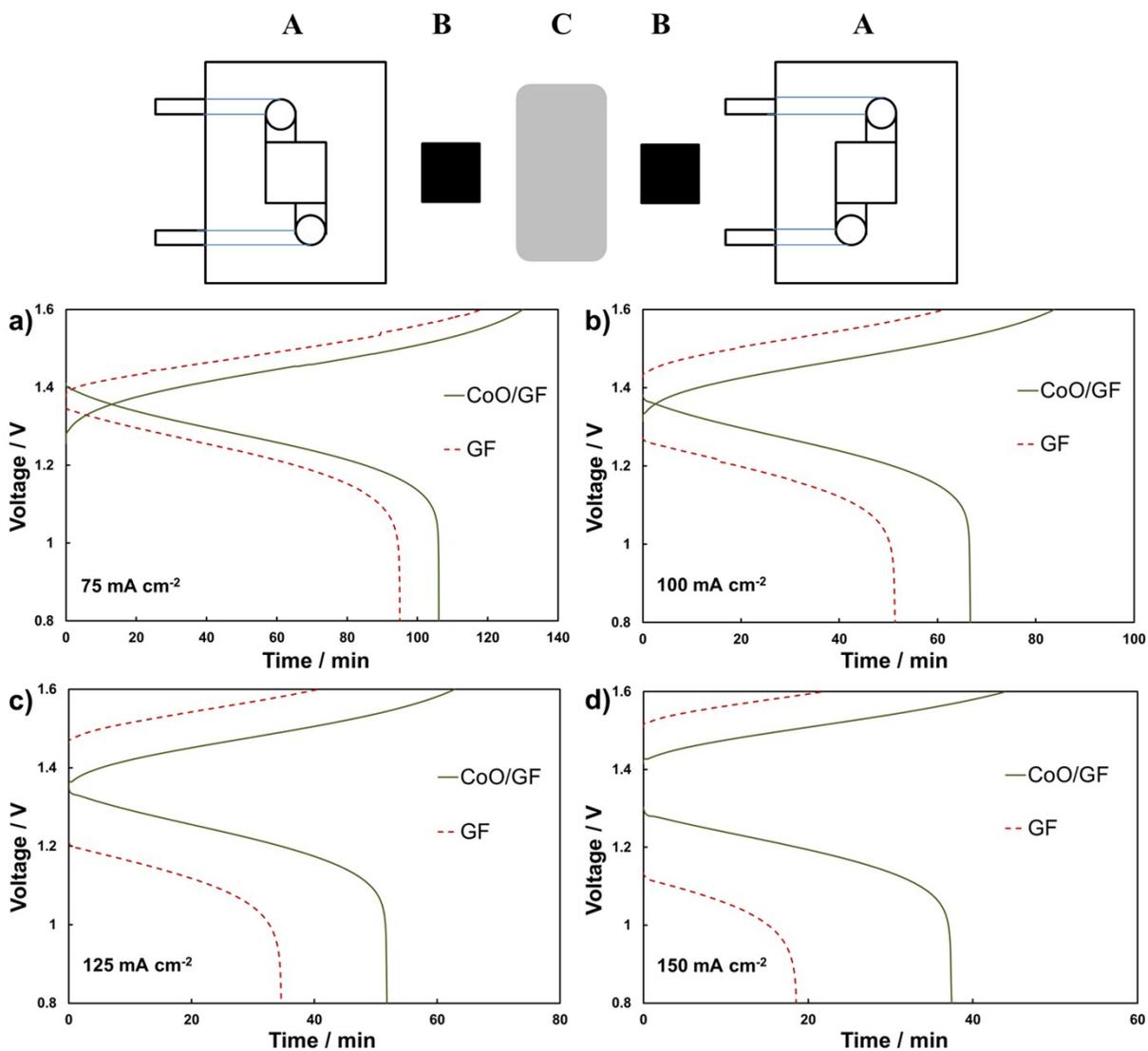
**Fig. S7:** Schematic of the key components of VRFB (A) flow frame plate (B) graphite felt (C) membrane and the cell performance of charge-discharge of the flow cells employing GF and CoO/GF electrodes at a constant current density of (a) 75 mA cm<sup>-2</sup> (b) 100 mA cm<sup>-2</sup> (c) 125 mA cm<sup>-2</sup> (d) 150 mA cm<sup>-2</sup>.
