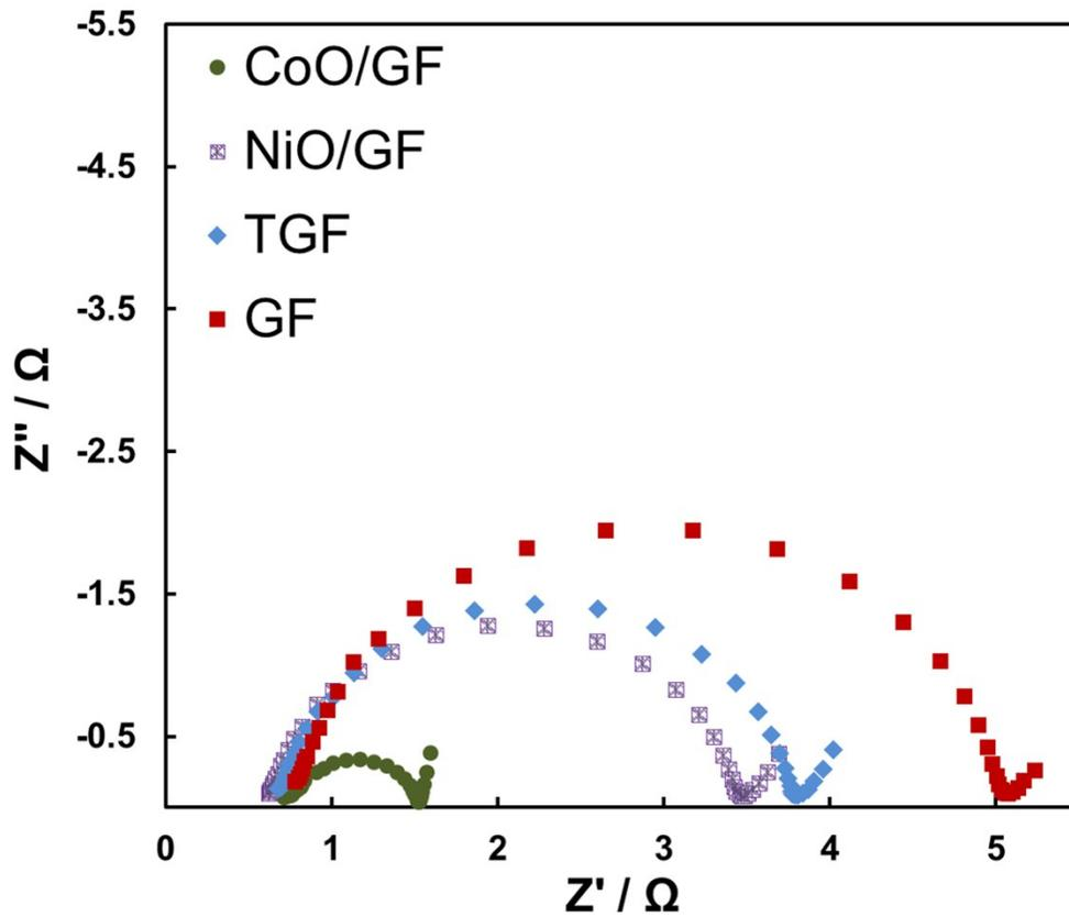
**Fig. S6:** Nyquist plots of GF, TGF, NiO/GF and CoO/GF electrodes in 0.1 M  $\text{VO}_2^+$  / 0.1 M  $\text{VO}_2^+$  in 2 M  $\text{H}_2\text{SO}_4$ .
