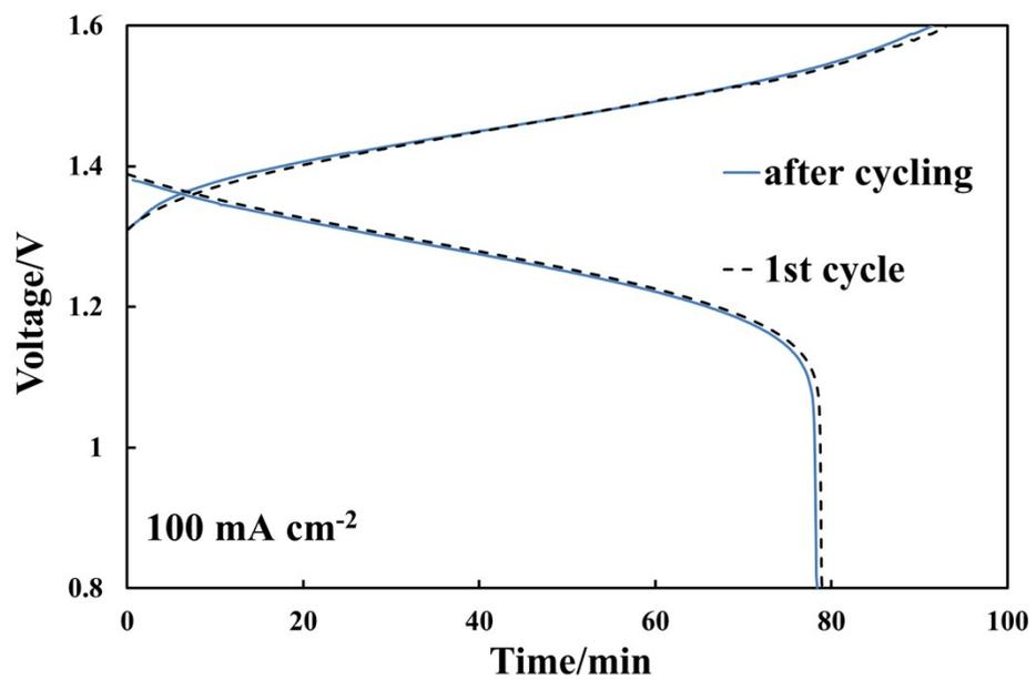
**Fig. S8:** Charge-discharge of the flow cell employing NiCoO<sub>2</sub>/GF electrode. After 50 cycles, the electrolyte was refreshed using newly prepared solutions.
