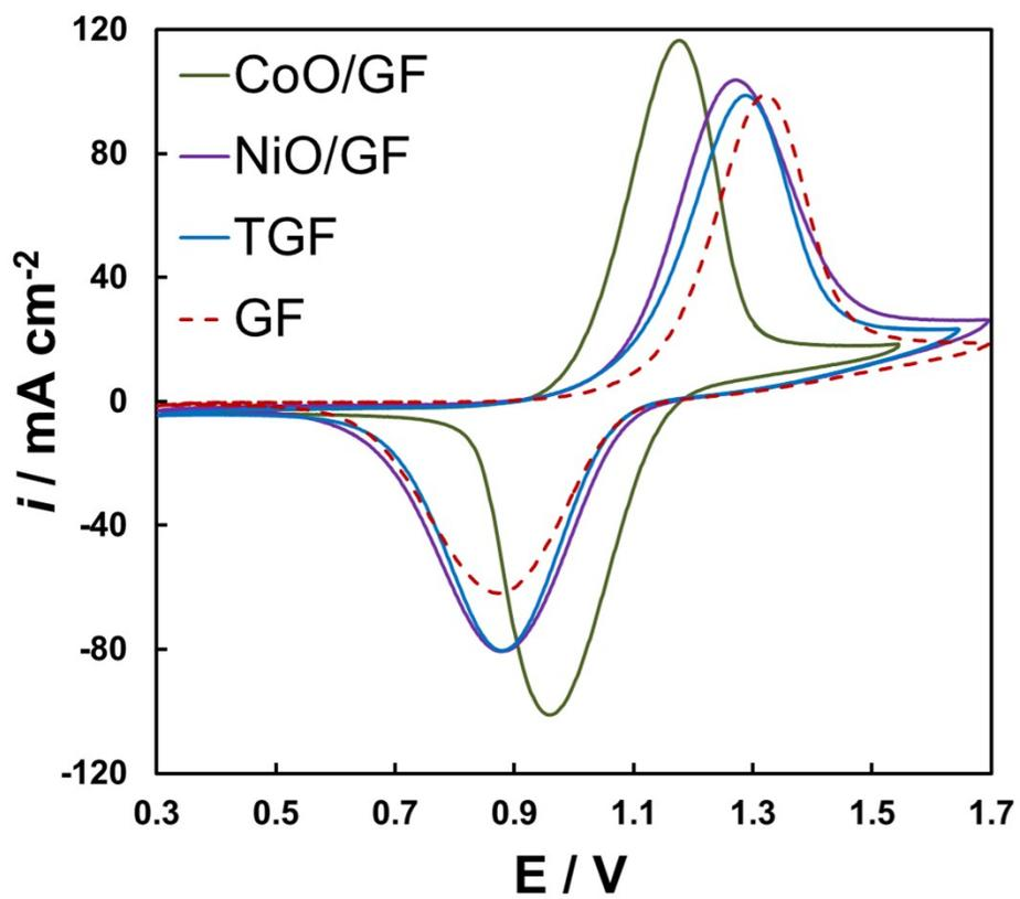
**Fig. S4:** Cyclic voltammograms of GF, TGF, NiO/GF and CoO/GF electrodes at a scan rate of  $2.5 \text{ mV s}^{-1}$  in  $0.2 \text{ M VOSO}_4 + 2 \text{ M H}_2\text{SO}_4$ .
