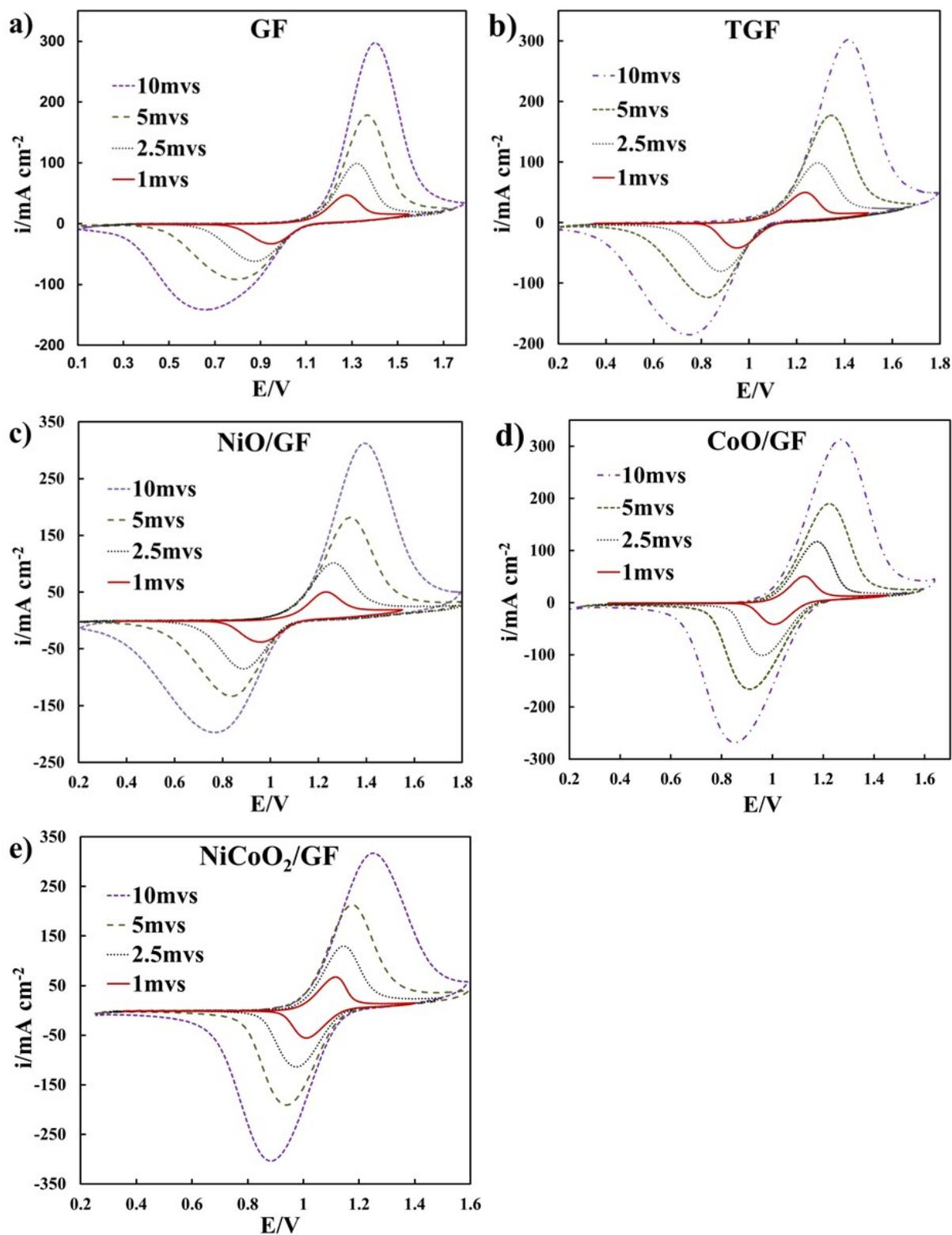
**Fig. S5:** Cyclic voltammograms of GF, TGF, NiO/GF, CoO/GF and NiCoO<sub>2</sub>/GF electrodes at a scan rate of 1, 2.5, 5 and 10  $\text{mv s}^{-1}$  in  $0.2\text{ M VOSO}_4 + 2\text{ M H}_2\text{SO}_4$ .
