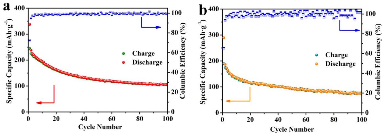
**Fig. S11.** Cycling performance of 3D-NFLG at a current density of (a)  $2 \text{ A g}^{-1}$  and (b)  $5 \text{ A g}^{-1}$  for 100 cycles.
