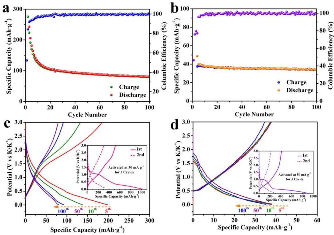
**Fig. S9. Electrochemical performance of potassium-ion batteries.** (a) Reversible specific capacity and coulombic efficiency and (b) potential versus specific capacity for  $\text{Fe}_2\text{O}_3@\text{NFLG-300}$  electrode during different cycles at  $1.0 \text{ A g}^{-1}$ , (c) Reversible specific capacity and coulombic efficiency and (d) potential versus specific capacity for  $\text{Fe}_2\text{O}_3@\text{NFLG-900}$  during different cycles at  $1.0 \text{ A g}^{-1}$ .
