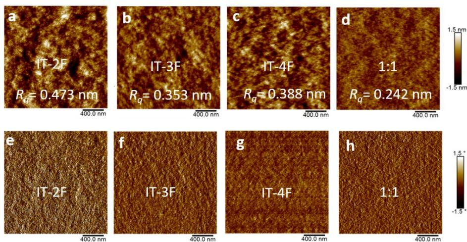
**Fig. S9.** a–d) AFM height images and e–f) AFM phase images of the neat and blended films.
