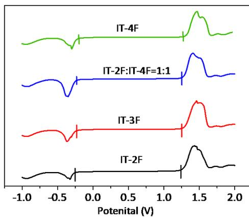
**Fig. S4.** Square wave voltammetry of acceptors and acceptor blends.
