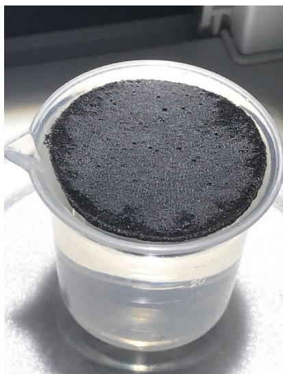
Fig. S5 photo image of the CPHS/aerogel functional PVA hydrogel, the hydrogel can self-float on deionized water. The volume of the deionized water was 33 ml.
