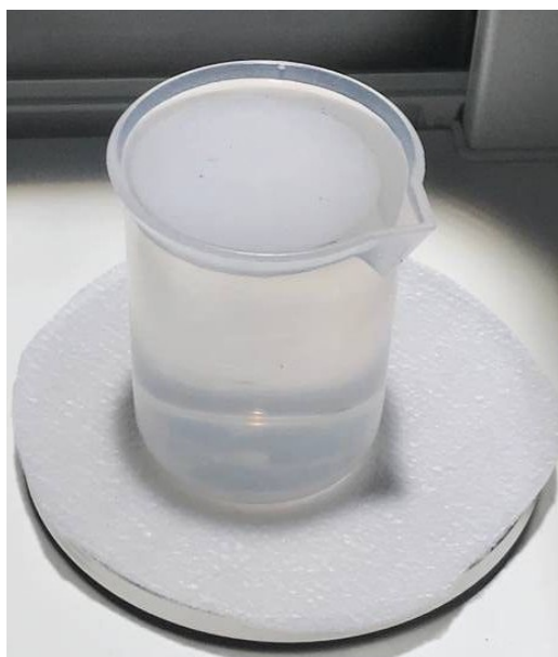
Fig. S17 Photo image of aerogel functionalized PVA hydrogels after stabilized in water. The hydrogel was white and it could self-float on water.
