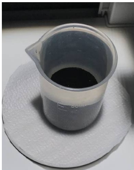
Fig. S15 Photo image of CPHS functionalized PVA hydrogels after stabilized in water. The hydrogel was black and it sink into the water bottom.
