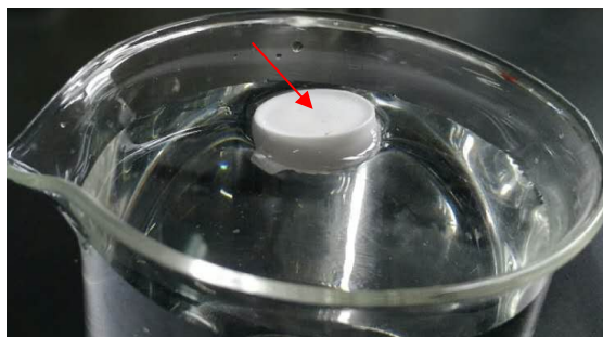
Fig. S4 PVA composite hydrogel with 15 wt.% of aerogel microparticles.
