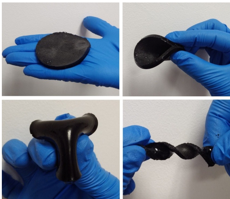
Fig. S7 Photo images of the hydrogel with or without deformation.
