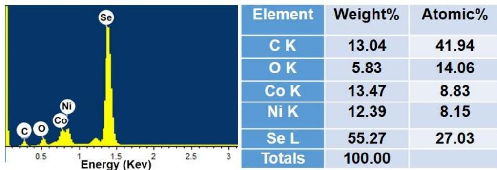
**Fig. S2** Energy dispersive spectrometer (EDS) analysis of  $\text{Ni}_{0.47}\text{Co}_{0.53}\text{Se}_2$  micro-nanosphere.
