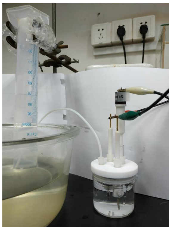
Figure S6 The gases collection device by water displacement.
