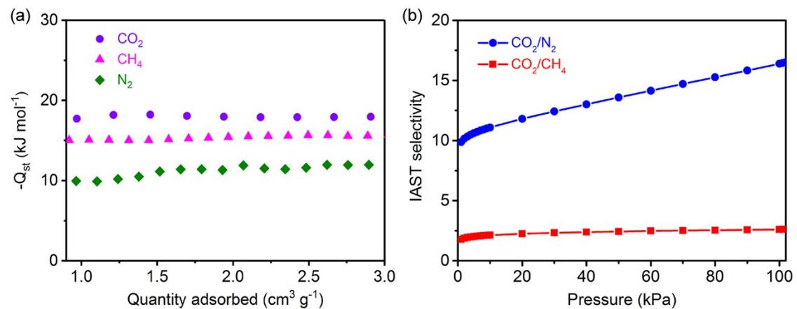
Fig. S4. (a) The isosteric heat of adsorption ( $Q_{st}$ ) for  $\text{CO}_2$ ,  $\text{CH}_4$  and  $\text{N}_2$  of COF-300. (b) The ideal adsorption solution theory (IAST) selectivity of COF-300 for the equal molar mixtures of  $\text{CO}_2/\text{CH}_4$  or  $\text{CO}_2/\text{N}_2$  at 298K and 1 bar.
