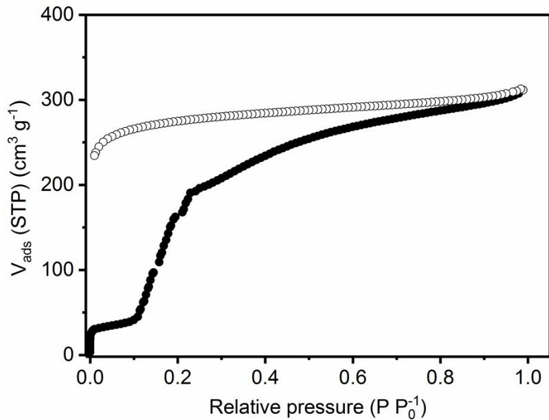
Fig. S17.  $N_2$  sorption isotherm (77 K) of COF@PEI (adsorption: solid symbols; desorption: empty symbols).
