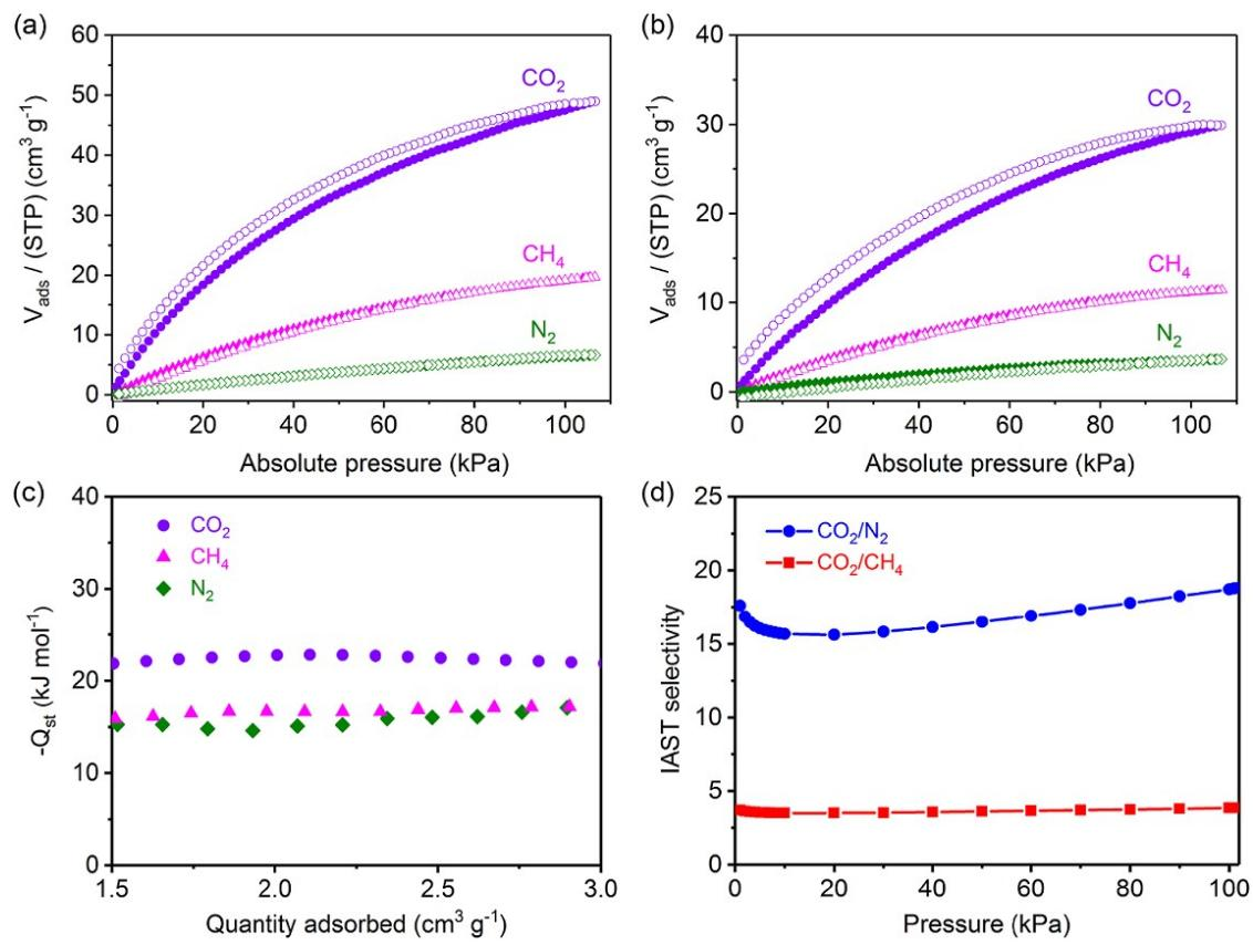
Fig. S18.  $\text{CO}_2$ ,  $\text{CH}_4$  and  $\text{N}_2$  sorption isotherms of COF@PEI measured at (a) 273 K and (b) 298 K. (c) The isosteric heat of adsorption ( $Q_{\text{st}}$ ) for  $\text{CO}_2$ ,  $\text{CH}_4$  and  $\text{N}_2$  of COF@PEI. (d) The ideal adsorption solution theory (IAST) selectivity of COF@PEI for  $\text{CO}_2/\text{CH}_4$  or  $\text{CO}_2/\text{N}_2$  equal molar mixtures at 298 K and 1 bar.
