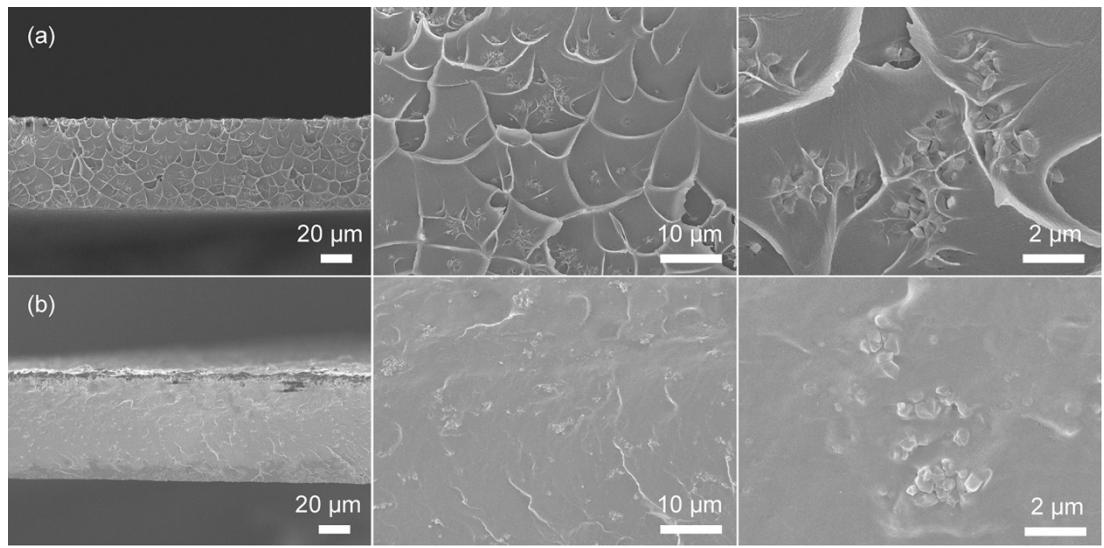
Fig. S19. Cross-sectional FESEM images of (a) COF@PEI/6FDA-DAM-7 and (b) COF@PEI/Pebax-10 MMMs at different magnifications.
