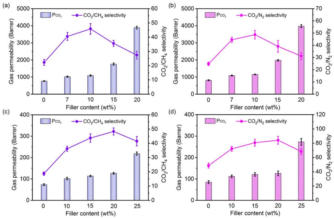
Fig. S20. The effect of COF@PEI filler content on membrane separation performance tested at 25 °C with a transmembrane pressure of 1 bar. (a) CO<sub>2</sub>/CH<sub>4</sub> and (b) CO<sub>2</sub>/N<sub>2</sub> separation performance of COF@PEI/6FDA-DAM series MMMs. (c) CO<sub>2</sub>/CH<sub>4</sub> and (d) CO<sub>2</sub>/N<sub>2</sub> separation performance of COF@PEI/Pebax series MMMs.
