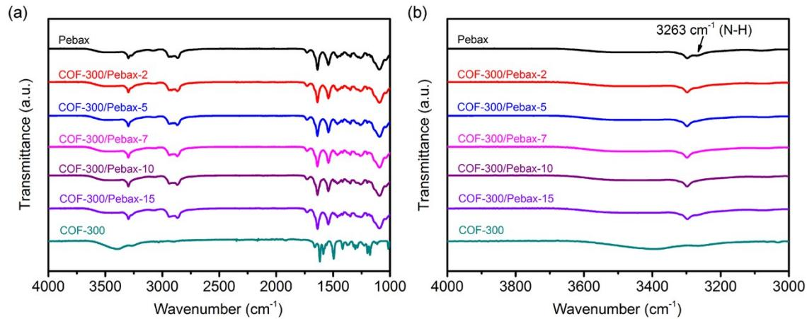
Fig. S8. FTIR spectra of COF-300/Pebax series MMMs.
