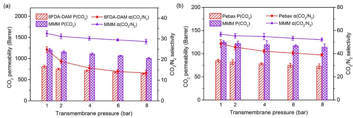
Fig. S13. Transmembrane pressure influence on the  $\text{CO}_2/\text{N}_2$  separation performance of (a) 6FDA-DAM and (b) Pebax systems.
