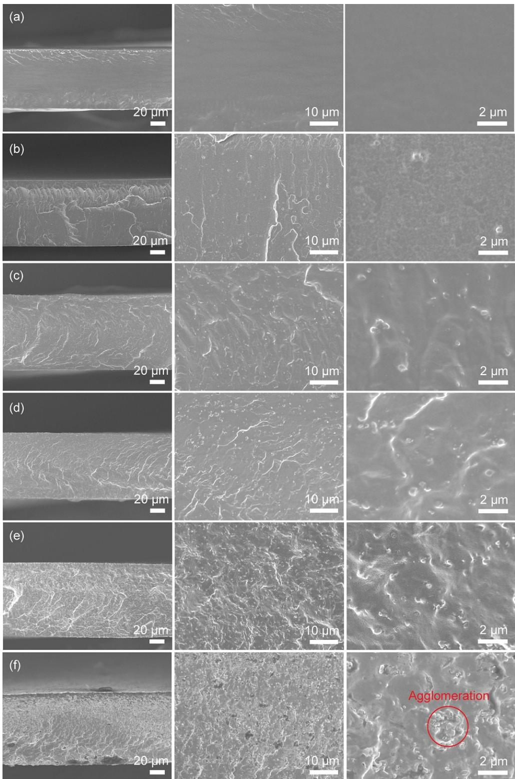
Fig. S6. Cross-sectional FESEM images of COF-300/Pebax MMMs containing (a) 0 wt%, (b) 2 wt%, (c) 5 wt%, (d) 7 wt%, (e) 10 wt% and (f) 15 wt% COF-300 fillers at different magnifications.
