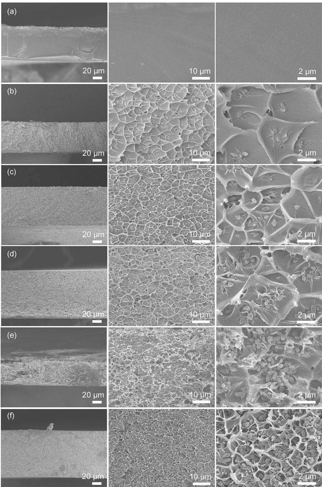
Fig. S5. Cross-sectional FESEM images of COF-300/6FDA-DAM MMMs containing (a) 0 wt%, (b) 2 wt%, (c) 5 wt%, (d) 7 wt%, (e) 10 wt% and (f) 15 wt% COF-300 fillers at different magnifications.
