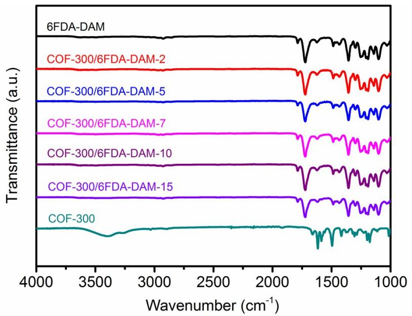
Fig. S7. FTIR spectra of COF-300/6FDA-DAM series MMMs.
