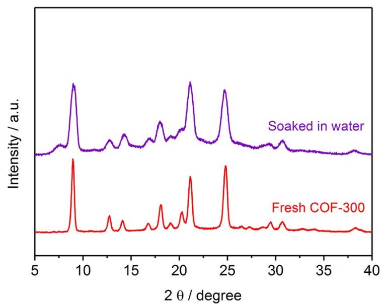
Fig. S2. PXRD patterns of fresh COF-300 and COF-300 soaked in water at room temperature for 3 days.
