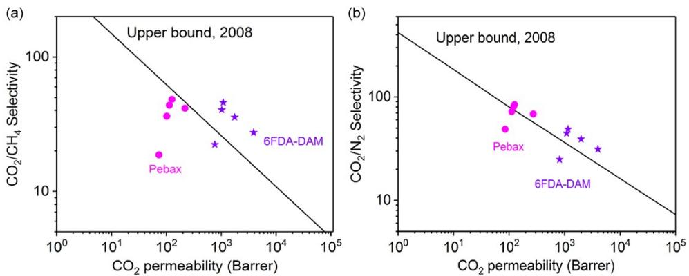
Fig. S21. Robeson upper bound plots for (a) CO<sub>2</sub>/CH<sub>4</sub> and (b) CO<sub>2</sub>/N<sub>2</sub> of COF@PEI/6FDA-DAM and COF@PEI/Pebax MMMs.
