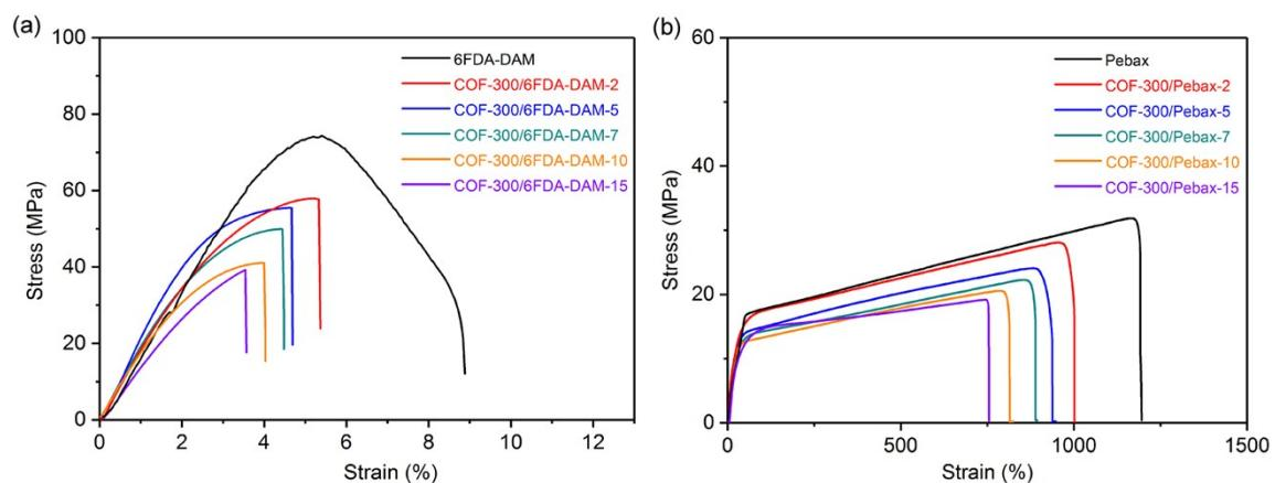
Fig. S12. Stress-strain curves for (a) COF-300/6FDA-DAM series MMMs; (b) COF-300/Pebax series MMMs.
