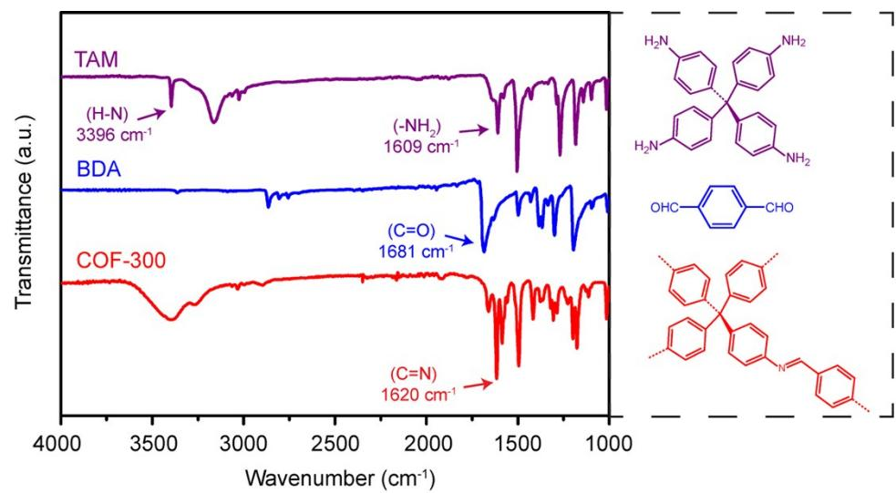
Fig. S1. FTIR spectra of COF-300 and its monomers.
