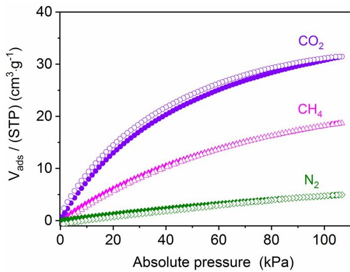
Fig. S3. CO<sub>2</sub>, CH<sub>4</sub>, and N<sub>2</sub> sorption isotherms of COF-300 measured at 273 K.
